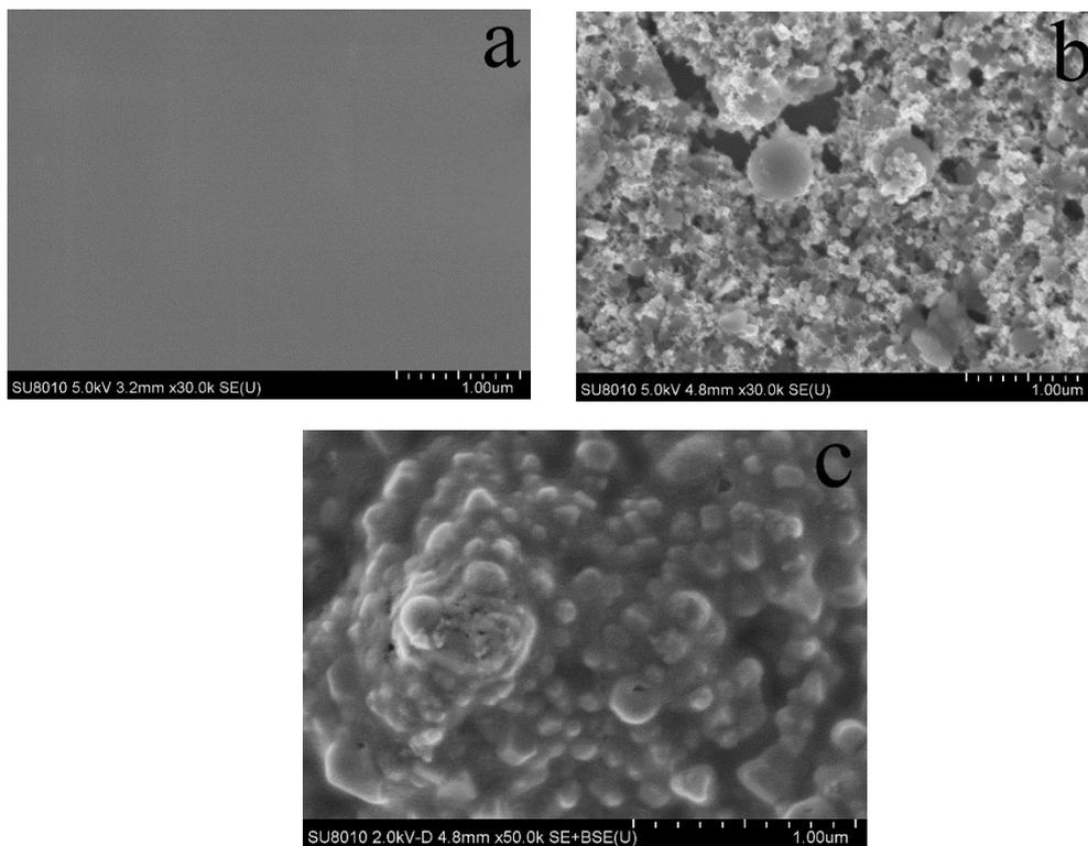
**Figure S 6.** SEM images of a bare GCE (a), a Yb-MOF@Au-NPs/GCE (b) and an anti-CEA/Yb-MOF@Au-NPs/GCE (c).
