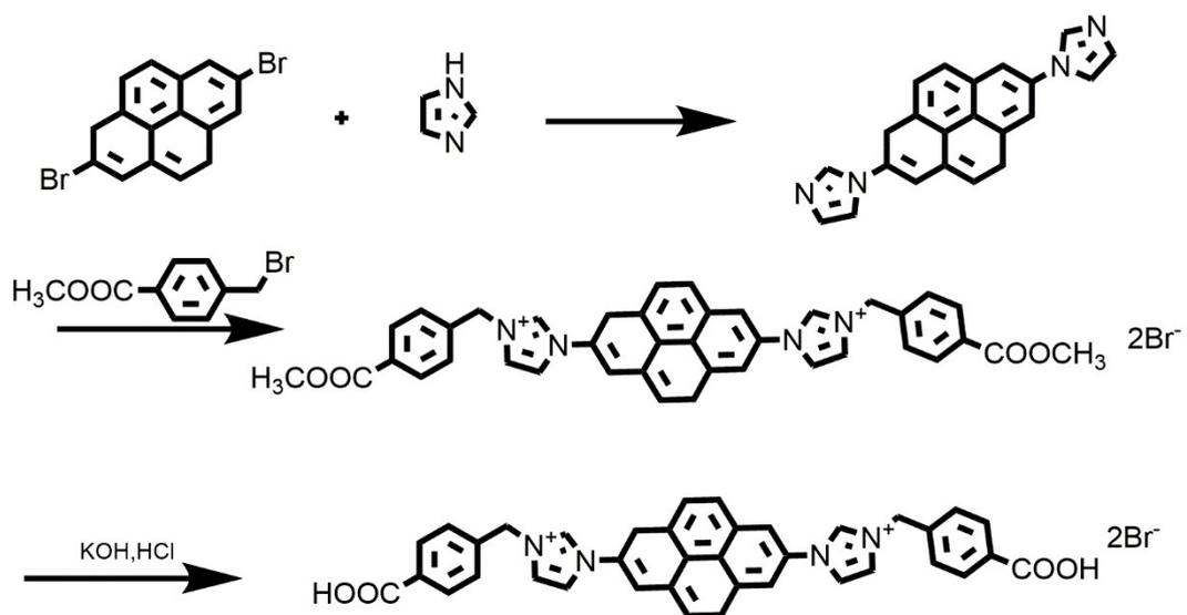
**Scheme S1.** Scheme for the synthesis of DDPDBCBIIm(Br)<sub>2</sub> ionic liquid.
