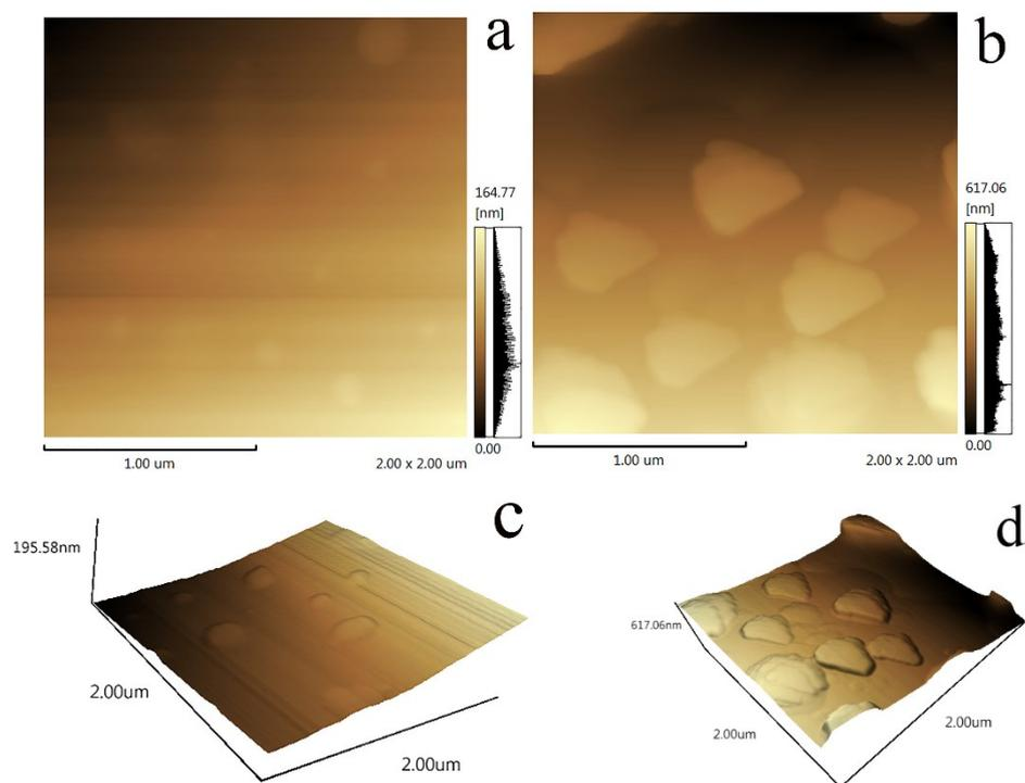
**Figure S 7.** AFM images of an Yb-MOF@Au-NPs/GCE (a) and an anti-CEA/ Yb-MOF@Au-NPs/GCE (b); 3D images of Yb-MOF@Au-NPs/GCE(c) and anti-CEA/ Yb-MOF@Au-NPs/GCE (d).
