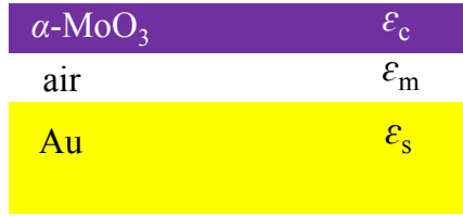
Fig. S3 Side view of the layered structure of monolayer \alpha -MoO 3 /nano airgap/Au.
