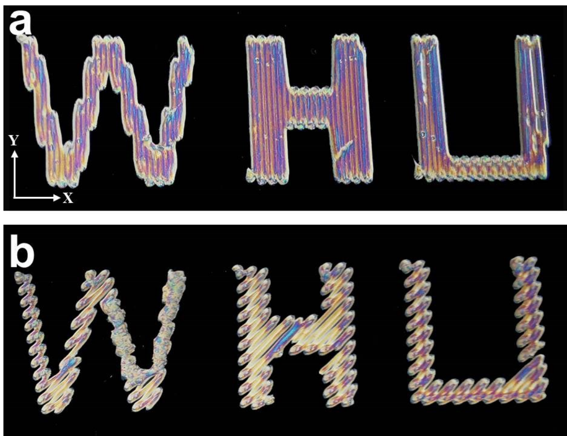
Figure S9. Photographs of “WHU” patterns printed with the recycled inks using a nozzle with a diameter of 0.6 mm under polarized light. Printing conditions: (a) grid fill width was 0.6 mm and writing angle was 90°. (b) grid fill width was 0.3 mm and writing angle was 45°. The length of all patterns in Y direction was 2 cm.
