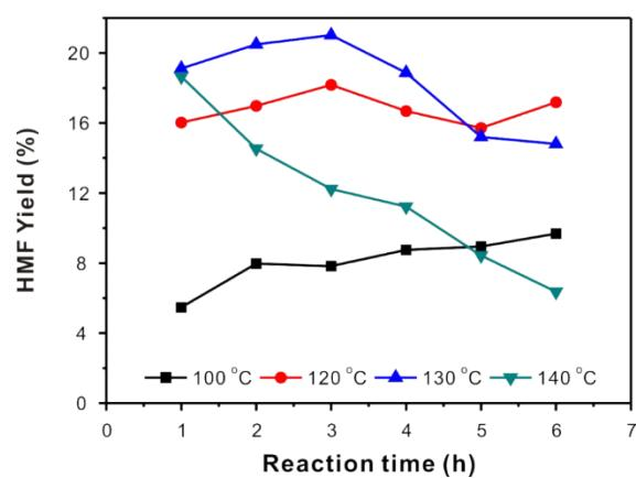
**Fig. S4** Changes in HMF yields from glucose over BS-GO depending on the temperature and reaction time shown in Table S6.
