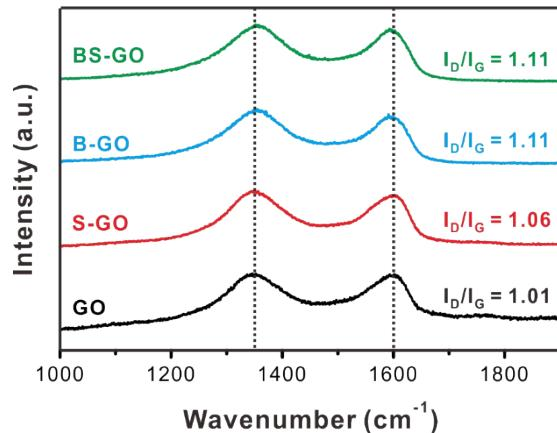
**Fig. S2** Raman spectra of GO and GO-derivatives. An argon ion laser, with a wavelength of 532 nm, was used as an excitation source. The D and G bands appear at 1346  $\text{cm}^{-1}$  and 1600  $\text{cm}^{-1}$ , respectively.
