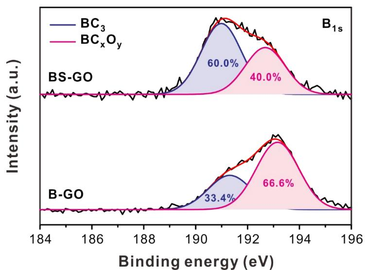
**Fig. S1** Deconvoluted high-resolution XPS B1s spectra of B-GO and BS-GO.
