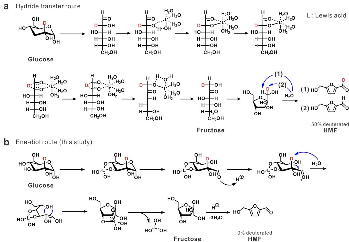
**Fig. S5** Reaction pathways from *D*-Glucose-2-*d*<sub>1</sub> to HMF with (a) the hydride transfer route and (b) the ene-diol route.
