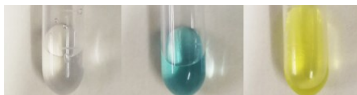
Figure S5. Photographs of TMB+H 2 O 2 , TMB+H 2 O 2 +Pt@HSA/CA NPs, and TMB+H 2 O 2 +Pt@HSA/CA NPs+H 2 SO 4 .
