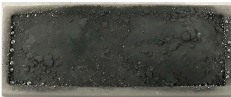
Supplementary Figure 5 Optical image of the product with 25.3% of %B, showing original powder morphologies after the growth.
