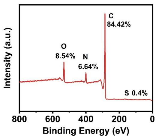
**Fig. S2** XPS survey spectrum of ACNS.
