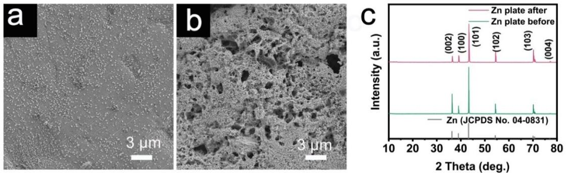
**Fig. S6** SEM images of Zn anode (a) before and (b) after cycling. (c) XRD patterns of Zn anode before and after cycling.
