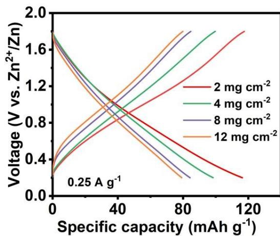
**Fig. S3** GCD curves of the ACNS under various mass loadings.
