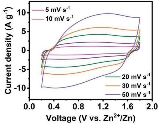
**Fig. S4** CV curves of the quasi-solid-state Zn// $\kappa$ -CG/PAAm/Zn(CF<sub>3</sub>SO<sub>3</sub>)<sub>2</sub>//ACNS ZHSC at different scan rates.
