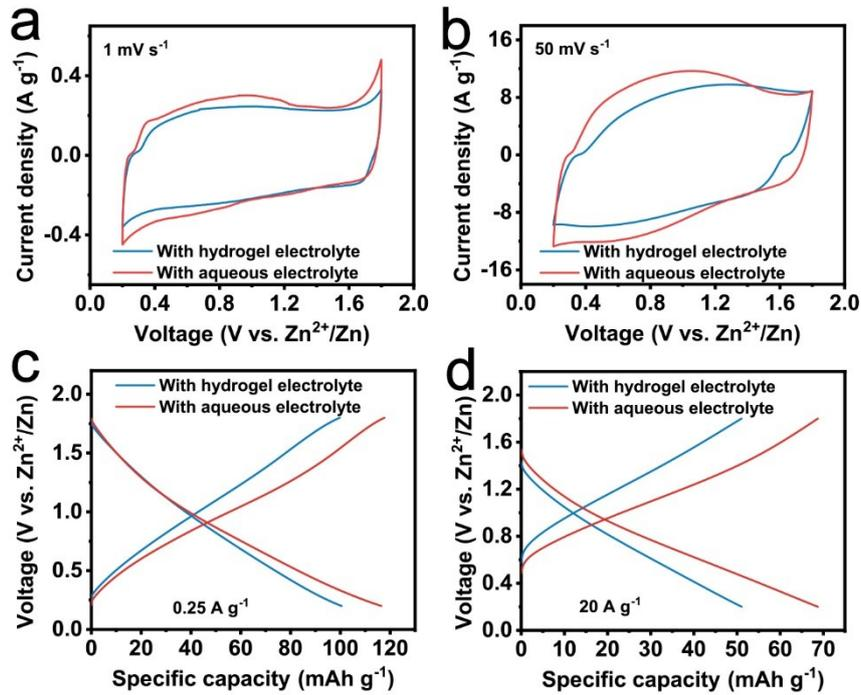
**Fig. S5** CV curves of ZHSCs with different electrolytes at (a) 1 mV s<sup>-1</sup> and (b) 50 mV s<sup>-1</sup>. GCD curves of ZHSCs with different electrolytes at (c) 0.25 A g<sup>-1</sup> and (d) 20 A g<sup>-1</sup>.
