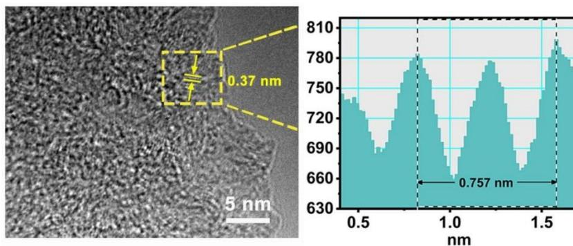
**Fig. S1** HRTEM image of ACNS with the corresponding intensity profile for the line scan across the lattice fringes.
