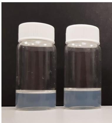
Figure S2. Vials containing liposomal dispersions of DPPC/Cholesterol stabilized by 20.0 mol % of DDP-PG72 (left) and DDP-PG110 (right).
