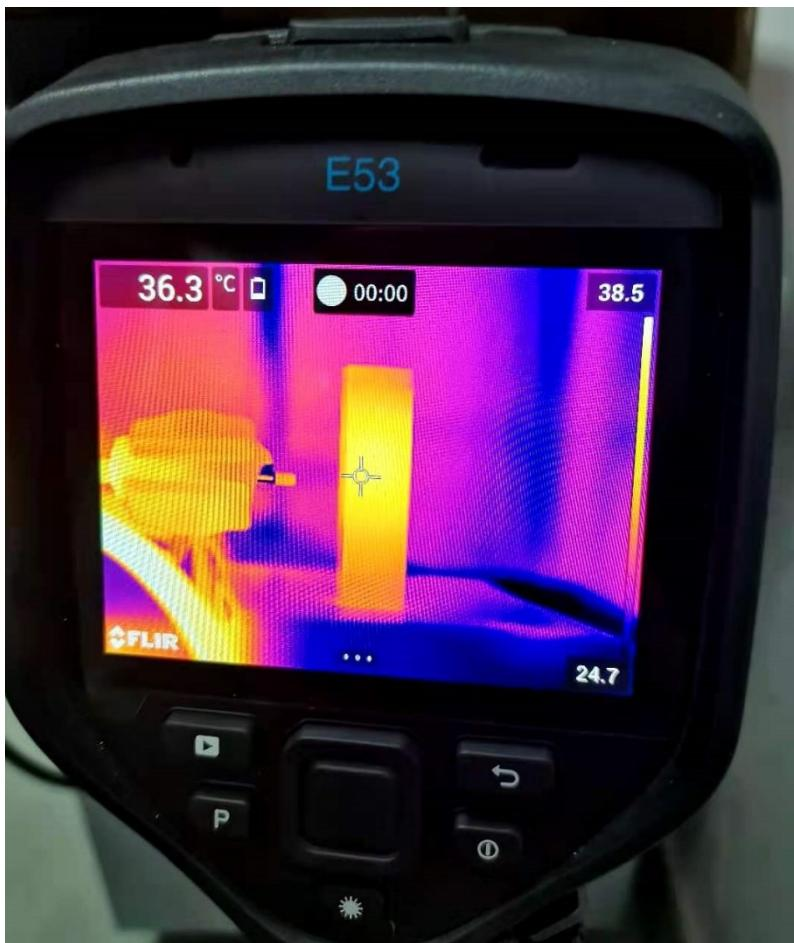
**Fig. S17** Photothermal conversion characterizations of Gd-Fe/HCSs aqueous solution
