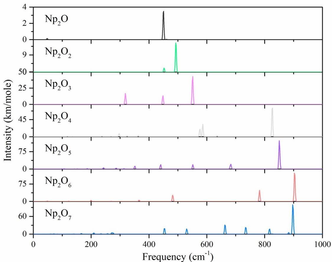
**Figure S8.** DFT computed spectrum of the lowest-energy isomer for  $[\text{Np}_2\text{O}_x]$  species. None scaled.
