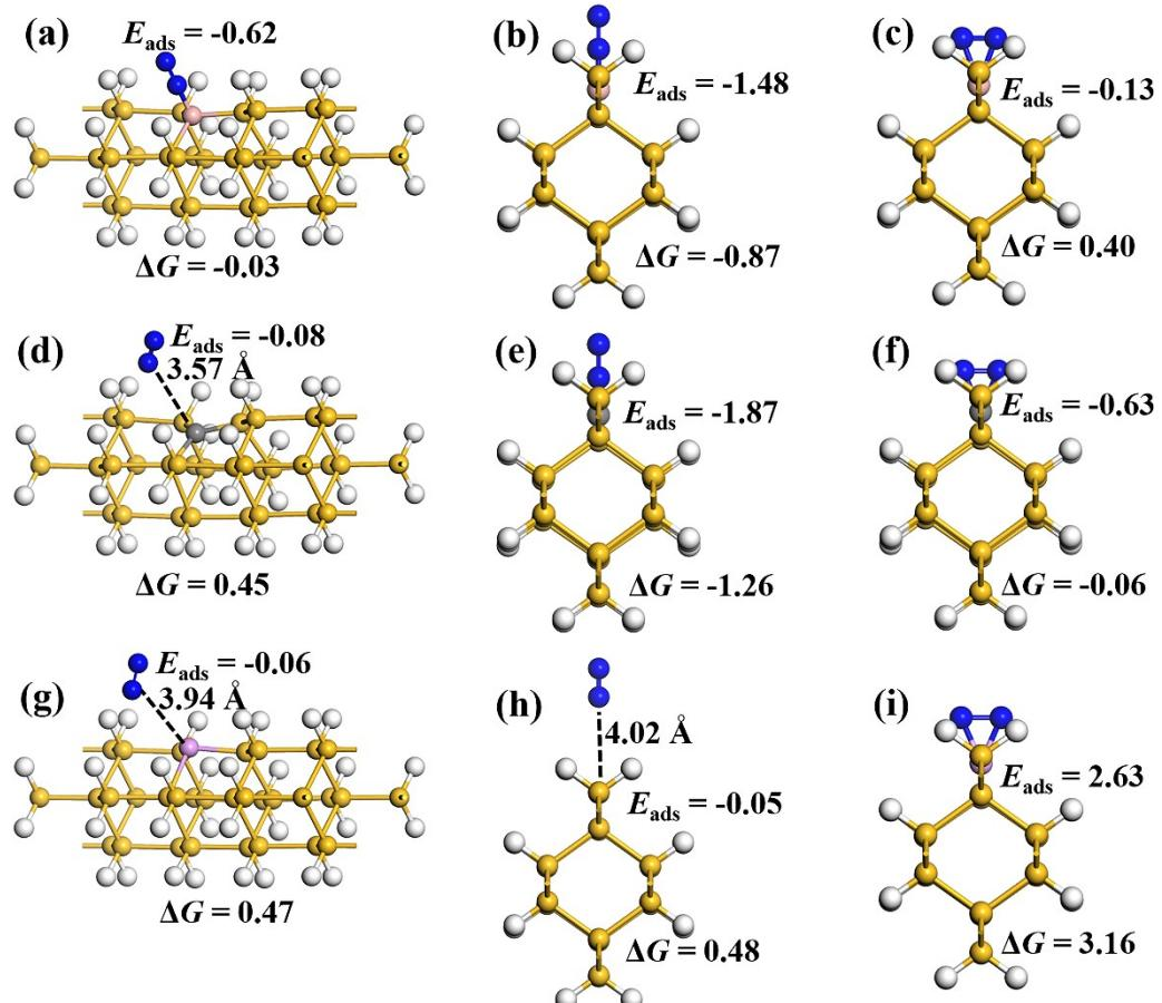
**Fig. S7** N<sub>2</sub> adsorption configurations on B<sub>3</sub>C, B<sub>2</sub>C, C<sub>3</sub>C, C<sub>2</sub>C, P<sub>3</sub>C, and P<sub>2</sub>C catalysts. Black values near the dash line indicate the distance between N<sub>2</sub> and active sites. Color scheme: Si (yellow), H (White), N (blue).
