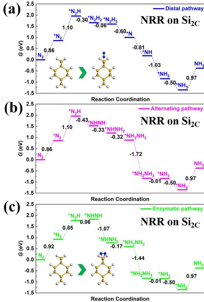
**Fig. S6** Diagram of the free energy evolution along the reaction coordination, including the distal (a), alternating (b), and enzymatic (c) pathways. Insets in the images display the N<sub>2</sub> capture step. Color scheme: Si (yellow), H (White), N (blue).
