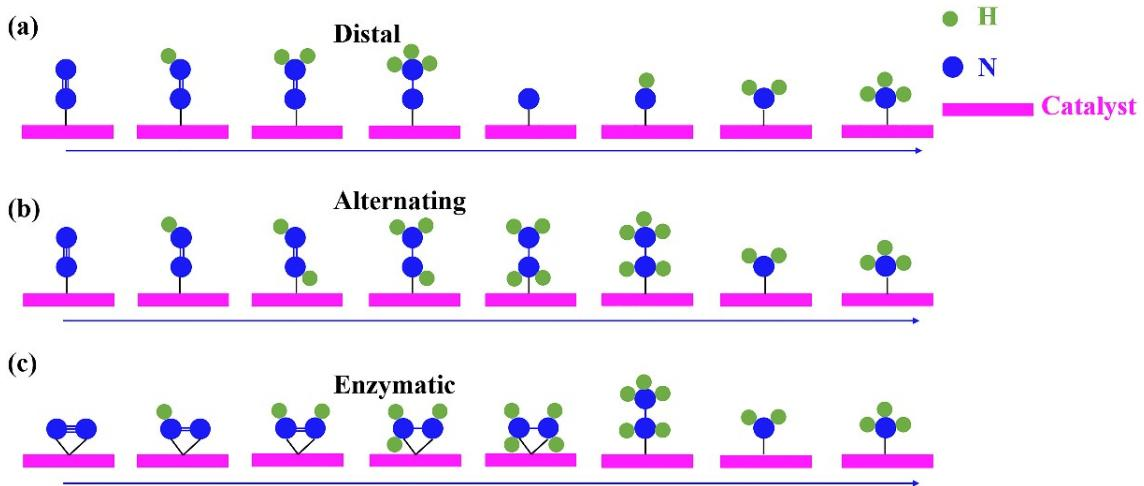
**Fig. S3** Schematic diagram of NRR pathways, including (a) distal, (b) alternating and (c) enzymatic ones.
