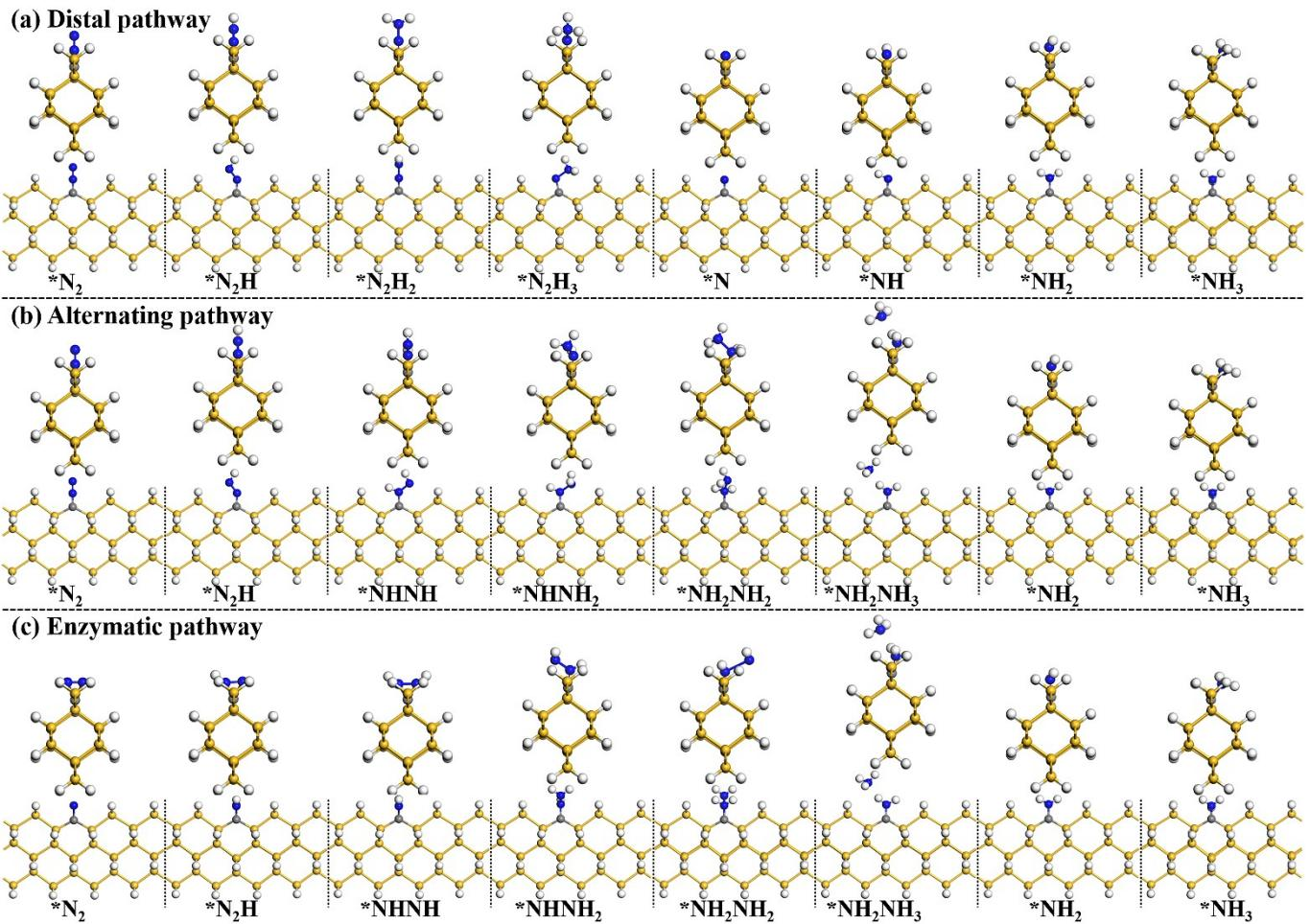
**Fig. S8** NRR on C<sub>2</sub>C, including the distal, alternating and enzymatic pathways. Color scheme: Si (yellow), H (White), N (blue), C (grey).
