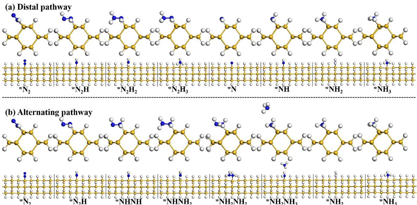
**Fig. S4** NRR pathways on  $\text{Si}_3\text{C}$ , including (a) distal and (b) alternating reaction pathways. Color scheme: Si (yellow), H (White), N (blue).
