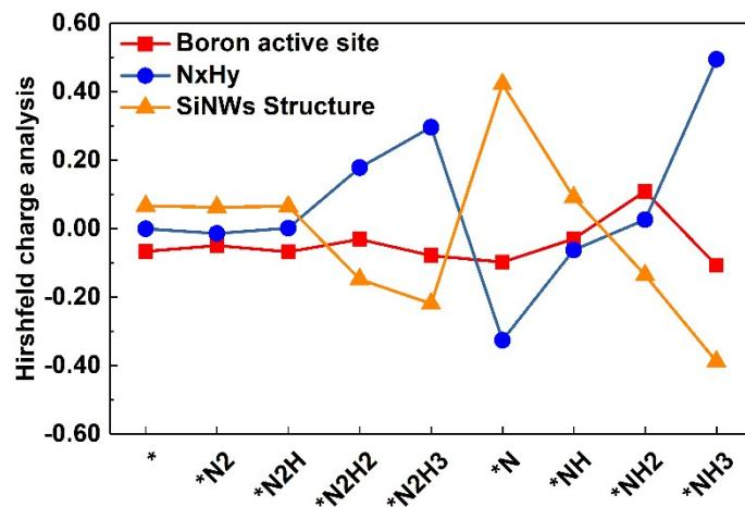
**Fig. S11** Hirshfeld analysis for the optimal distal reaction pathway on  $\text{B}_{2\text{C}}$ .
