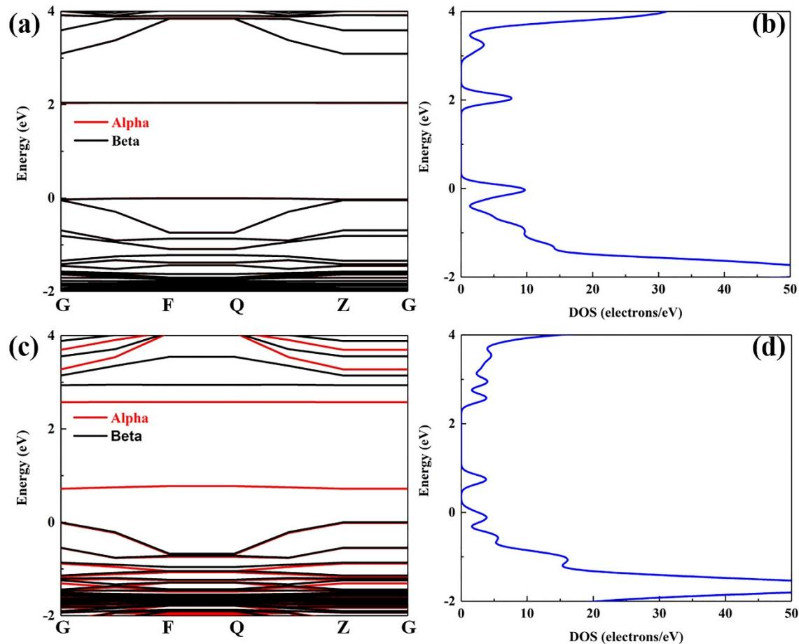
**Fig. S12** Band structure and density of states (DOS) for Si<sub>2</sub>C (a, b) and B<sub>2</sub>C (c, d).
