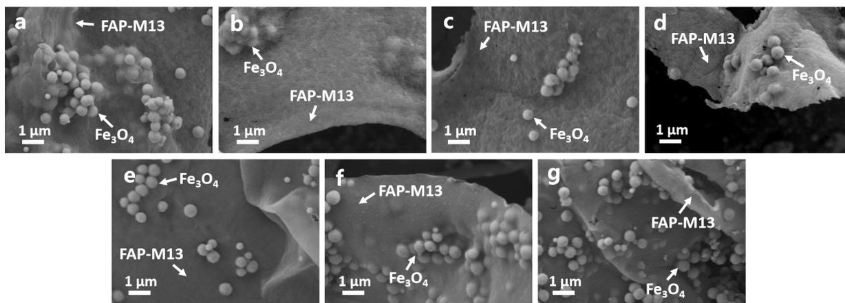
**Fig. S8** The SEM images of the structures of (FAP-M13)-Fe<sub>3</sub>O<sub>4</sub> magnetic virus hydrogels under different crosslinking pH including (a) pH = 4, (b) pH = 6, (c) pH = 7, (d) pH = 7.5, (e) pH = 8, (f) pH = 9, (g) pH = 11. The rest of preparation conditions were 0.5% glutaraldehyde at 37 °C, 200rpm, 4h. Arrows point to crosslinked FAP-M13 hydrogel network and bare Fe<sub>3</sub>O<sub>4</sub>.
