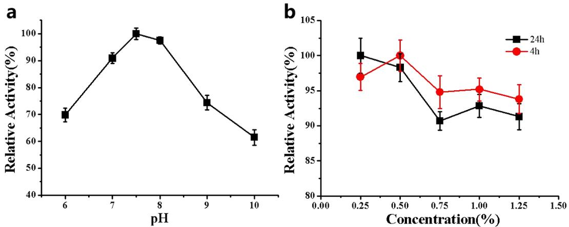
**Fig. S4** Optimization of magnetic composite hydrogel preparation conditions. (a) Optimization of crosslinking pH under 0.5% glutaraldehyde at 37 °C, 200rpm, 4h. (b) Optimization of glutaraldehyde final concentration for crosslinking under 4h or 24h at pH=7.5, 37 °C, 200rpm.
