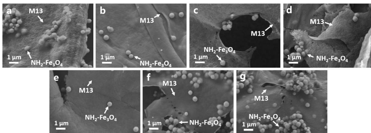
**Fig. S7** The SEM images of the structures of M13-(NH<sub>2</sub>-Fe<sub>3</sub>O<sub>4</sub>) magnetic virus hydrogels under different crosslinking pH including (a) pH = 4, (b) pH = 6, (c) pH = 7, (d) pH = 7.5, (e) pH = 8, (f) pH = 9, (g) pH = 11. The rest of preparation conditions were 0.5% glutaraldehyde at 37 °C, 200rpm, 4h. Arrows point to crosslinked M13 hydrogel network and NH<sub>2</sub>-Fe<sub>3</sub>O<sub>4</sub>.
