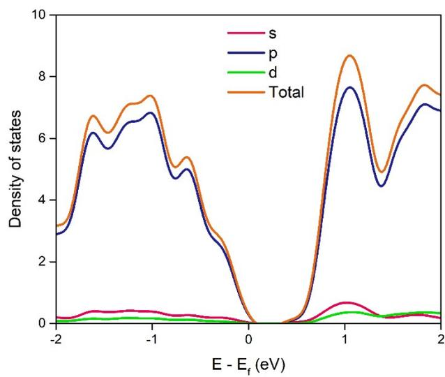
**Figure S2.** Sum and partial density of states of tellurene.
