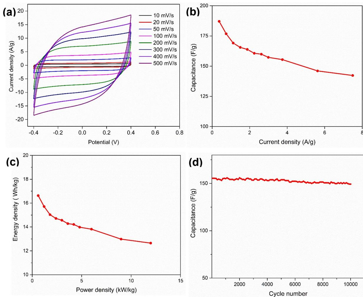
**Figure S5:** Gravimetric electrochemical performance Ni-Mn oxides/CNT@CNF super capacitor device (a) cyclic voltammograms at various scan rates of from 10 to 500 mV s<sup>-1</sup> b) specific gravimetric capacitance at different current densities c) energy and power densities and d) cycling test at a current density of 3.74 A g<sup>-1</sup>.
