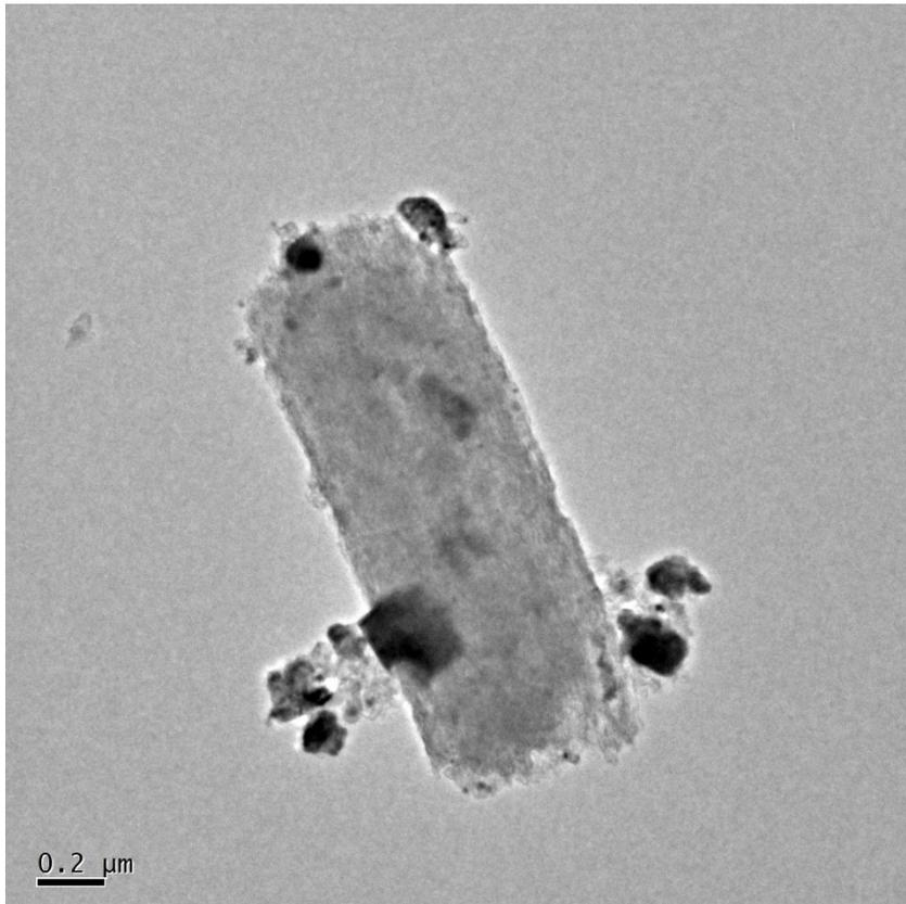
**Figure S4:** TEM image of a part of the nanofiber showing the growth of Ni-Mn oxides antennas out of the fibres surface.
