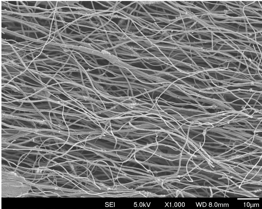
**Figure S2:** SEM images of the as prepared free-standing Ni-Mn oxides /CNT@CNF electrode.
