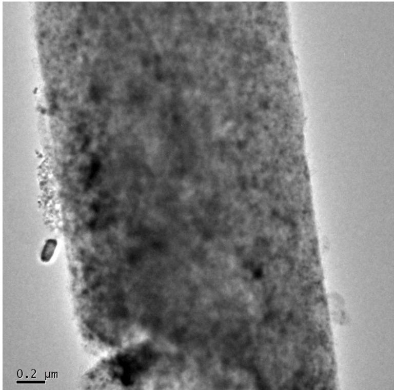
**Figure S3:** TEM image of the nanofibers showing the tubular structure is composed of interconnected nanoparticles.
