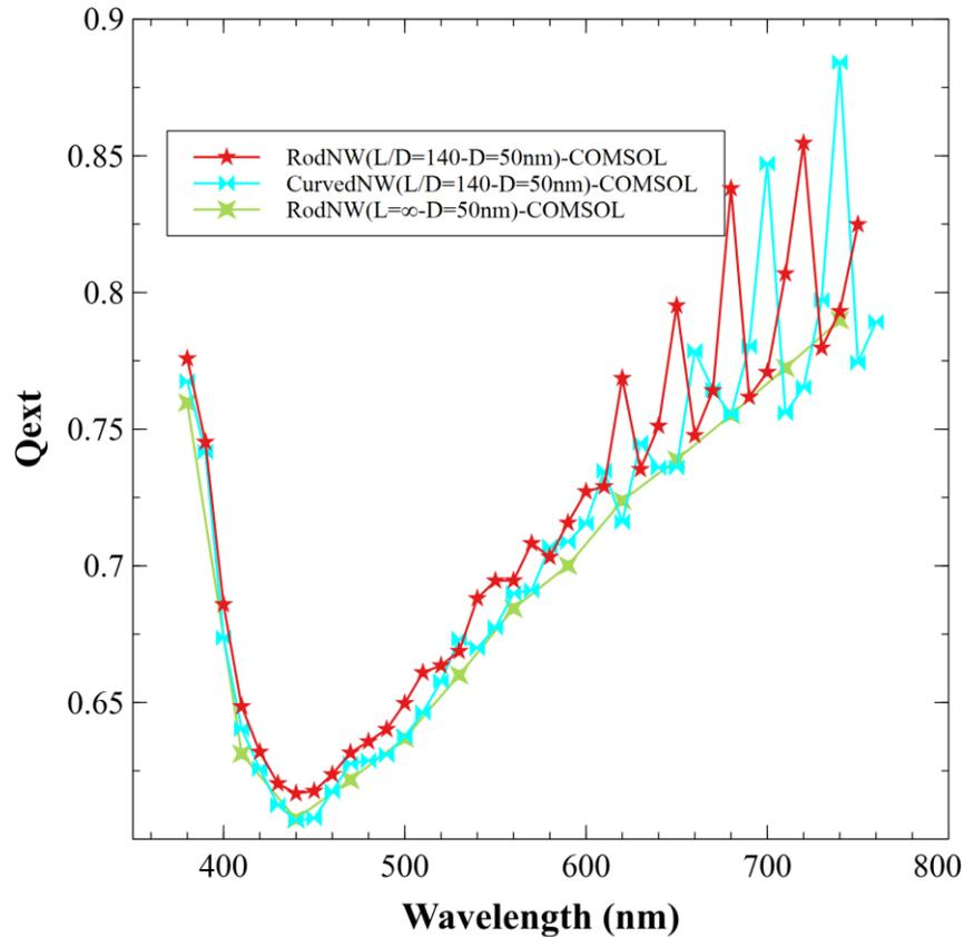
**Figure S4.** Extinction efficiencies as a function of wavelength from  $350 \text{ nm}$  to  $750 \text{ nm}$  of an Ag single nanowire calculated using COMSOL. The red, cyan, and green color curves refer to straight/finite, curved/finite and infinite nanowire (2- dimensional circular disk), respectively. In all simulations, the nanowires have the same diameter of  $D = 50 \text{ nm}$  and the finite nanowires (straight and curved) have the same (arc) length of  $L = 7 \mu\text{m}$ .
