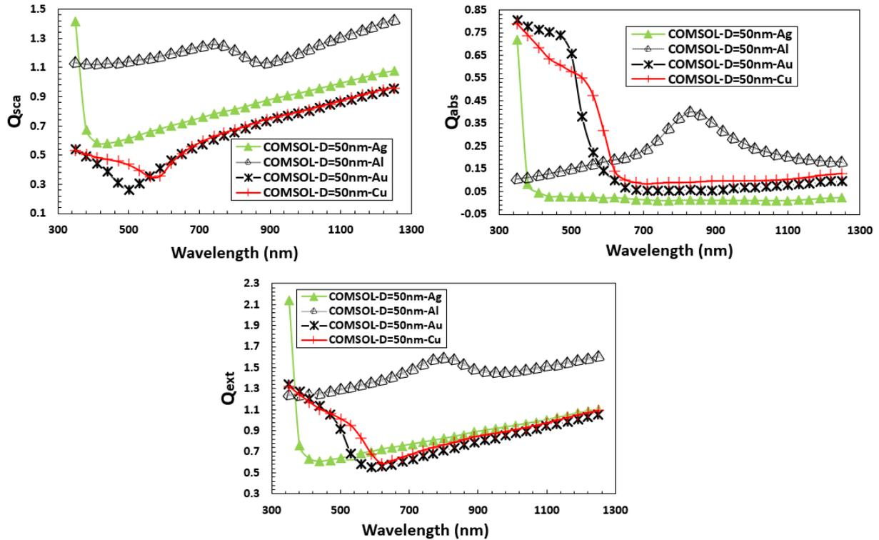
**Figure S3.** (top-left) Scattering, (top-right) absorption, and (bottom) extinction efficiency coefficients obtained using COMSOL for different materials (Ag, Al, Au, Cu) and of cylindrical shape with a diameter of 50 nm. The wavelength was varied from  $\sim 300 - 1300$  nm. These results were taken with the 2D circular disk model.
