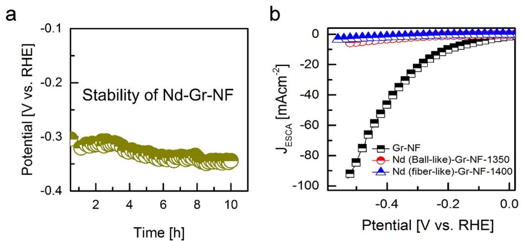
**Fig. S7** Stability for 10 hours (a) and ESCA normalized LSV's of Gr-NF, Nd-Gr-NF-1350 and Nd-Gr-NF-1400
