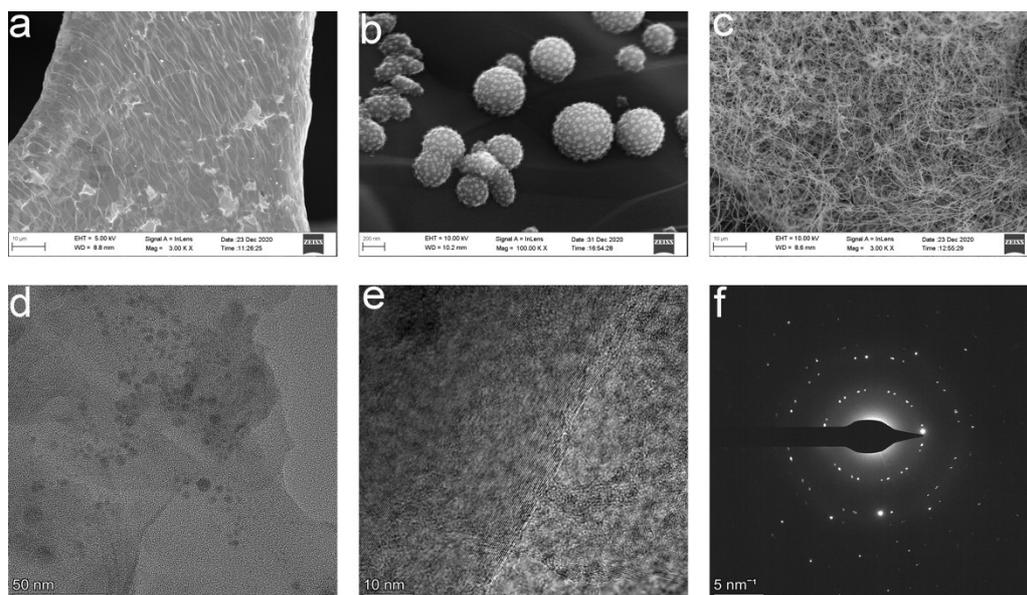
**Fig. S8** SEM of graphene (a), Nd-balls on graphene (b), and Nd-fiber on graphene grown on nickel foam (c). HRTEM of ball-like Nd in graphene sheets (d), high-resolution HRTEM (e), and SAED pattern (f).
