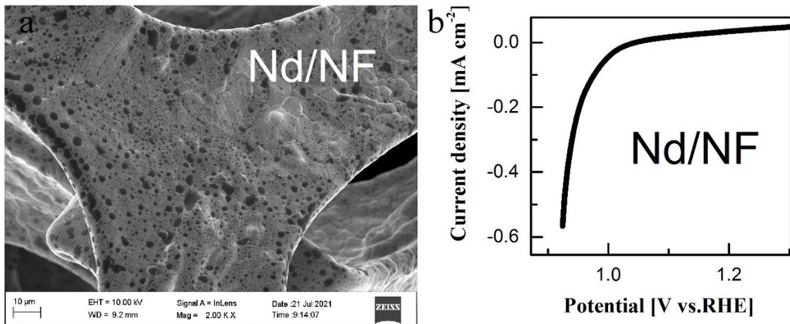
**Fig. S6** Nd deposited on nickel foam (NF) (a) and corresponding LSV in. KOH medium (b)
