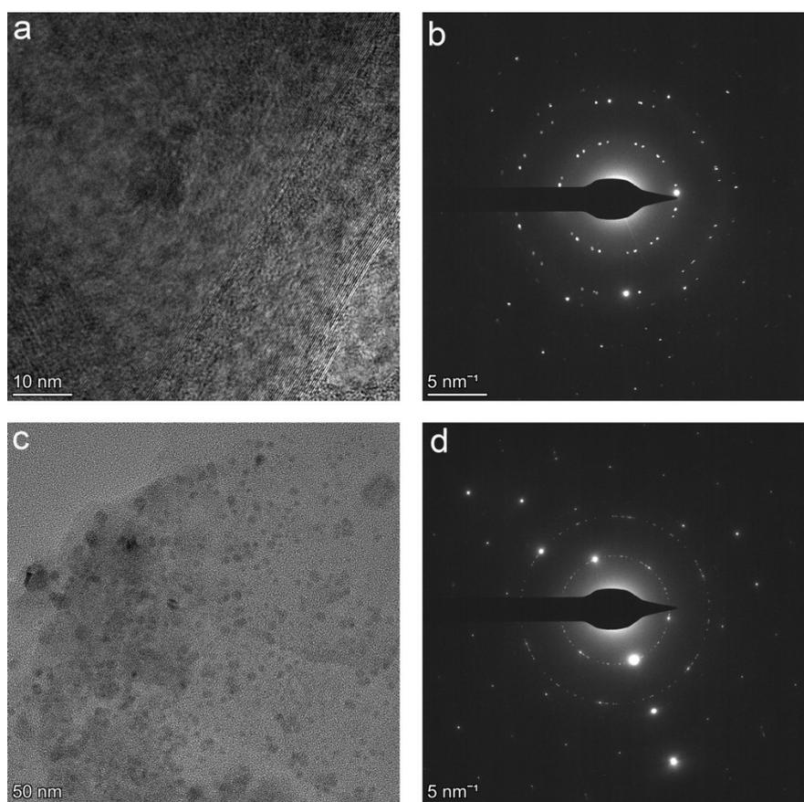
**Fig. S5** HRTEM of transferred as-grown graphene on nickel foam (a) and its corresponding SAED pattern (b). The transferred Nd-graphene with small Nd-particles (c) and corresponding SAED pattern (d).
