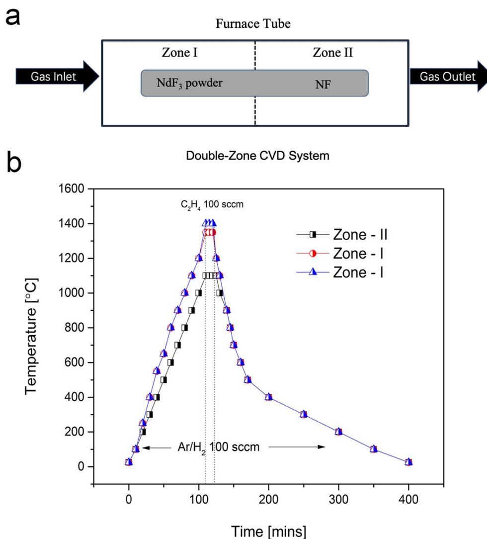
**Fig. S1** (a) Schematic of double zone CVD system and (b) growth conditions (temperature vs. time (flow of gases))
