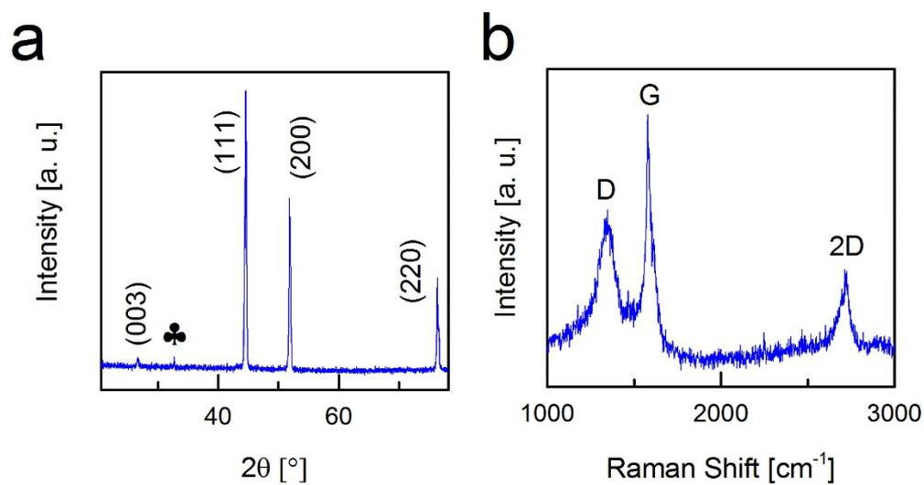
**Fig. S9** XRD of Nd-Gr-NF (a) and Raman spectroscopy (b)
