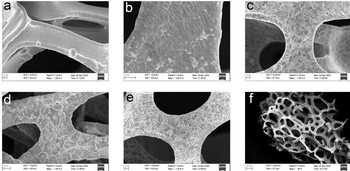
**Fig. S4** Surface of nickel foam (a), graphene grown on nickel substrate (b), Nd-Gr/NF-1200°C, (c) Nd-Gr/NF-1250°C, (d) Nd-Gr/NF-1300°C (e) Nd-Gr/NF-1350°C (f) Nd-Gr/NF-1400°C
