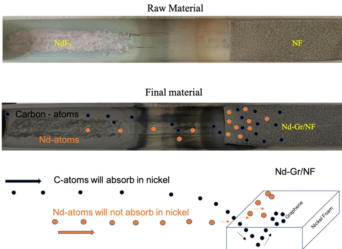
**Fig. S2** A comparison of the situation when loading the prepared samples and after the experiment, and the schematic of growth mechanism.
