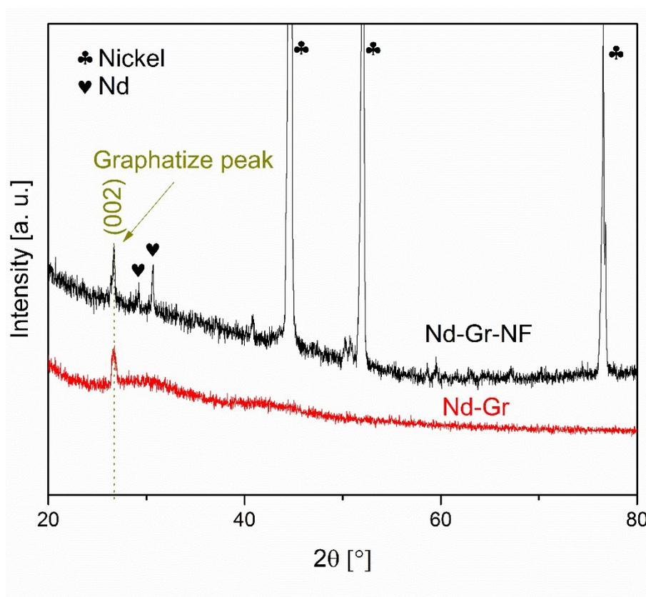
**Fig. S3** The XRD of Nd-Gr-NF and nickel etched Nd-Gr samples <sup>10</sup>
