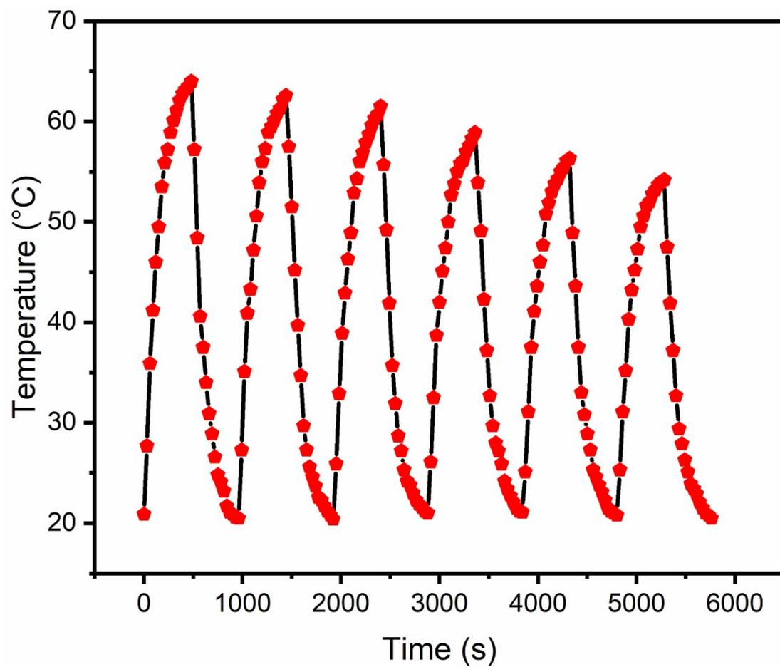
**Figure S8.** Heat-cold cycle experiment of the NIR-II nanoprobe under 633 nm laser irradiation.
