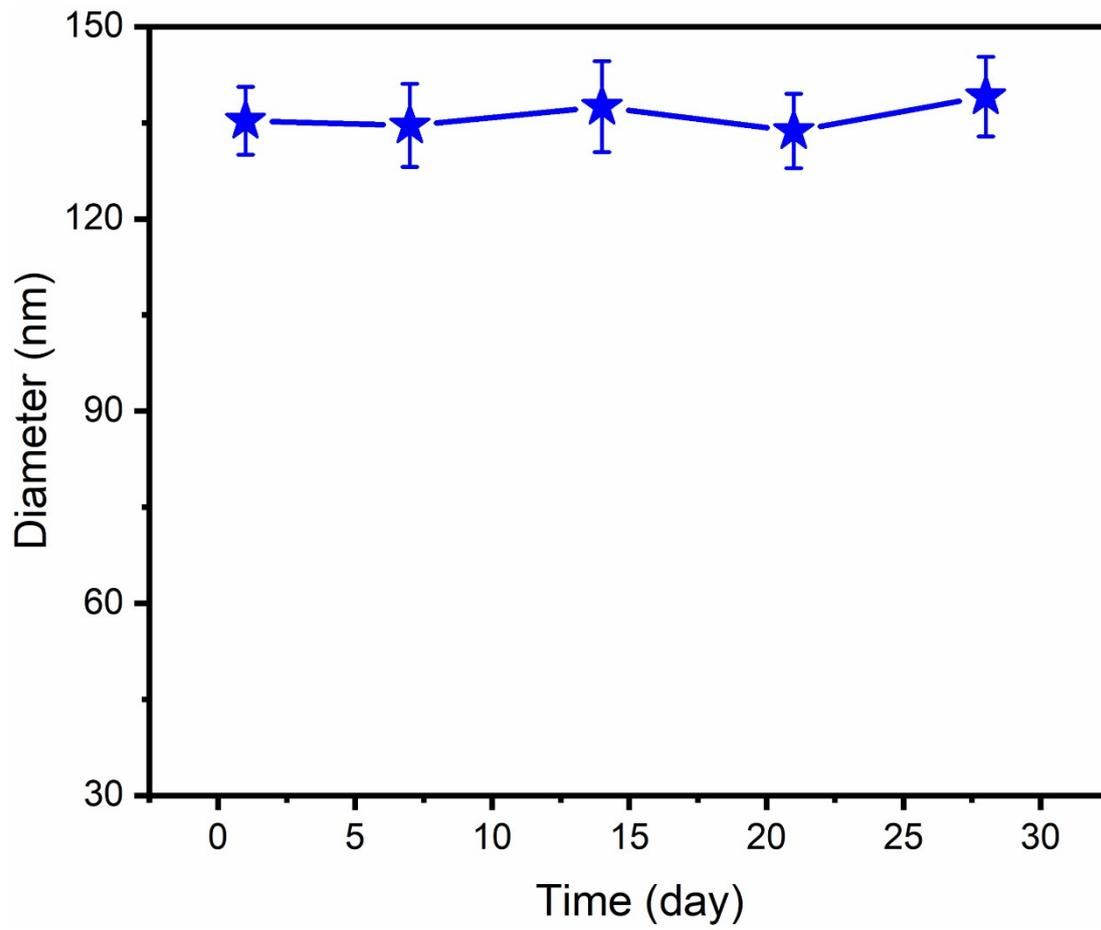
**Figure S10.** Changes in the hydration radius of the nanoprobe placed in PBS for 28 d.
