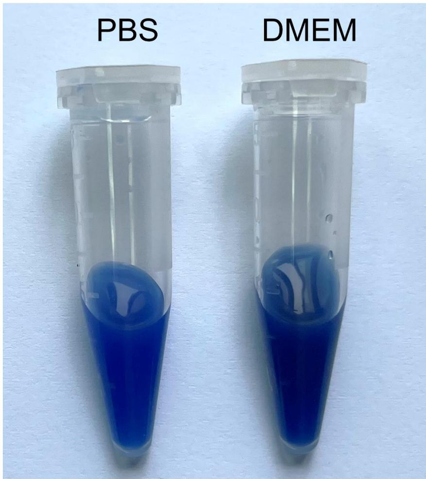
Figure S9. Photograph of nanoprobe suspended in PBS or DMEM containing 10% FBS for 28 d.
