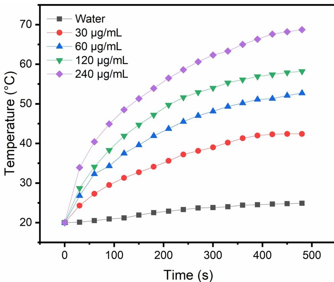
**Figure S7.** Photothermal performance of the NIR-II nanoprobes with different concentrations under 633 nm laser irradiation.
