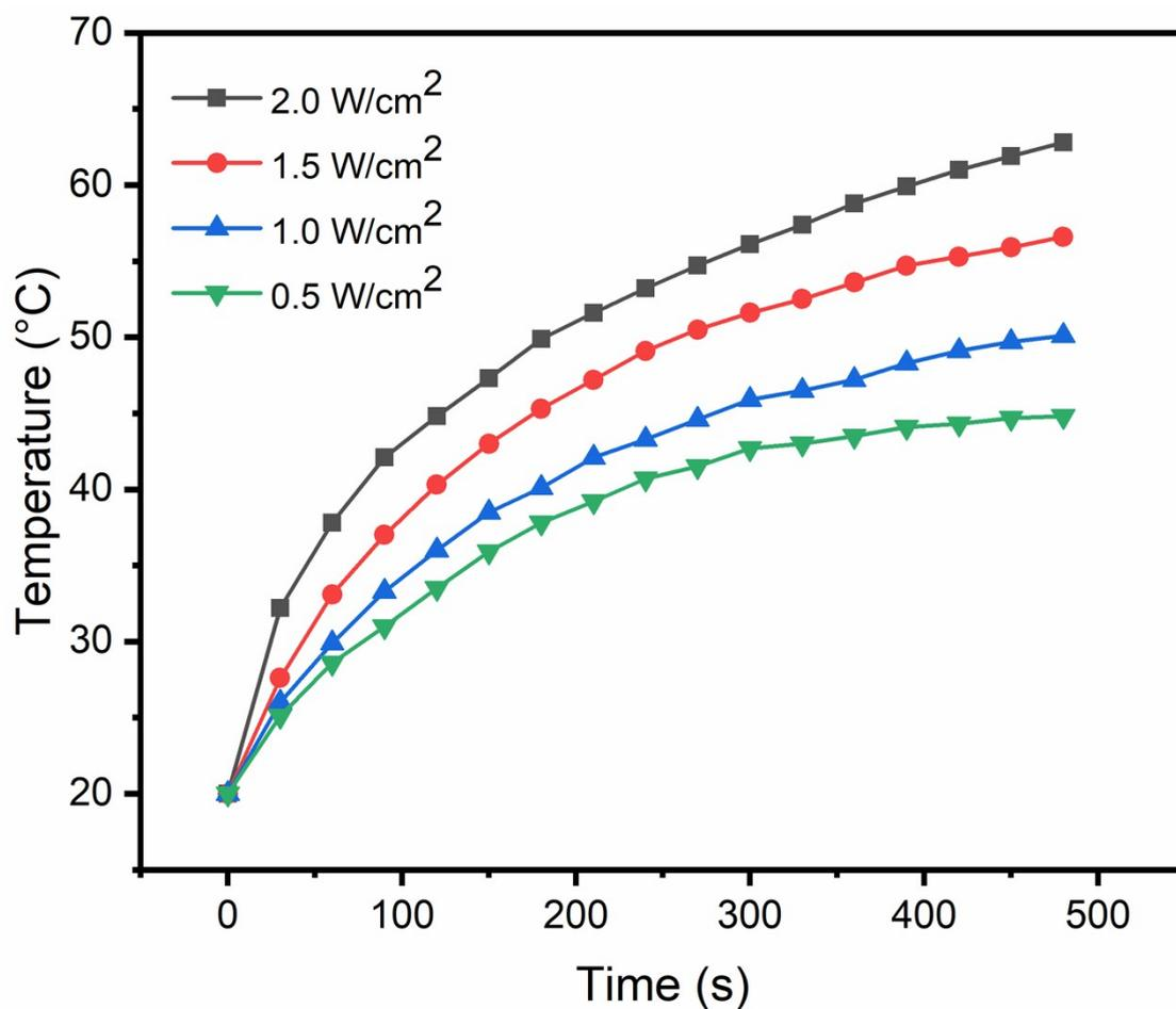
**Figure S6.** Photothermal performance of the NIR-II nanoprobe under different powers of 633 nm laser irradiation.
