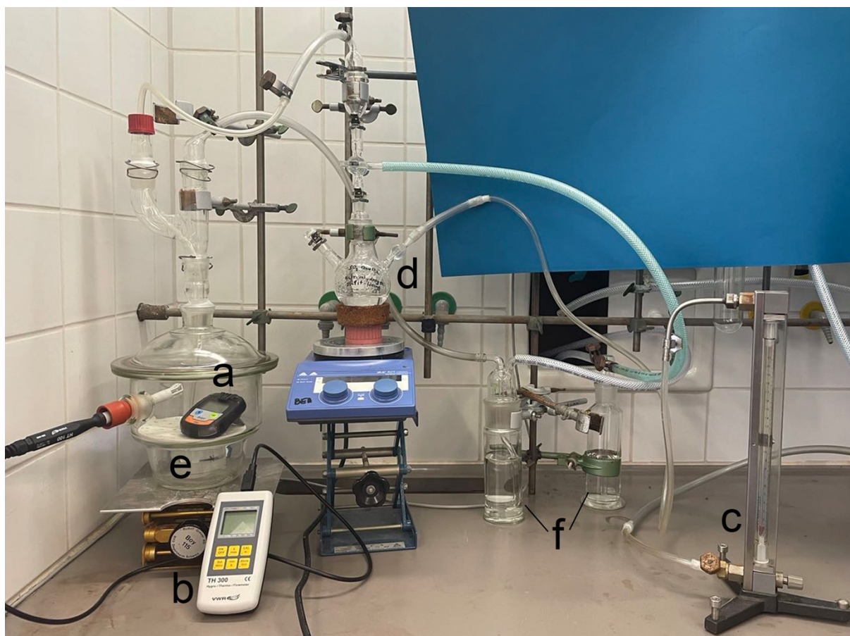
Scheme S1 Setup for humid SO 2 exposure experiments. a) SO 2 sensor, b) Hygrometer, c) Flowmeter, d) Natrium metabisulfite solution (Na 2 S 2 O 5 ), e) Sodium chloride solution, f) H 2 O.
