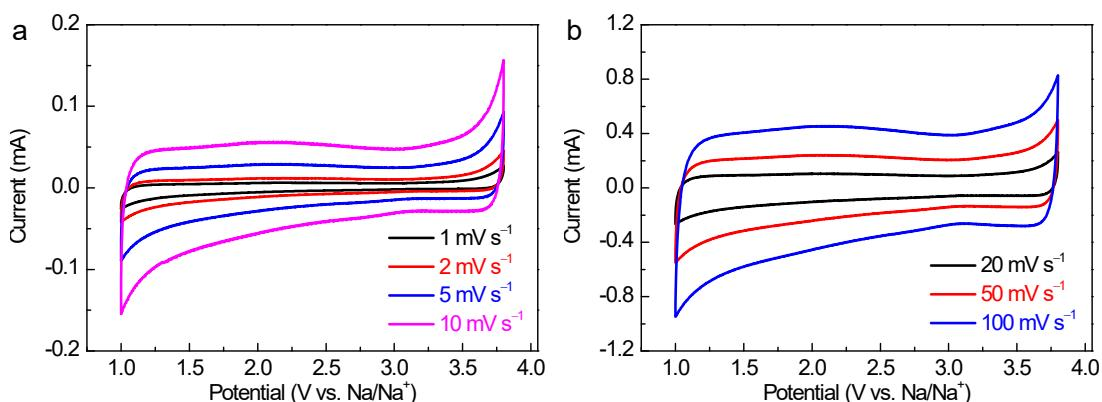
**Figure S16.** (a, b) CV curves of the ordinary carbon cathode at different scan rates ranging from 1 to 10 mV
