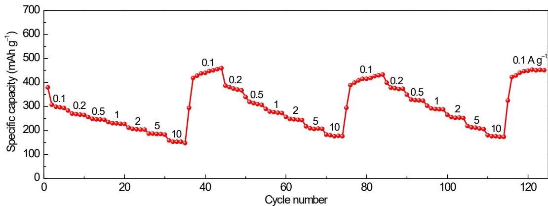
**Figure S13.** Rate capability of the HSIH-CMs anode at different current densities ranging from  $0.1$  to  $10 \text{ A g}^{-1}$ .
