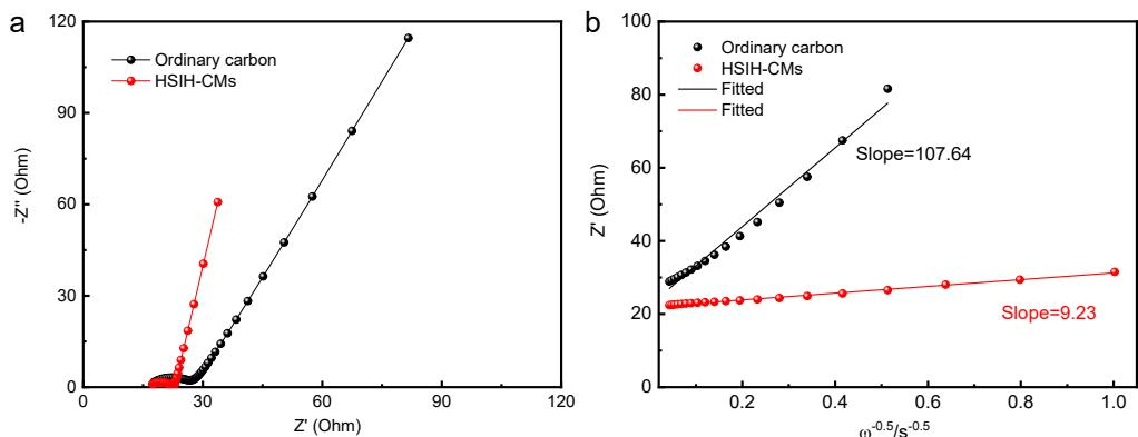
**Figure S15.** (a) Nyquist plots of the HSIH-CMs and ordinary carbon anodes after 100 cycles. (b) The  $Z' \sim \omega^{-1/2}$  plots of the HSIH-CMs and ordinary carbon anodes after 100 cycles at the low-frequency region, respectively.
