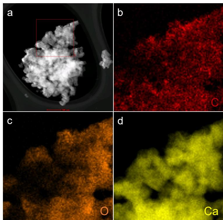
**Figure S6.** HAADF-STEM image (a) and corresponding EDX maps (b-d) of HSIH-CMs@CaO.
