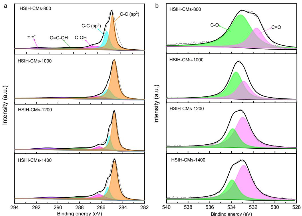
**Figure S11.** The XPS spectra for C 1s (a) and O 1s (b) of HSIH-CMs at different temperature.
