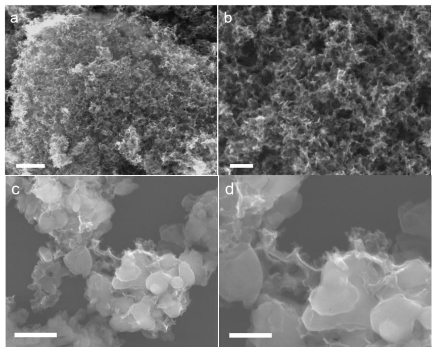
**Figure S1.** SEM images of HSIH-CMs (a, b) and HSIH-CMs@CaO (c, d). Scale bar: (a, c) 0.5  $\mu$ m; (b, d) 0.2  $\mu$ m.
