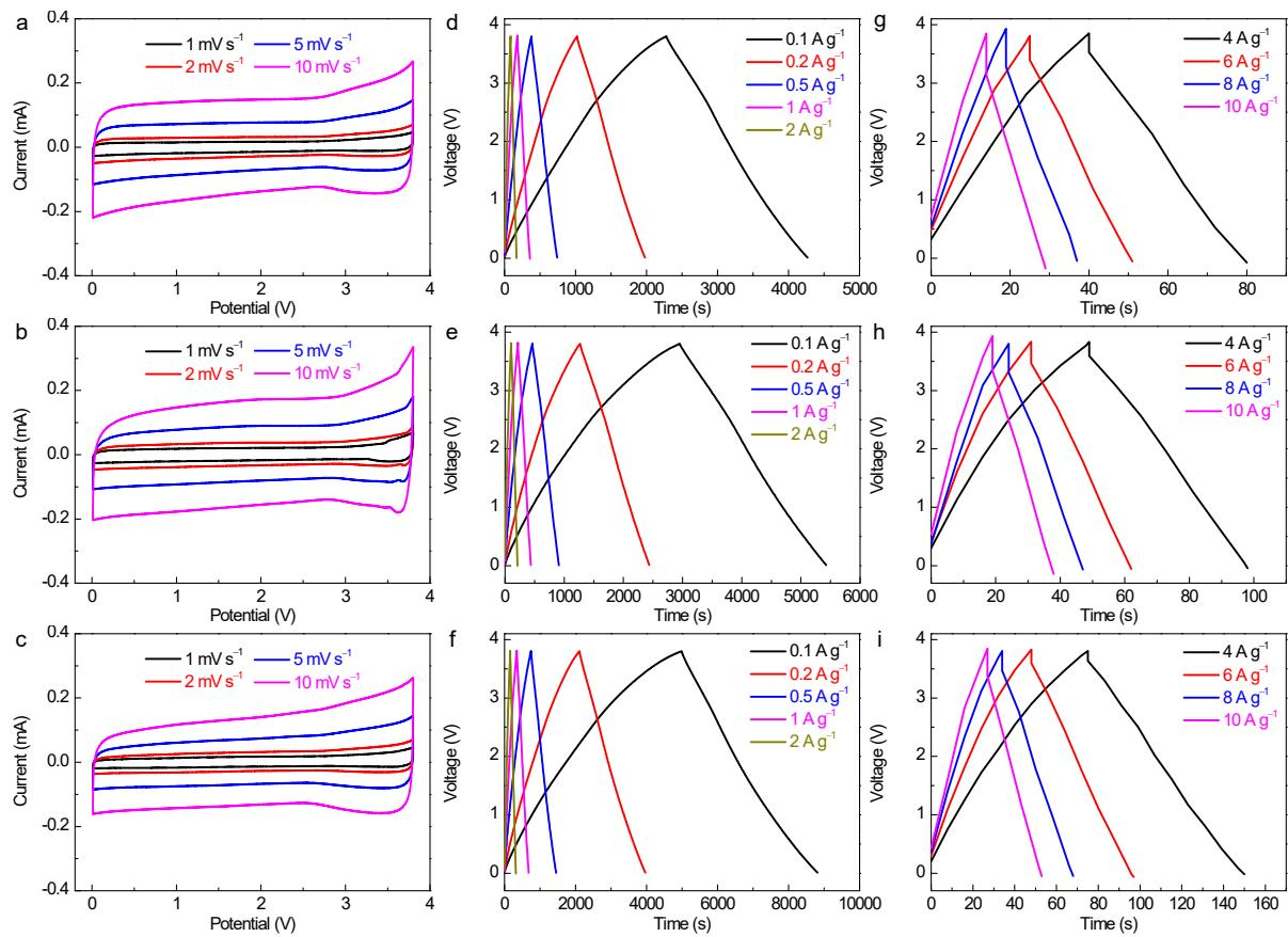
**Figure S18.** CV curves of the HSIH-CMs//HSIH-CMs SIC devices with different anode/cathode mass ratios: (a) 1:1, (b) 1:2, (c) 1:4. Galvanostatic charge-discharge curves of HSIH-CMs//HSIH-CMs SIC devices with different anode/cathode mass ratios of 1:1 (d, g), 1:2 (e, h), and 1:4 (f, i) at various current densities ranging from 0.1 to 10 A g<sup>-1</sup>.
