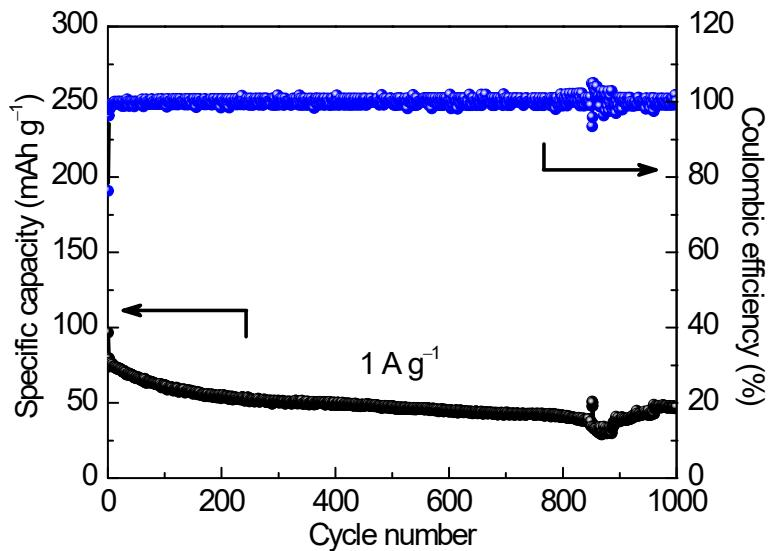
**Figure S14.** Cycling performance and corresponding Coulombic efficiency of the ordinary carbon anode at a current density of  $1 \text{ A g}^{-1}$ .
