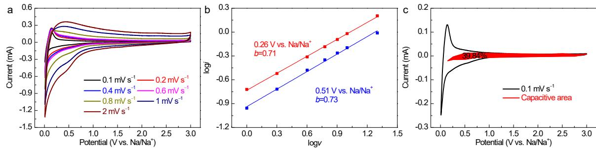
**Figure S10.** (a) CV curves of the ordinary carbon anode at various scan rates ranging from  $0.1$  to  $2\text{ mV s}^{-1}$ . (b)  $b$  values of the ordinary carbon anode at potentials of  $0.26$  and  $0.51$  V. (c) CV profile of the ordinary carbon anode with the capacitive contribution at a scan rate of  $0.1\text{ mV s}^{-1}$ .
