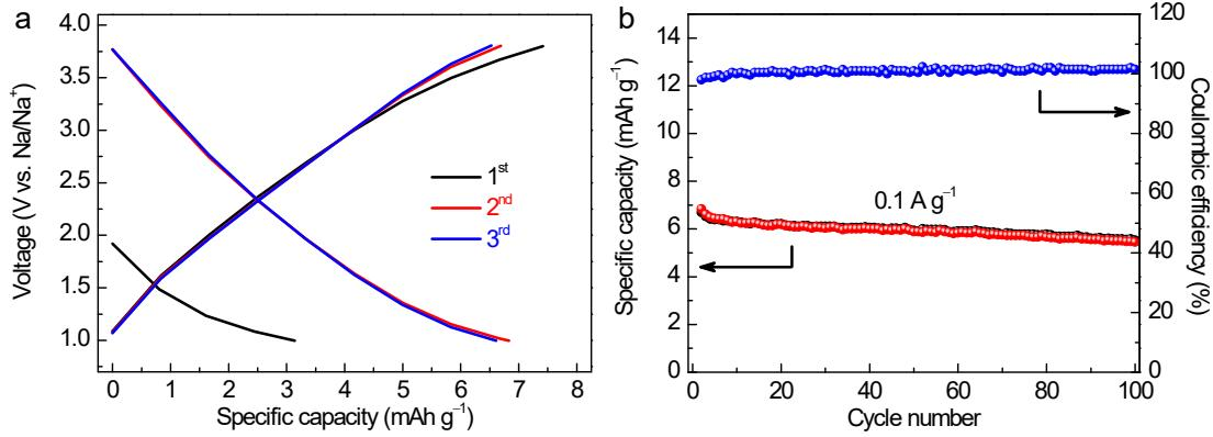
**Figure S17.** (a) The 1<sup>st</sup>, 2<sup>nd</sup> and 3<sup>rd</sup> galvanostatic charge-discharge curves of the ordinary carbon cathode at a current density of 0.1 A g<sup>-1</sup>. (b) Cycling performance and the corresponding Coulombic efficiency of the ordinary carbon cathode at current density of 0.1 A g<sup>-1</sup>.
