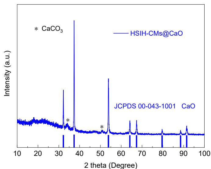
**Figure S5.** XRD pattern of the HSIH-CMs@CaO material.
