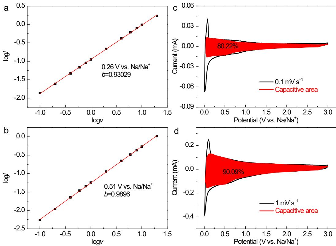
**Figure S9.** (a, b)  $b$  values of the HSIH-CMs anode at potentials of 0.26 V (a) and 0.51 V (b), respectively. (c, d) CV profiles of the HSIH-CMs with the capacitive contribution at scan rates of  $0.1 \text{ mV s}^{-1}$  (c) and  $1 \text{ mV s}^{-1}$  (d), respectively.
