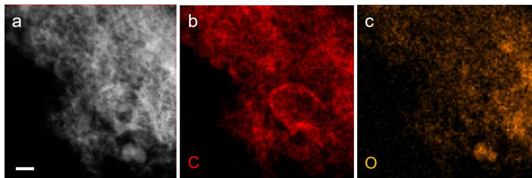
**Figure S4.** HAADF-STEM image (a) and corresponding EDX maps (b, c) of HSIH-CMs, scale bar: 100 nm.
