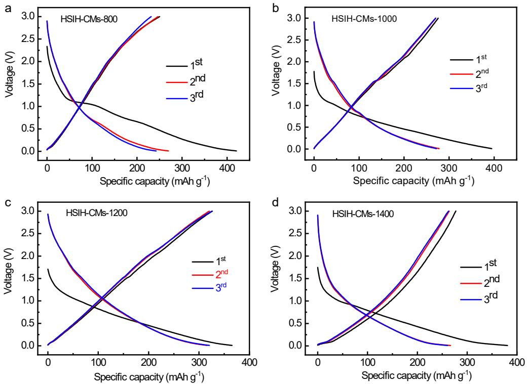
**Figure S12.** The first, second, and third galvanostatic discharge–charge profiles of (a) HSIH-CMs-800, (b) HSIH-CMs-1000, (c) HSIH-CMs-1200 and (d) HSIH-CMs-1400 anode at a current density of  $100 \text{ mA g}^{-1}$ .
