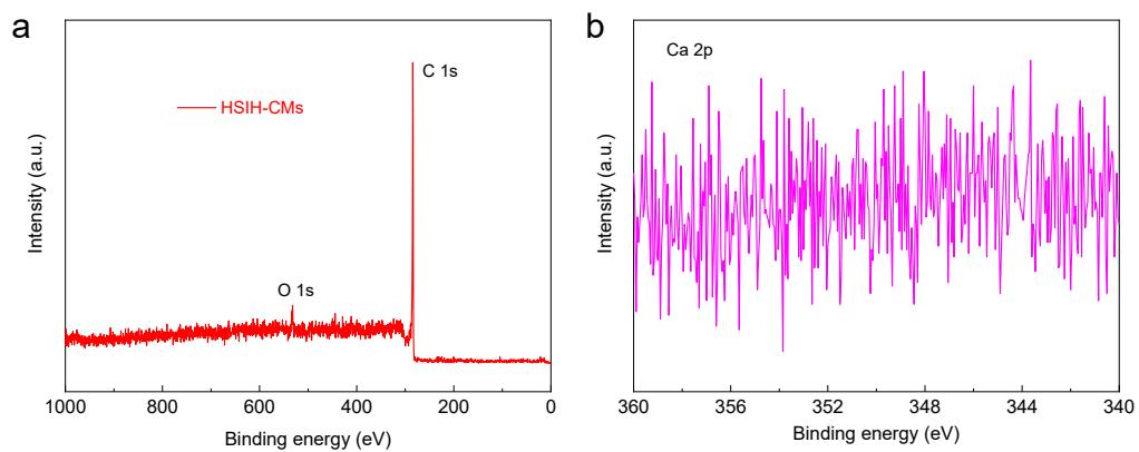
**Figure S7.** The XPS survey spectra (a) and Ca 2p spectra (b) of HSIH-CMs.
