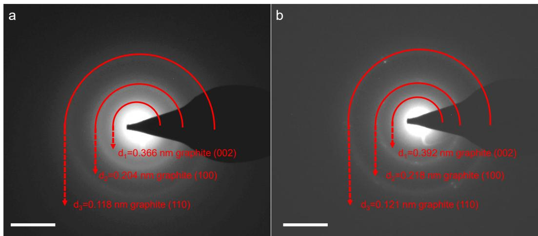
**Figure S3.** SAED patterns of the ordinary carbon (a) and HSIH-CMs (b) materials, respectively. Scar bar: (a) 5 1/nm; (b) 5 1/nm.
