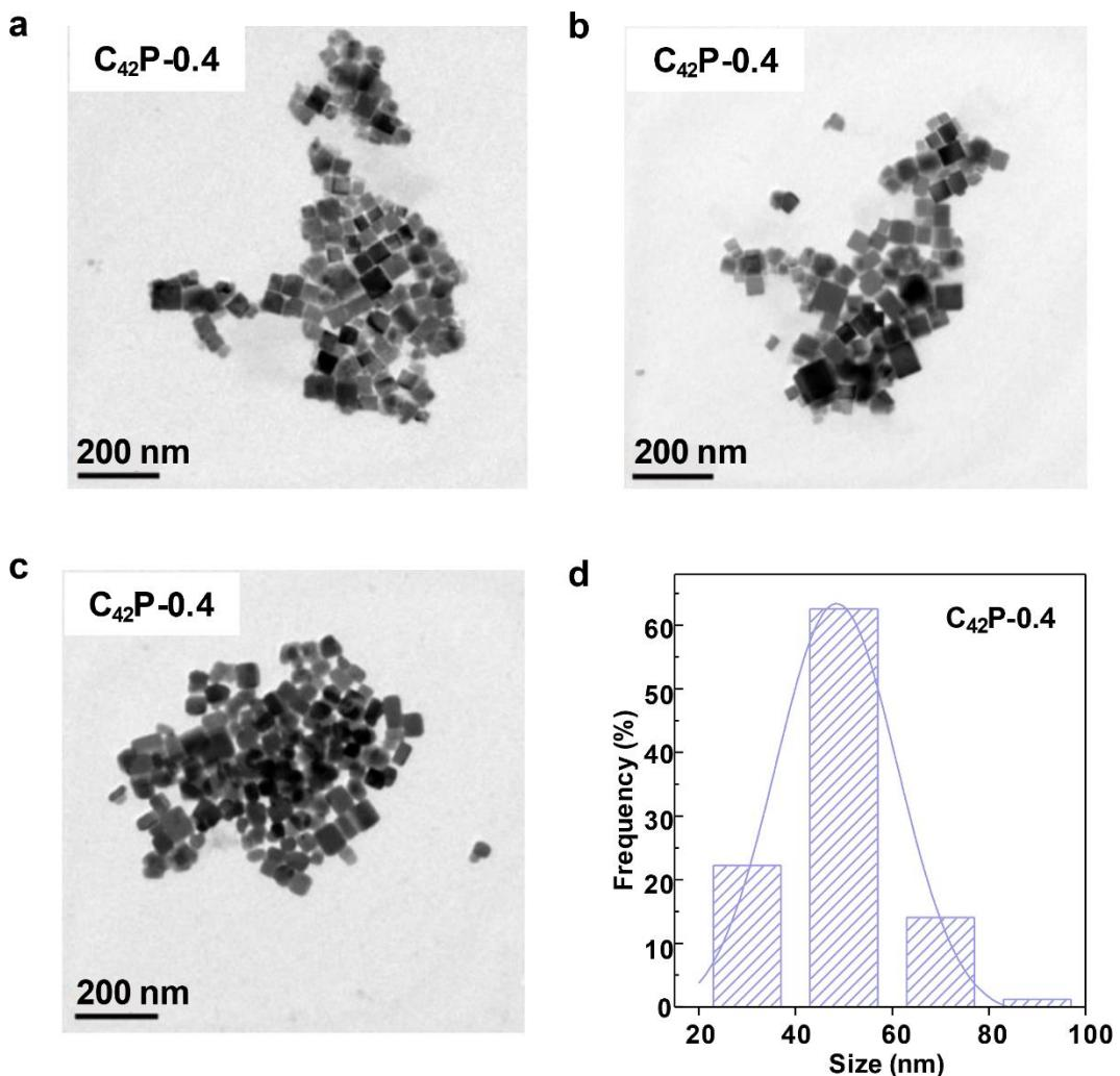
**Figure S6.** (a-c) Multiple TEM images of C<sub>42</sub>P-0.4. (d) Size-distribution histogram of C<sub>42</sub>P-0.4 based on multiple TEM images.
