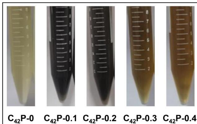
**Figure S2.** Photographs of the CsSnI<sub>3</sub> NCs supernatant obtained after the first centrifugation. The samples were synthesized with different ratios of C<sub>42</sub>P to Cs.
