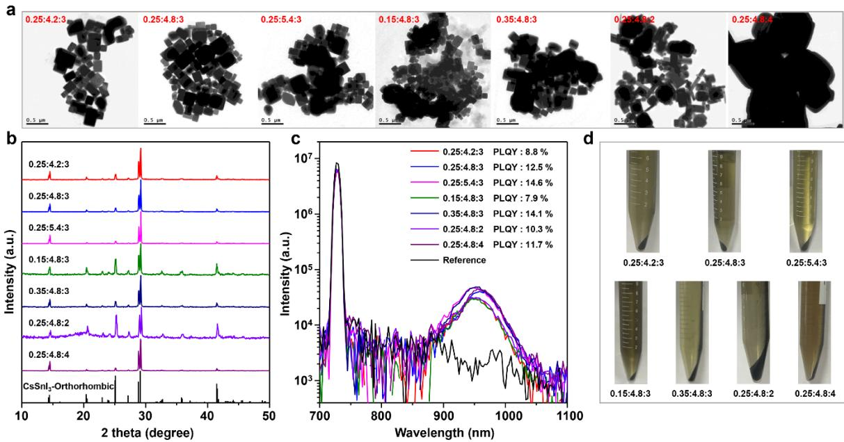
**Figure S1.** a-c) TEM images (a), XRD patterns (b), and PLQY measurements (c) of large-sized CsSnI<sub>3</sub> synthesized with different Cs:Sn:I precursor ratios. All samples are large-sized precipitates obtained after the first centrifugation of the crude solution. d) Photographs of the CsSnI<sub>3</sub> solution with different Cs:Sn:I precursor ratios after the first centrifugation. The detailed synthetic parameters are shown in **Table S1**.
