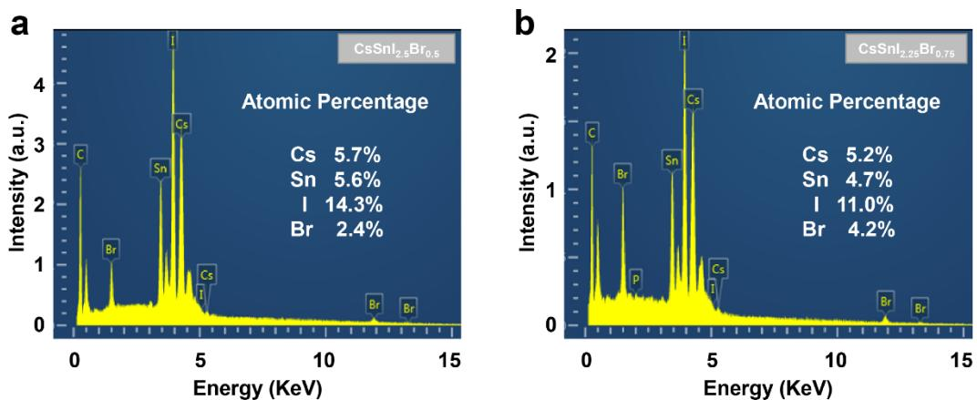
**Figure S15.** EDS spectra of (a)  $\text{CsSnI}_{2.5}\text{Br}_{0.5}$  and (b)  $\text{CsSnI}_{2.25}\text{Br}_{0.75}$  NCs synthesized with  $\text{C}_{42}\text{P}$ .
