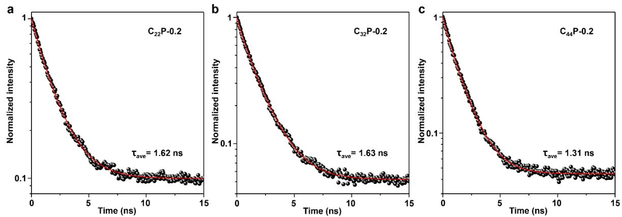
**Figure S12.** PL decay traces (black dots) and fitted curves (red lines) of (a)  $\text{C}_{22}\text{P}-0.2$ , (b)  $\text{C}_{32}\text{P}-0.2$ , and (c)  $\text{C}_{44}\text{P}-0.2$ .
