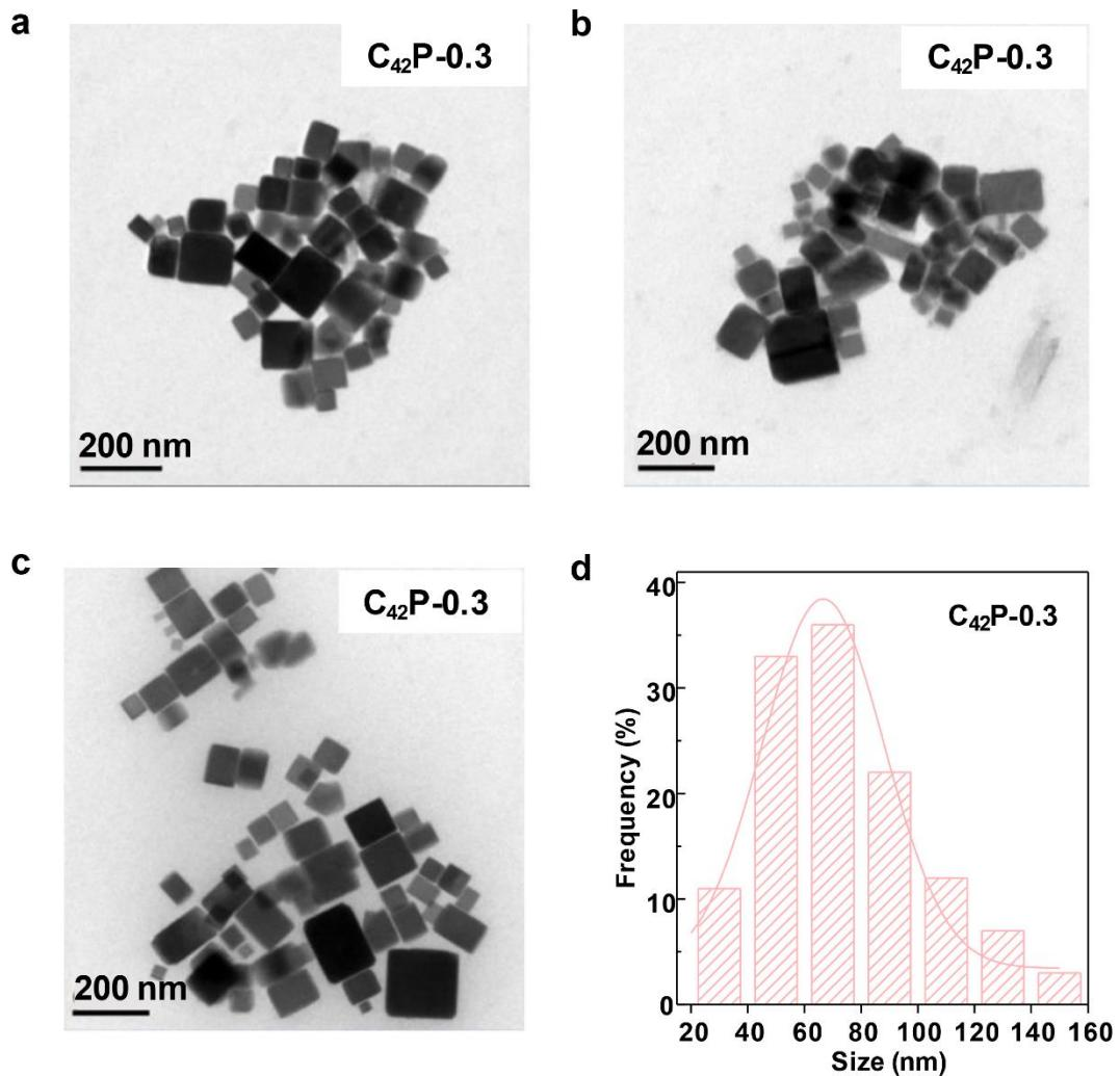
**Figure S5.** (a-c) Multiple TEM images of C<sub>42</sub>P-0.3. (d) Size-distribution histogram of C<sub>42</sub>P-0.3 based on multiple TEM images.
