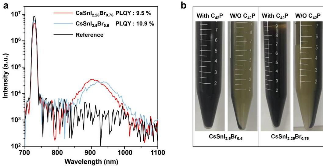
**Figure S16.** (a) PLQY measurements of  $\text{CsSnI}_{2.5}\text{Br}_{0.5}$  and  $\text{CsSnI}_{2.25}\text{Br}_{0.75}$  NCs synthesized with  $\text{C}_{42}\text{P}$ . (b) Photographs of  $\text{CsSnI}_{2.5}\text{Br}_{0.5}$  and  $\text{CsSnI}_{2.25}\text{Br}_{0.75}$  crude solution after the first centrifugation. The samples were synthesized with and without (W/O)  $\text{C}_{42}\text{P}$ . We note that NCs cannot be obtained in the absence of  $\text{C}_{42}\text{P}$ .
