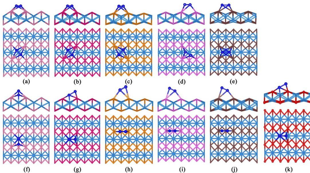
**Fig. S5** The side and top views of structures for  $N_2$  molecules with (a-e) side-on adsorption configurations on ScB, TiB, CrB, MoB, WB monolayer, respectively, and (f-k) end-on adsorption configurations on ScB, TiB, CrB, MoB, WB, VB monolayers, respectively.
