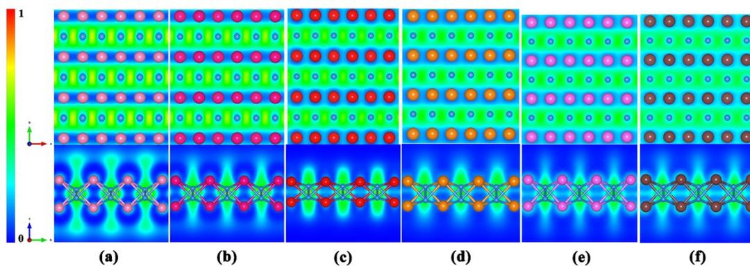
**Fig. S3** The electron localization functions (ELFs) of (a) ScB, (b) TiB, (c) CrB, (d) MoB, (e) WB, (f) VB monolayers from top (001) and side (100) views. ELF=0 means that the electrons are completely delocalized or do not exist, and ELF=1 illustrates that the electrons are completely localized.
