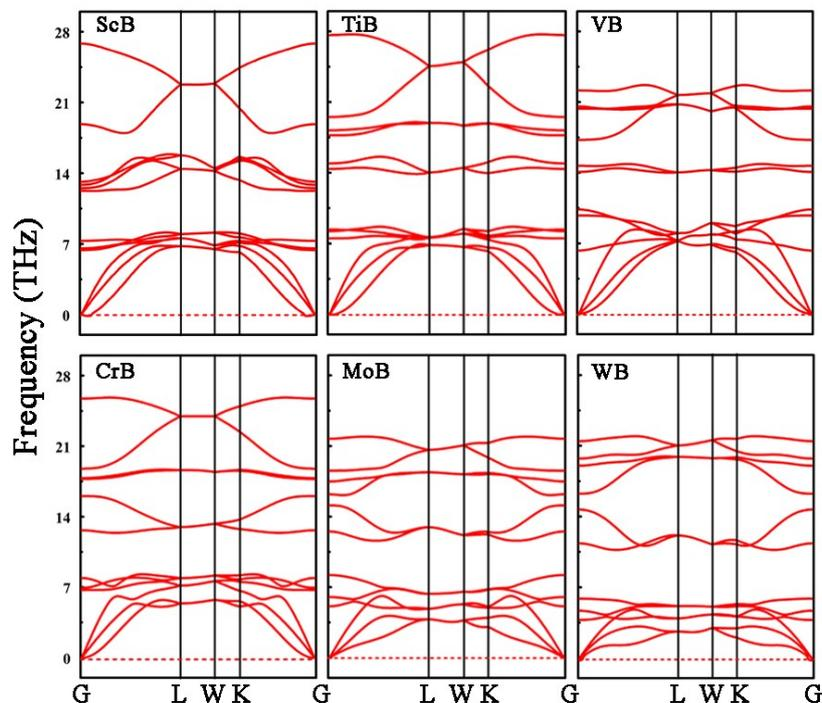
**Fig. S2** The calculated phonon dispersion curves of MB (M=Sc, Ti, V, Cr, Mo, and W) monolayers.
