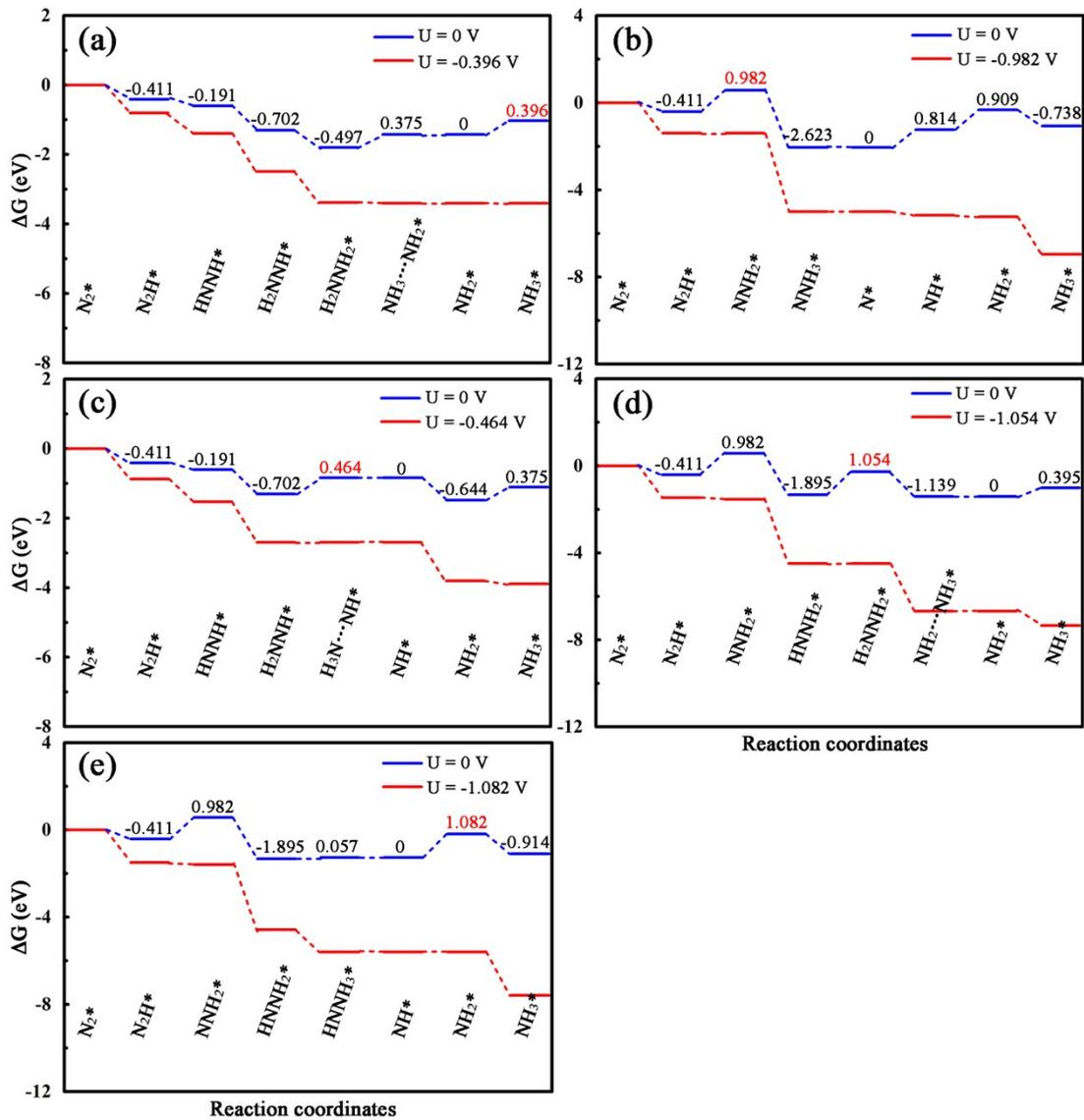
**Fig. S8** Free energy diagrams of  $N_2$  conversion into ammonia on VB monolayer via five different reaction pathways at  $N_2$  adsorption configurations with (a-e) end-on type, respectively.
