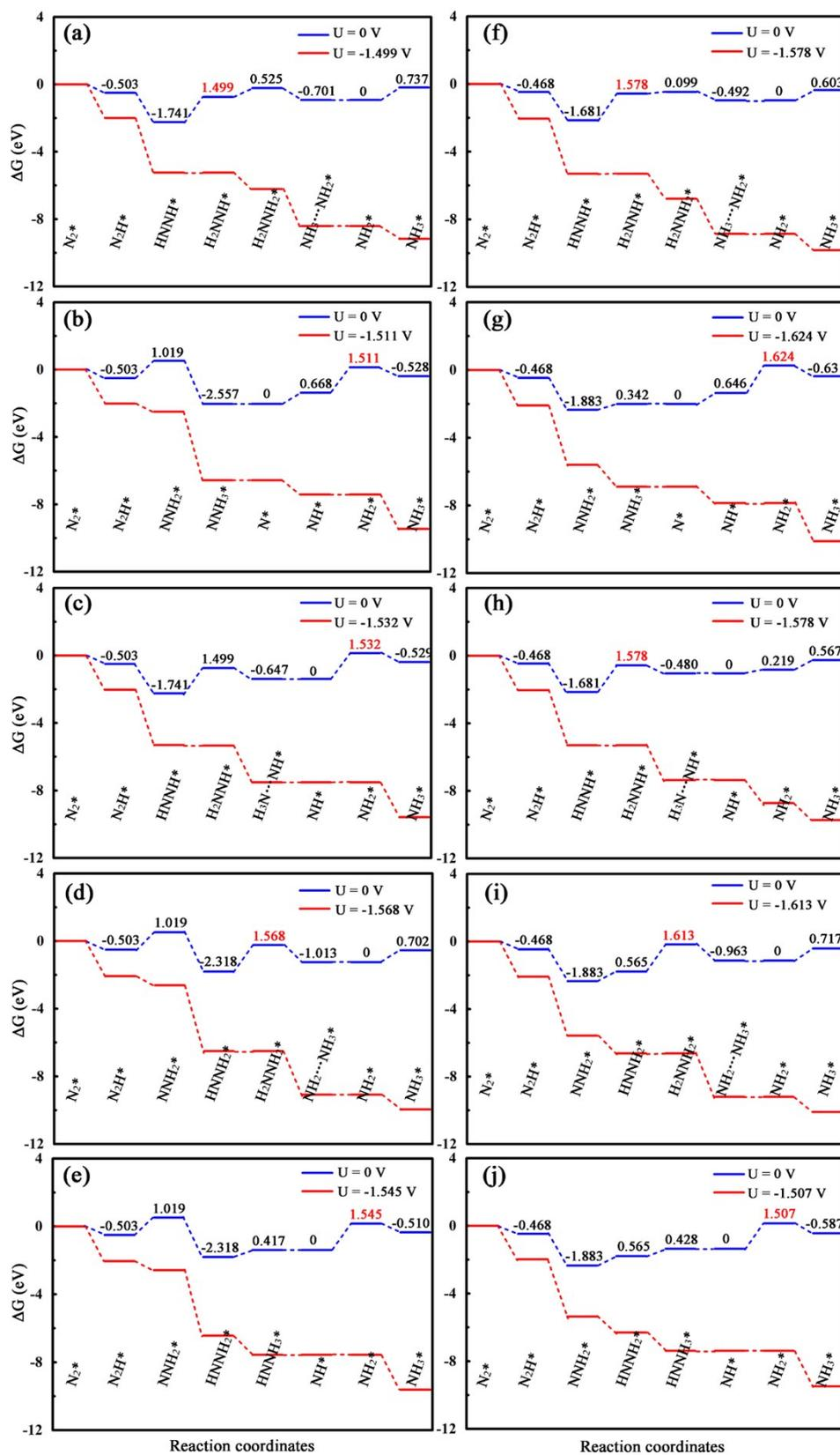
**Fig. S6** Free energy diagrams of  $N_2$  conversion into ammonia on ScB monolayer *via* five different reaction pathways at  $N_2$  adsorption configurations with (a-e) side-on and (f-j) end-on types, respectively.
