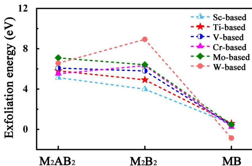
**Fig. S1** The calculated exfoliation energy from MAB to  $M_2AB_2$ , and from  $M_2AB_2$  to  $M_2B_2$ , and from  $M_2B_2$  to MB (M=Sc, Ti, V, Cr, Mo, and W; A=Al).
