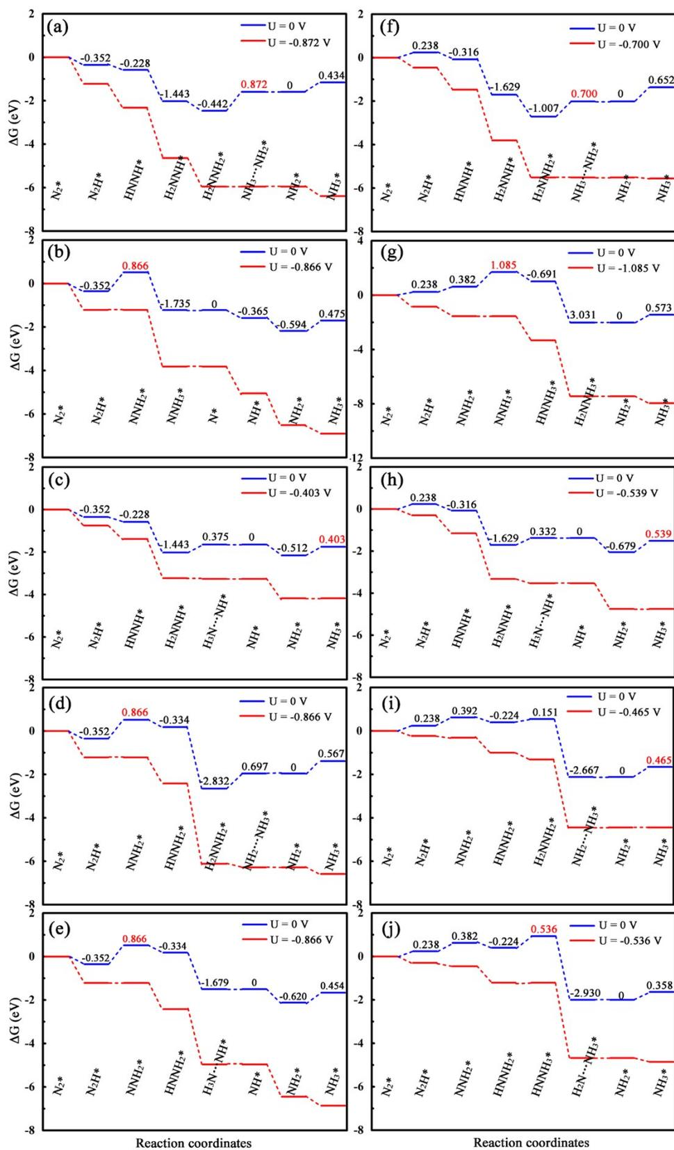
**Fig. S10** Free energy diagrams of  $N_2$  conversion into ammonia on MoB monolayer *via* five different reaction pathways at  $N_2$  adsorption configurations with (a-e) side-on and (f-j) end-on types, respectively.
