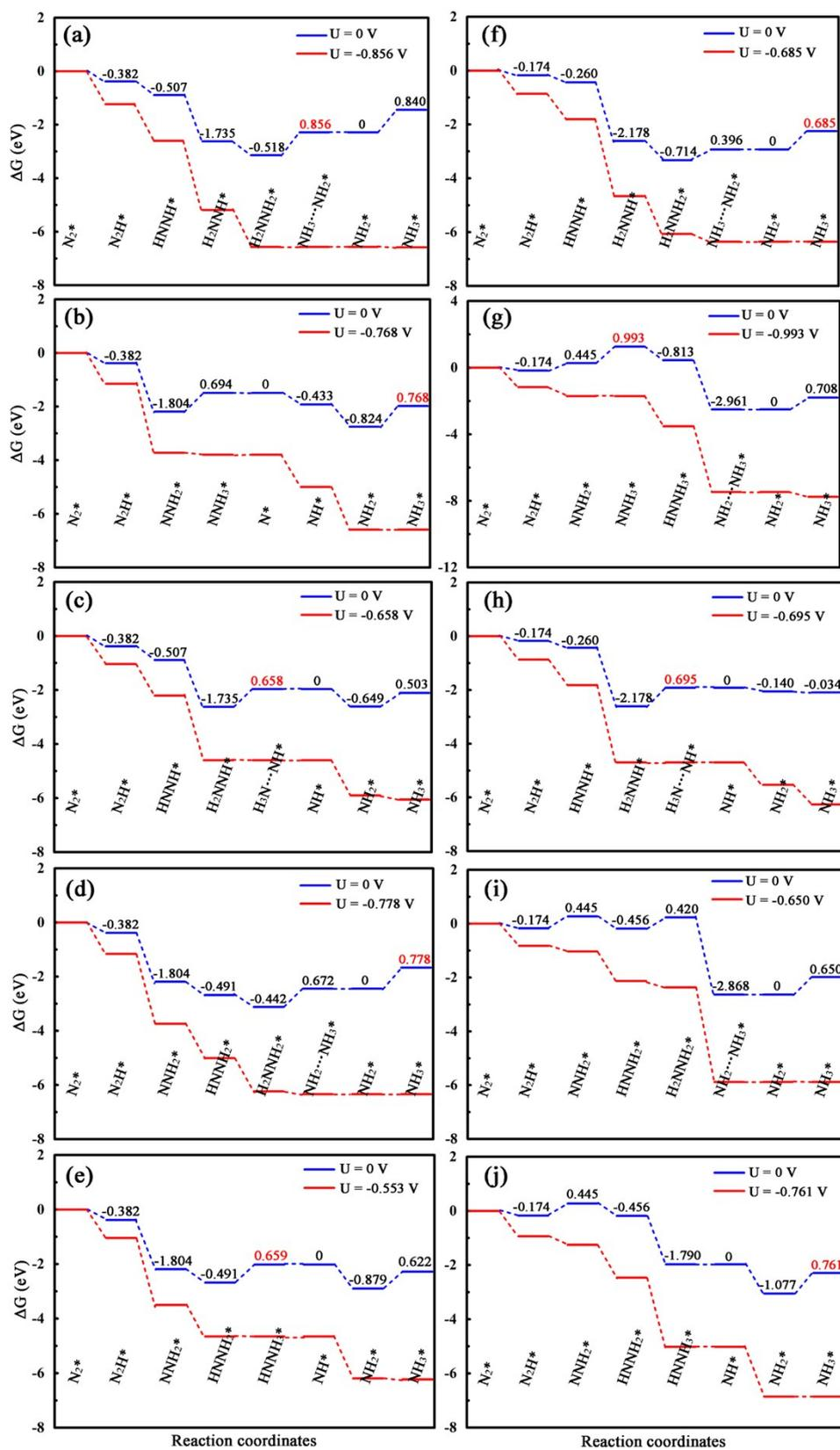
**Fig. S11** Free energy diagrams of  $N_2$  conversion into ammonia on WB monolayer via five different reaction pathways at  $N_2$  adsorption configurations with (a-e) side-on and (f-j) end-on types, respectively.
