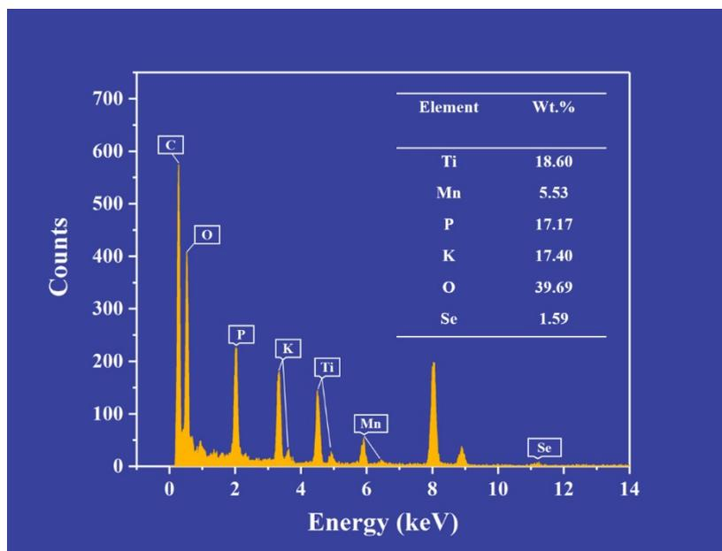
**Fig. S12** EDS tests of the F-MTP/C NFF electrode after long-term cycles.
