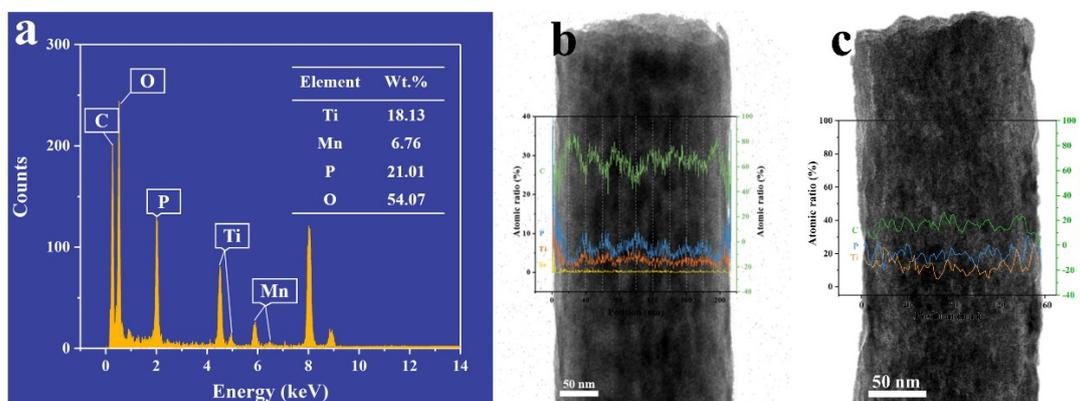
**Fig. S4** a.) EDS spectrum of MTP/C NFF. b) TEM-EDX lines scan of the atomic ratio of the elements (C, Ti, P and Se) of F-MTP/C NFF and c) MTP/C NFF.
