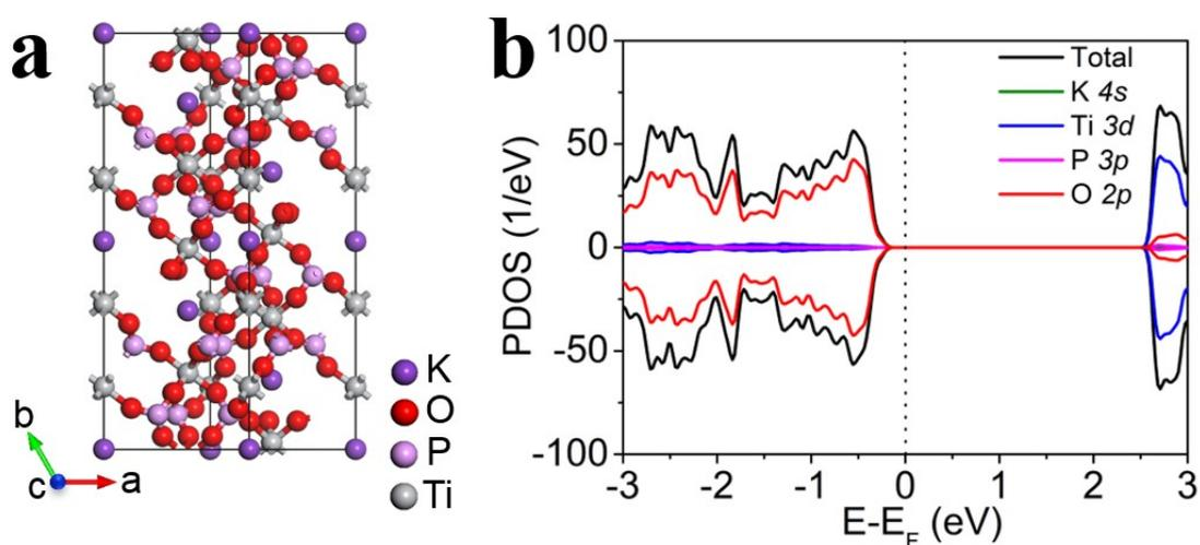
**Fig. S1** DFT-optimized geometry of KTP crystals; b) Projected densities of states (PDOS) of KTP crystals, as obtained at the DFT/PBE-D3 level.
