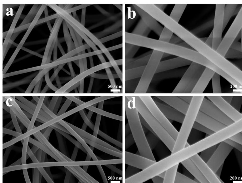
**Fig. S2** FE-SEM images of precursor nanofibers of a, b) F-MTP/C NFF and c, d) MTP/C NFF.
