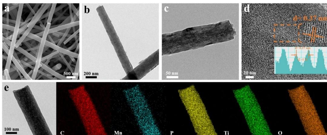
**Fig. S3** a) FE-SEM image; b, c) TEM images; d) HR-TEM image; e) Element mapping images of MTP/C NFF.
