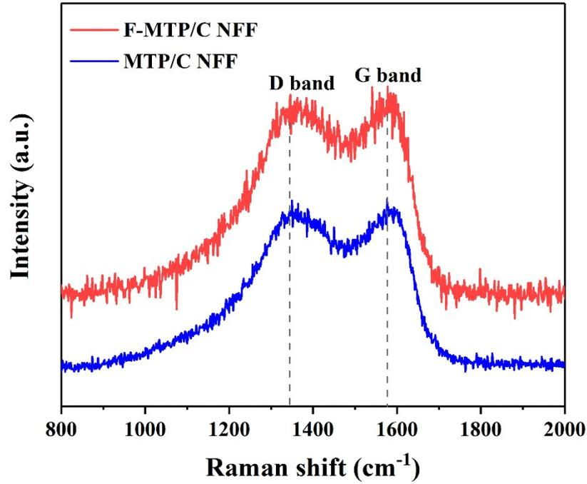
Fig. S7 Raman spectrums of F-MTP/C NFF and MTP/C NFF.
