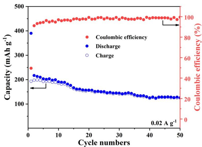
Fig. S10 Cycling performance of MTP/C NFF electrode at current density of 0.02 A g<sup>-1</sup>.
