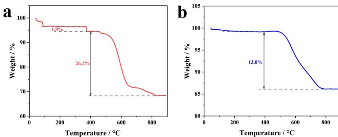
Fig. S6 TG curves in the air atmosphere of a) F-MTP/C NFF; b) MTP/C NFF.
