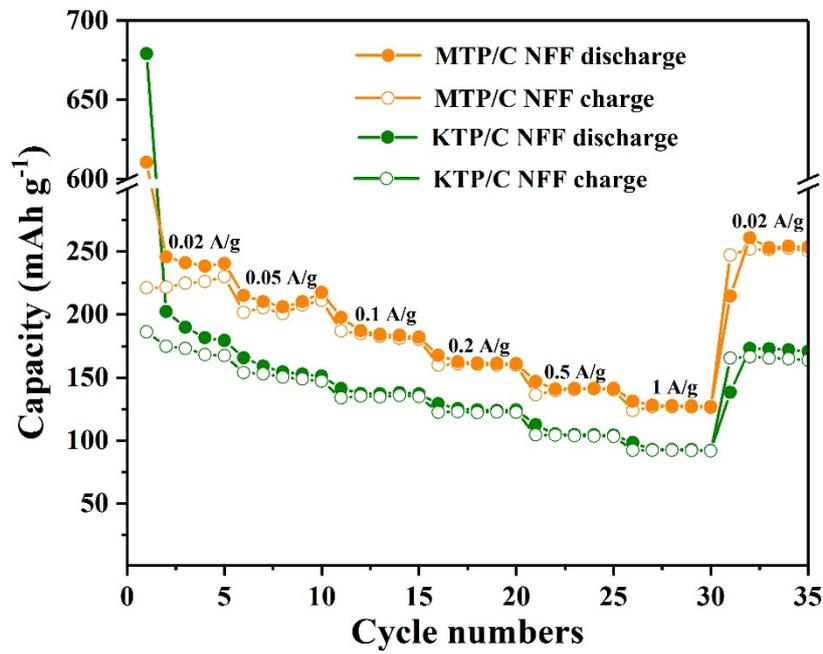
Fig. S8 Rate performance of MTP/C NFF and KTP/C NFF powder.
