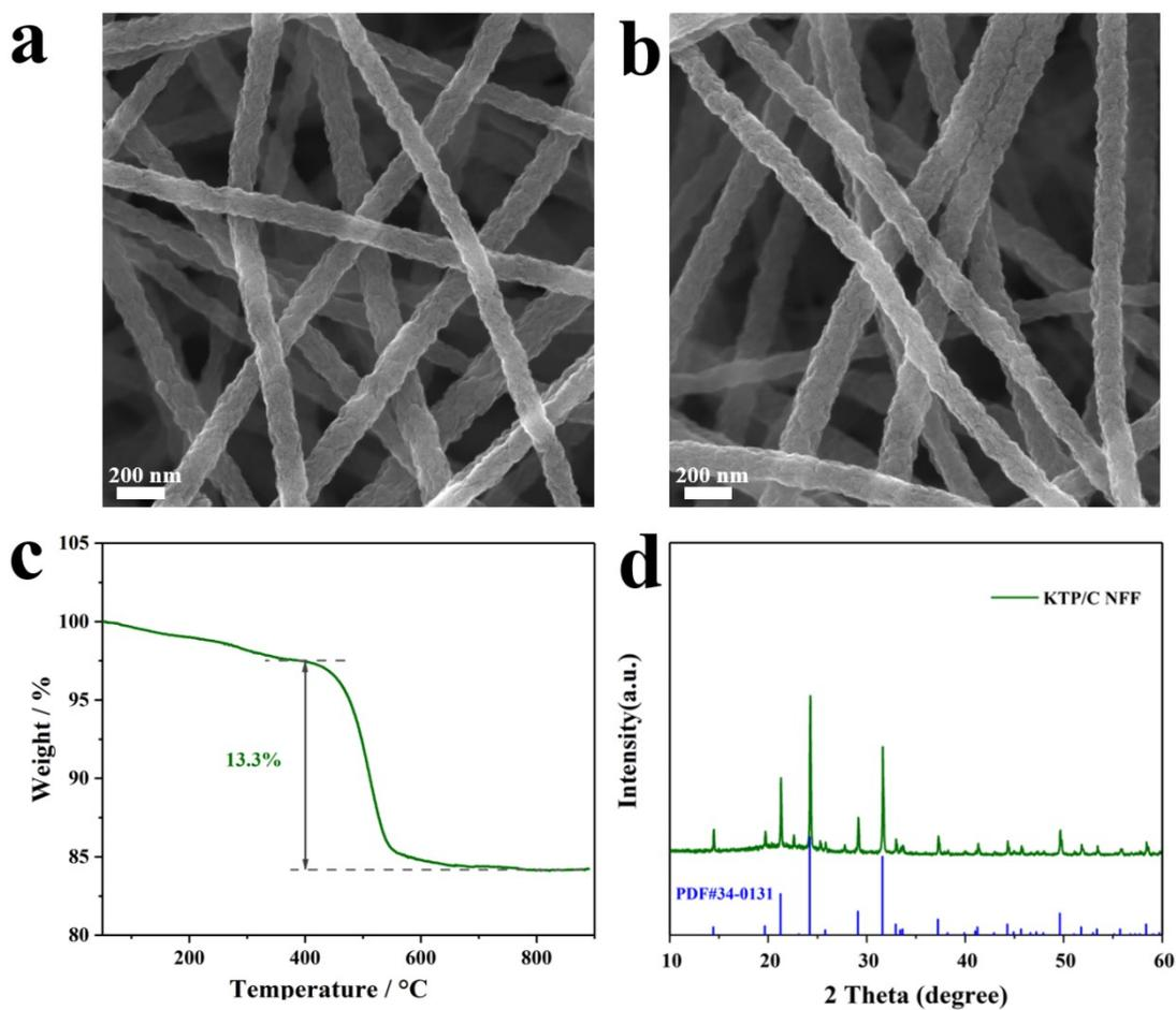
Fig. S9 a, b) FE-SEM images; c) TG curve; d) XRD image of the KTP/C NFF.
