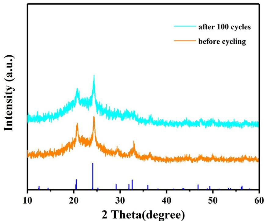
**Fig. S11** The XRD patterns of the F-MTP/C NFF electrode before and after cycling at a current density of  $1 \text{ A g}^{-1}$ .
