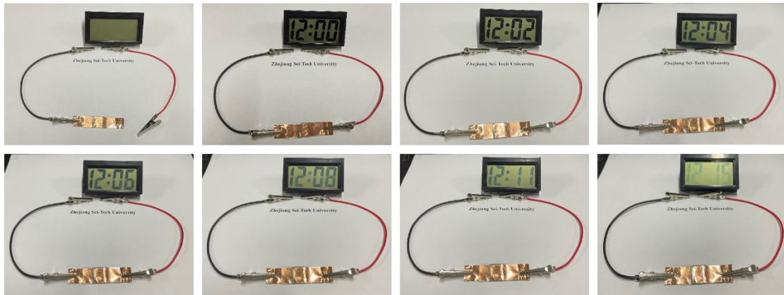
Figure S15. Photographs of electronic watch powered using CNFAs-8%/CNFAs-8% symmetric supercapacitor.
