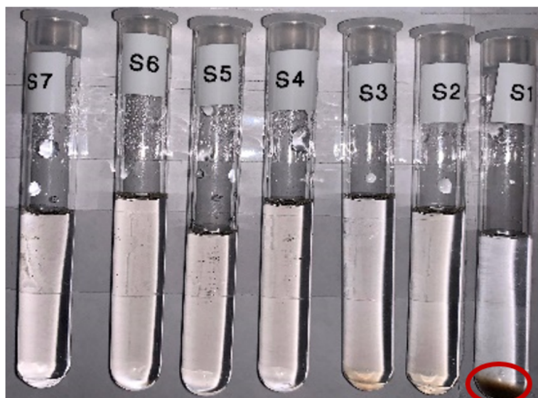
Figure S4: Photographic images of the DND suspensions ( 0.1 \text{ mg mL}^{-1} ) with different ionic strengths, at higher salt concentrations (S1) the ND particles aggregated strongly and precipitated as shown.
