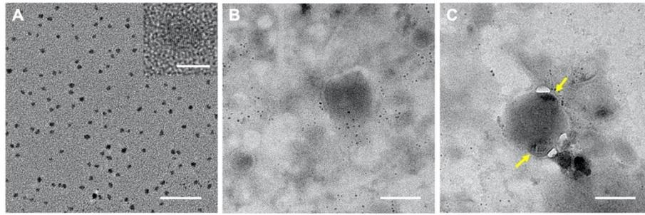
**Fig. S5** (A) HRTEM image of Ag<sub>2</sub>Se QDs. Scale bar: 50 nm. Inset: HRTEM image of a single Ag<sub>2</sub>Se QD. Scale bar: 5 nm. (B and C) HRTEM images of F-L-particles incubated Ag<sub>2</sub>Se QDs without and with electroporation. Scale bars: 100 nm.
