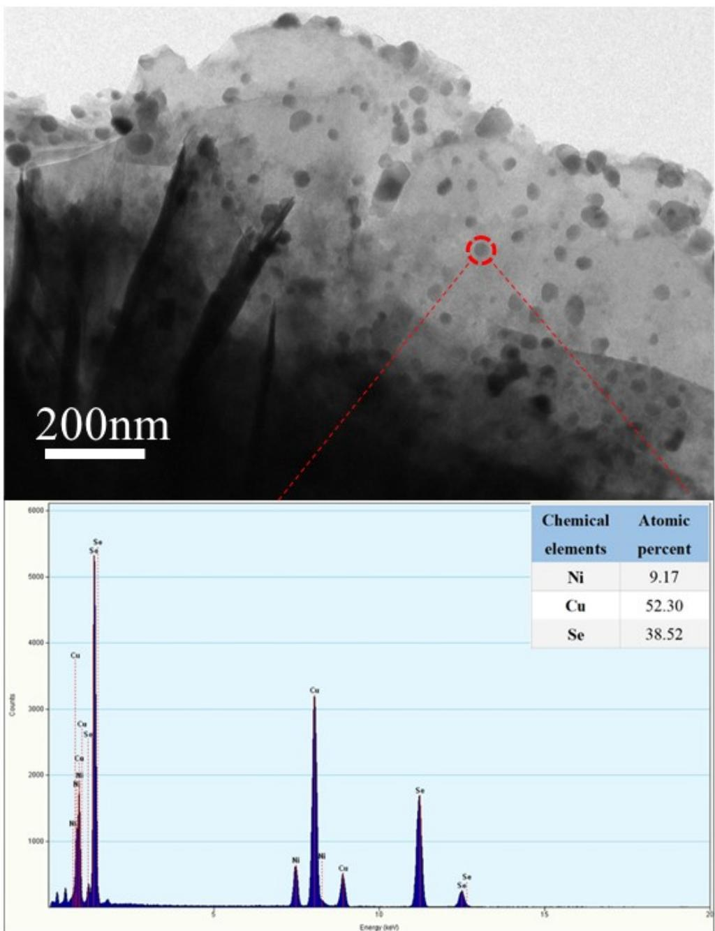
**Fig. S7.** EDS-point data of  $\text{NiSe}_2@\text{CuSe}_2/\text{NF}$ . Inset image is a table of atomic percent of Ni, Cu and Se.
