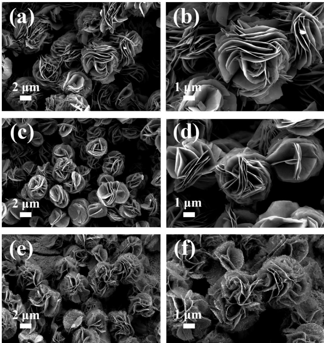
**Fig. S9.** SEM and magnified SEM images of  $\text{NiSe}_2@\text{CuSe}_2/\text{NF}$  at different hydrothermal temperatures: a-b) 120 °C, c-d) 160 °C , and e-f) 200 °C .
