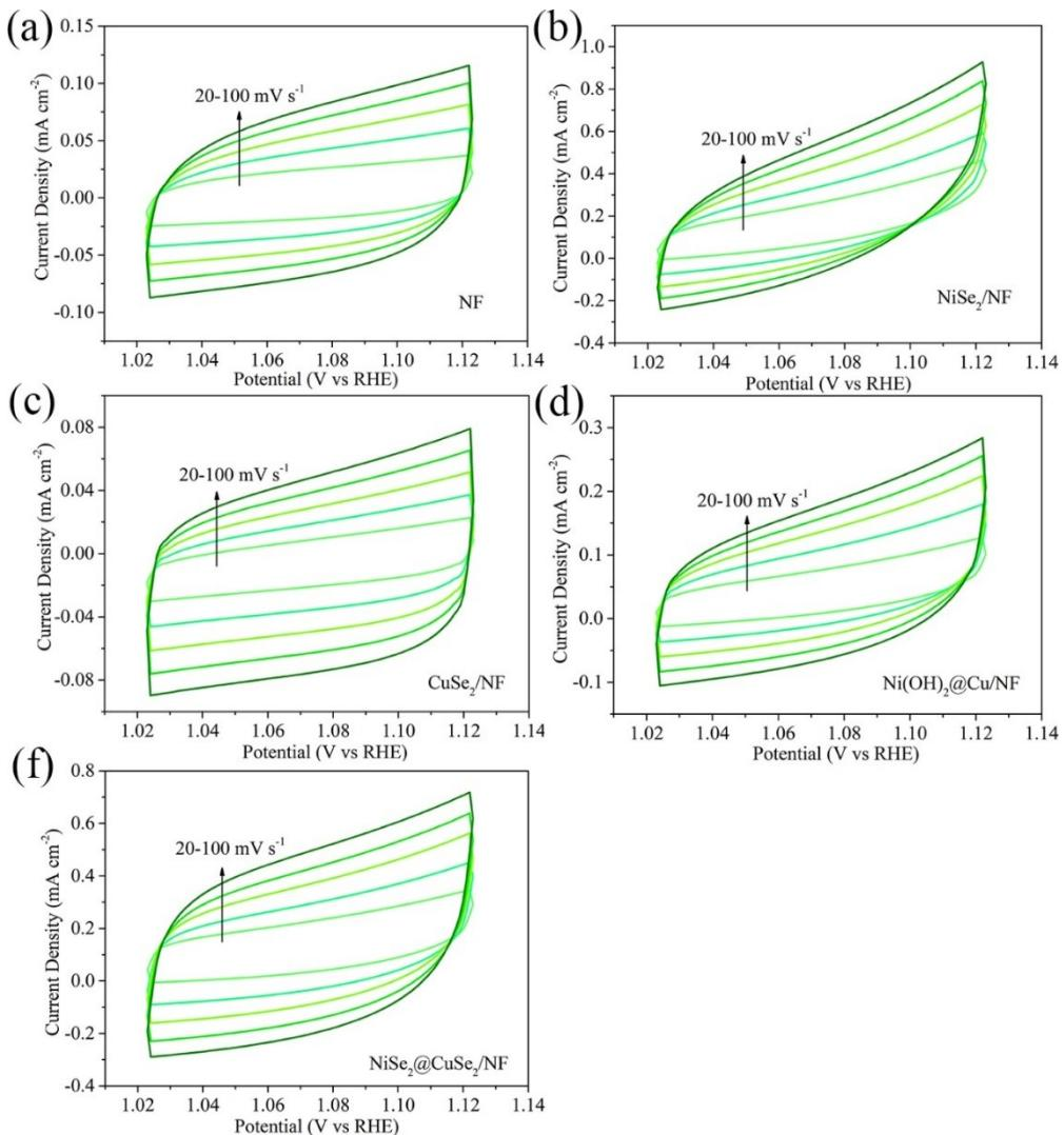
**Fig. S10.** CV curves at different scan rates for catalysts: a) NF, b) NiSe<sub>2</sub>/NF, c) CuSe<sub>2</sub>/NF, d) Ni(OH)<sub>2</sub>@Cu/NF, and e) NiSe<sub>2</sub>@CuSe<sub>2</sub>/NF.
