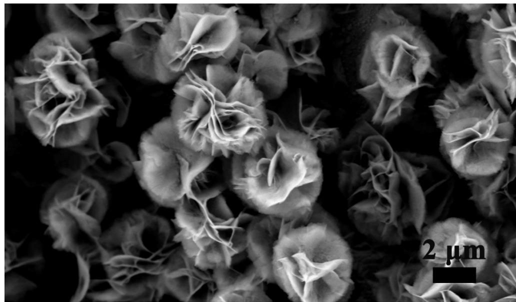
**Fig. S2.** SEM image of  $\text{Ni(OH)}_2@\text{Cu/NF}$ .
