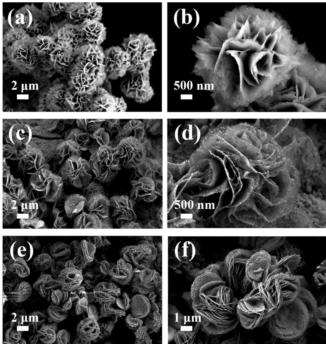
**Fig. S6.** SEM and magnified SEM images of a-b) NiCuSe-NF-0.1, c-d) NiCuSe-NF-0.2 e-f) NiCuSe-NF-0.3 (0.1, 0.2, 0.3 represent the ratio of nickel salt to copper salt).
