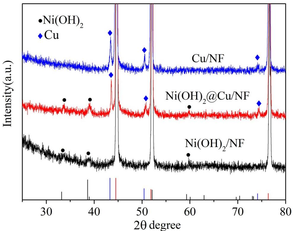
**Fig. S1.** XRD pattern of  $\text{Ni(OH)}_2@\text{Cu/NF}$ ,  $\text{Ni(OH)}_2/\text{NF}$  and  $\text{Cu/NF}$ .
