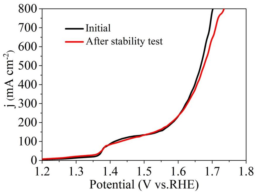
**Fig. S12.** LSV curves of  $\text{NiSe}_2@\text{CuSe}_2/\text{NF}$  before and after the test.
