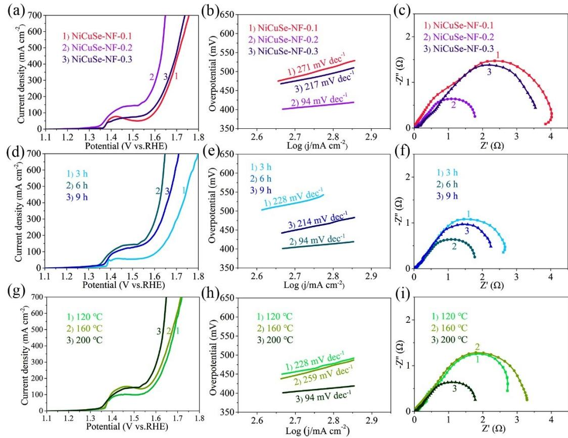
**Fig. S16.** a) OER polarization curves, b) Tafel slopes, c) Nyquist plots of NiCuSe-NF-0.1, NiCuSe-NF-0.2 and NiCuSe-NF-0.3. d) OER polarization curves, e) Tafel slopes, and f) Nyquist plots of different hydrothermal time (3 h, 6 h, 9 h). g) OER polarization curves, h) Tafel slopes, and i) Nyquist plots of different hydrothermal temperature (120 °C, 160 °C, 200 °C).
