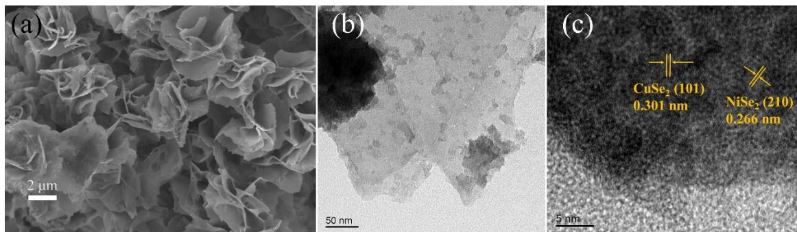
**Fig. S14.** a) SEM, b) TEM, and c) HRTEM images of  $\text{NiSe}_2@\text{CuSe}_2$  after test.
