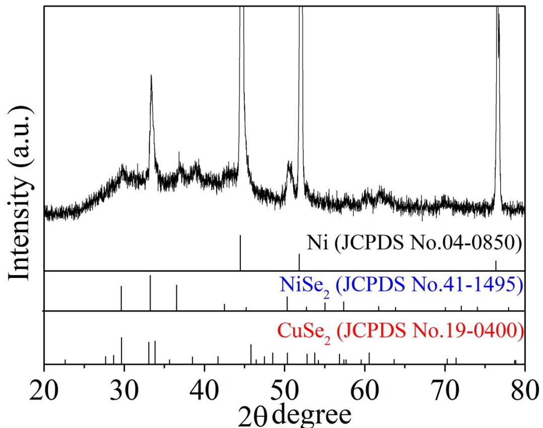
**Fig. S13.** XRD pattern of  $\text{NiSe}_2@\text{CuSe}_2/\text{NF}$  after test.
