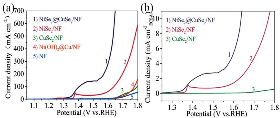
**Fig. S11.** a) LSV curves of  $\text{NiSe}_2@\text{CuSe}_2/\text{NF}$ ,  $\text{NiSe}_2/\text{NF}$ ,  $\text{CuSe}_2/\text{NF}$ ,  $\text{Ni(OH)}_2@\text{Cu/NF}$  and NF after iR compensation. b) The OER performance of  $\text{NiSe}_2@\text{CuSe}_2/\text{NF}$ ,  $\text{NiSe}_2/\text{NF}$ , and  $\text{CuSe}_2/\text{NF}$  after the electrochemical surface area normalization.
