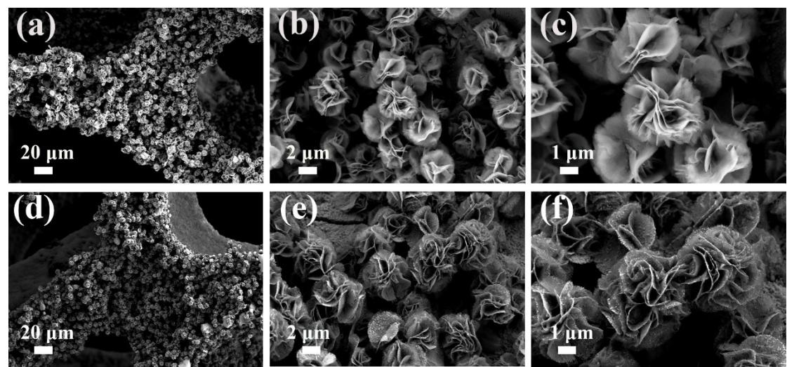
**Fig. S5.** SEM and magnified SEM images of a-c) Ni(OH)<sub>2</sub>@Cu/NF, d-f) NiSe<sub>2</sub>@CuSe<sub>2</sub>/NF.
