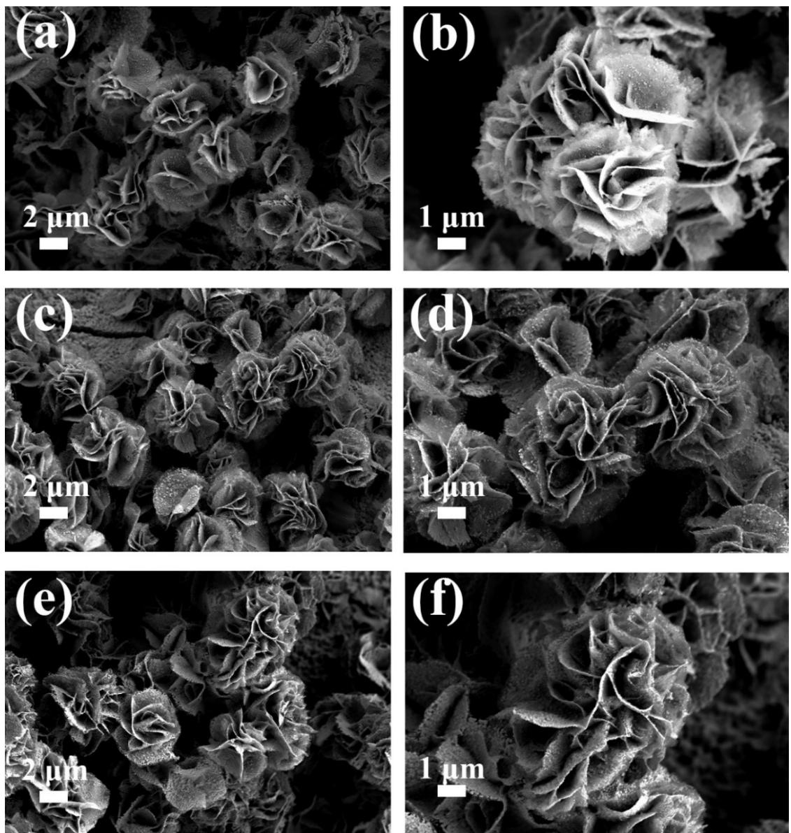
**Fig. S8.** SEM and magnified SEM images of NiSe<sub>2</sub>@CuSe<sub>2</sub>/NF with different hydrothermal time a-b) 3 h, c-d) 6 h e-f) 9 h.
