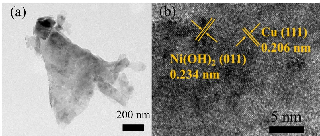
**Fig. S3.** a) TEM and b) HRTEM images of  $\text{Ni}(\text{OH})_2@\text{Cu}$ .
