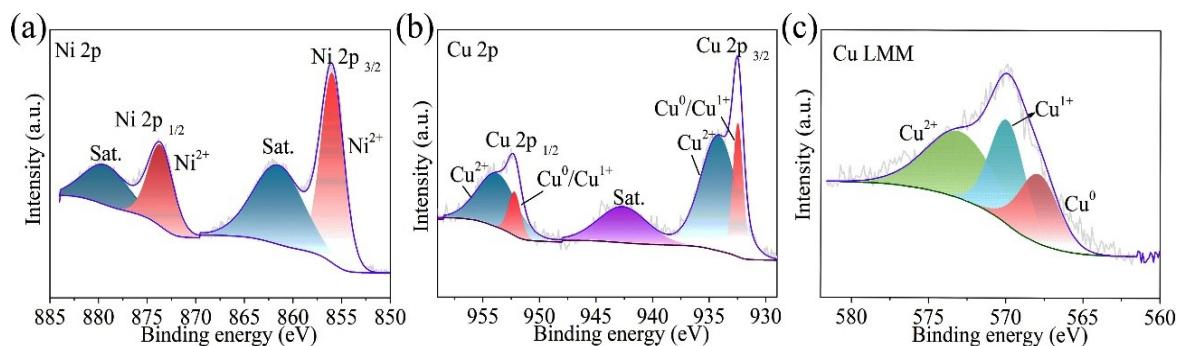
**Fig. S4.** The high-resolution XPS spectra of a) Ni 2p, b) Cu 2p, and c) Cu LMM for  $\text{Ni}(\text{OH})_2@\text{Cu}$ .
