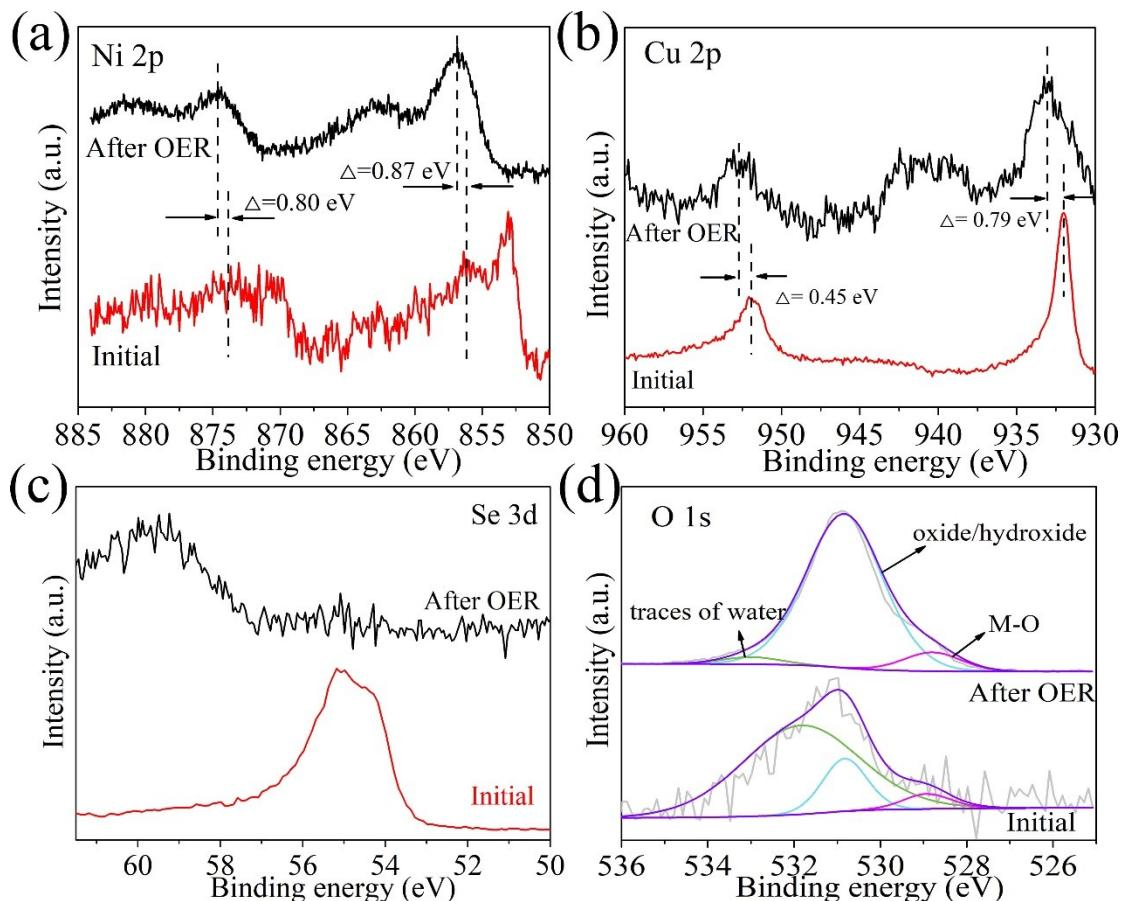
**Fig. S15.** The comparision of a) Ni 2p, b) Cu 2p spectrum, c) Se 3d spectrum and d) O 1s spectrum of  $\text{NiSe}_2@\text{CuSe}_2/\text{NF}$  before and after test.
