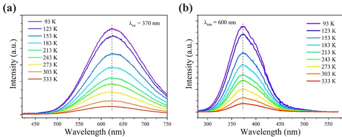
**Figure. S2** Temperature dependent (a) PL and (b) PLE spectra of the TZN-5-Laser sample.
