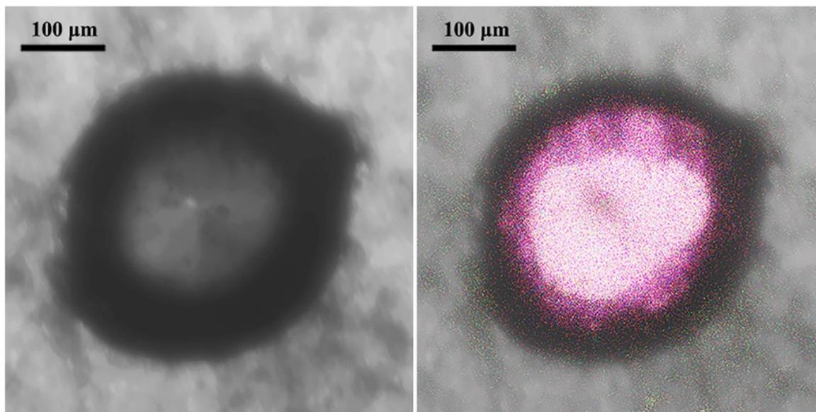
**Figure. S3** CLSM image of the surface of the laser spot in TZN-5-Laser sample. the photos are taken without (left) or with (right) 405 nm UV laser excitation.
