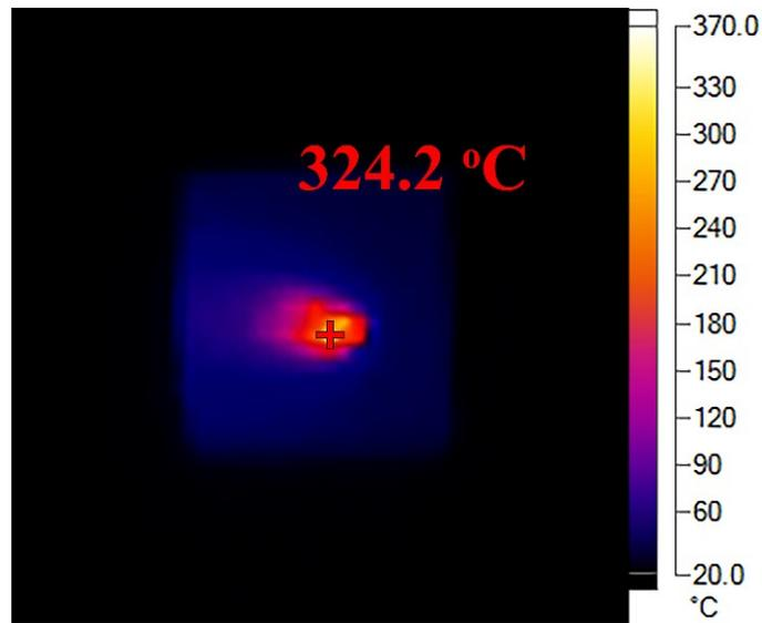
**Figure. S5** Thermal imaging photograph on the TZN-5 glass upon laser irradiation.
