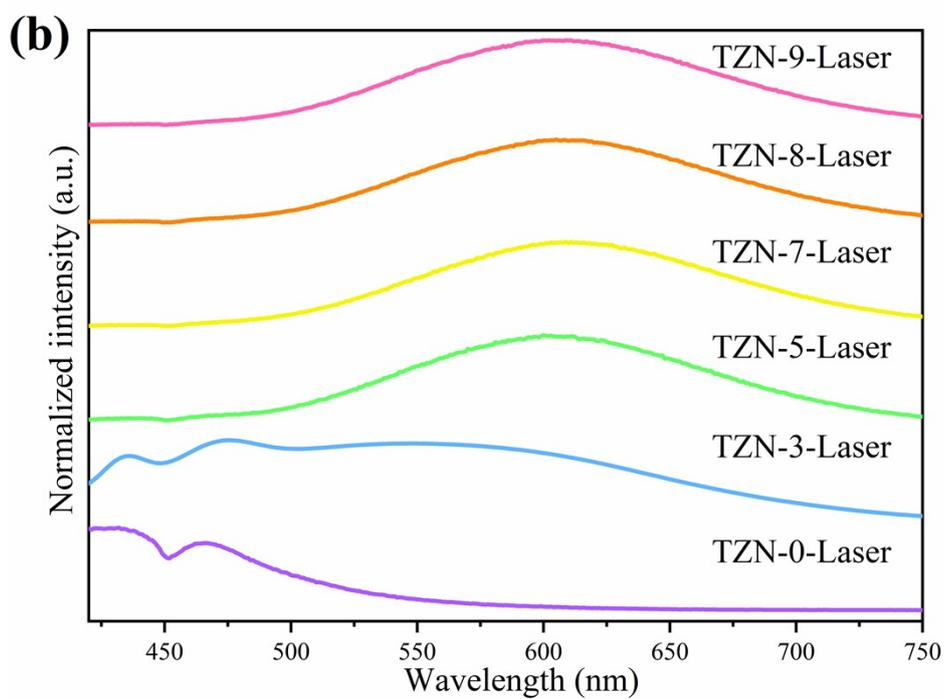
**Figure. S8** PL spectra of TZN-x glasses (a) before and (b) after laser irradiation.
