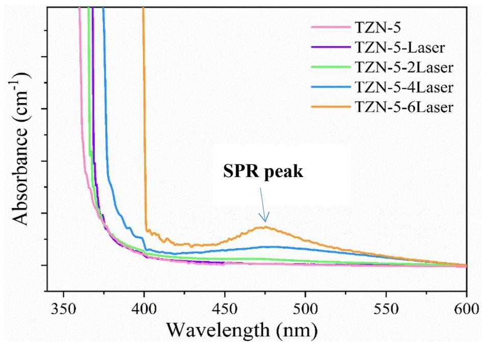
Figure. S7 The absorption spectra of the TZN-5 sample with laser irradiation for different number of shot times.
