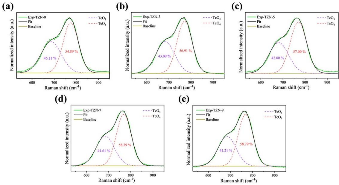
**Figure. S4** Raman spectra analyses on the B band and C band of the TZN-x glasses via Gaussian deconvolutions.
