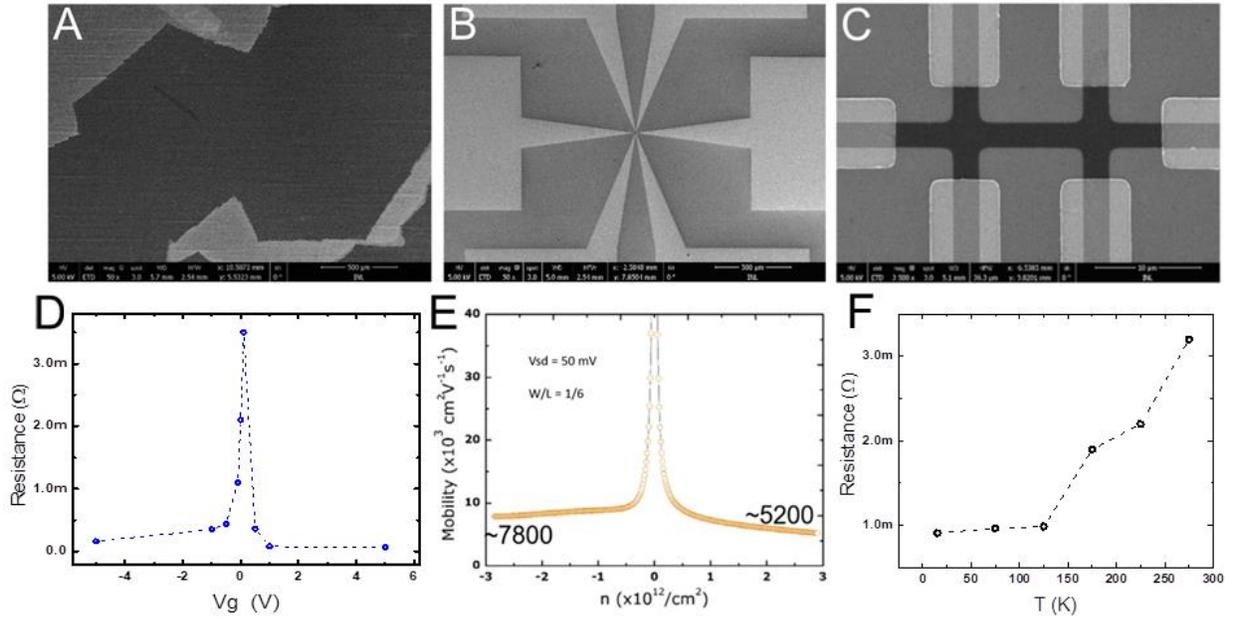
**Figure S1** – Quality of the graphene layer: a) SEM image of graphene obtained after CVD process on copper, b) Hall bar device designed for CVD graphene electrical characterization, c) zoom view of defined graphene sheet channel, d) resistivity as a function of gate voltage, e) CVD graphene carrier mobility and f) evolution of graphene resistance as a function of temperature.
