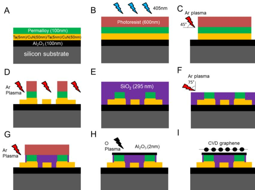
**Figure S2** – Fabrication process: a) Layers deposition, b) photoresist spinning and sensibilization, c) definition of each device area, d) pillars definition by milling e) oxide deposition by CVD, f) planarization, g) electrical contacts definition, h) tunnel barrier deposition and i) graphene transference.
