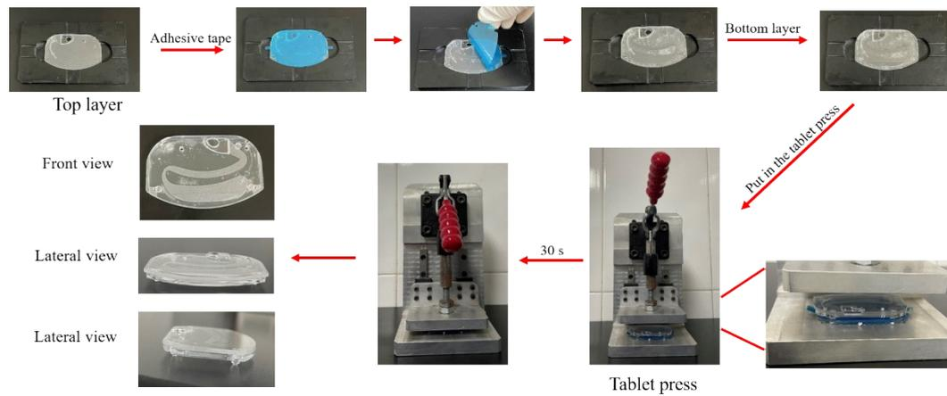
**Fig. S2** The detailed procedure of tablet pressing.
