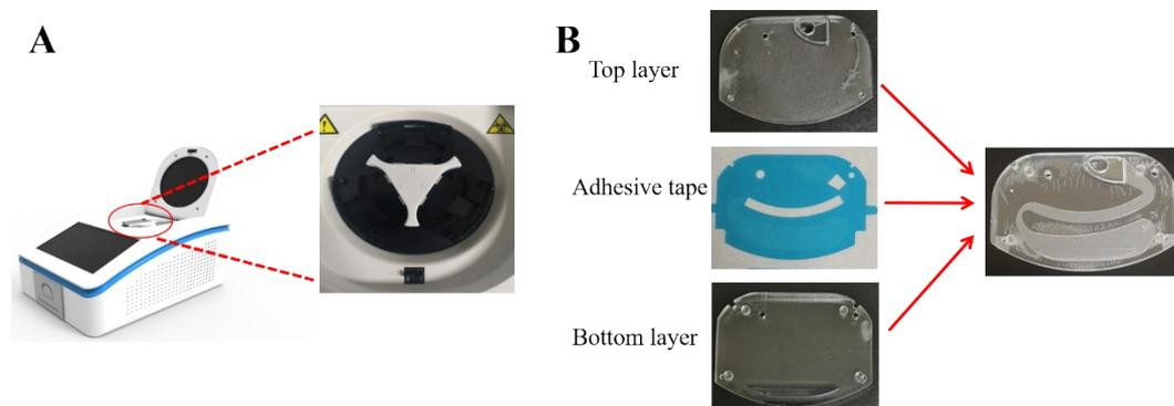
**Fig. S1** The configuration of the platform. (A) The constitution of the fluorescence detection analyzer. (B) The structure of the microfluidic chip for immune analysis.
