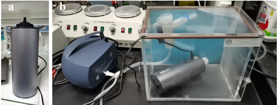
Fig. S6. (a) The suction pump with the membrane adaptor; (b) The picture of the viral sampling process.
