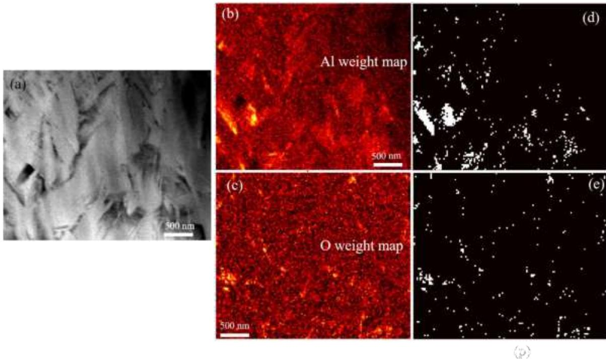
Figure S2: (a) HAADF STEM image of MoAlB (part of the area as shown in S1). (b)-(c) EDX weight mappings processed by multivariate statistical analysis [S1] for the Al-rich (b) and O-rich phases (c). Areas of Al-rich (d) and O-rich (e) phases are highlighted in white. The area fractions of the Al-rich and O-rich phases are 4.5% and 2%, respectively.
