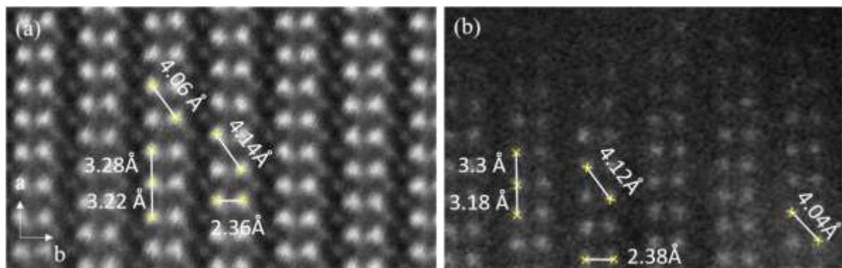
Figure S6: Gauss peak fitting were carried out for (a) MoAlB and (b) MoB region. Yellow crosses mark the center of mass of Mo atoms shown as example. Representative Mo-Mo distance measurements are marked by white lines
