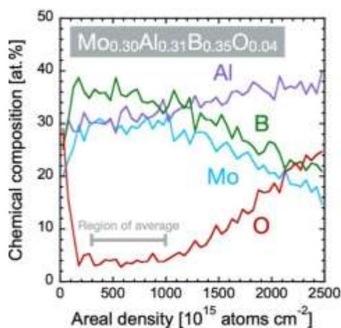
Figure S3: Chemical composition depth profile as obtained from ToF-ERDA. The region used to obtain the average composition of the MAB phase is indicated in grey.
