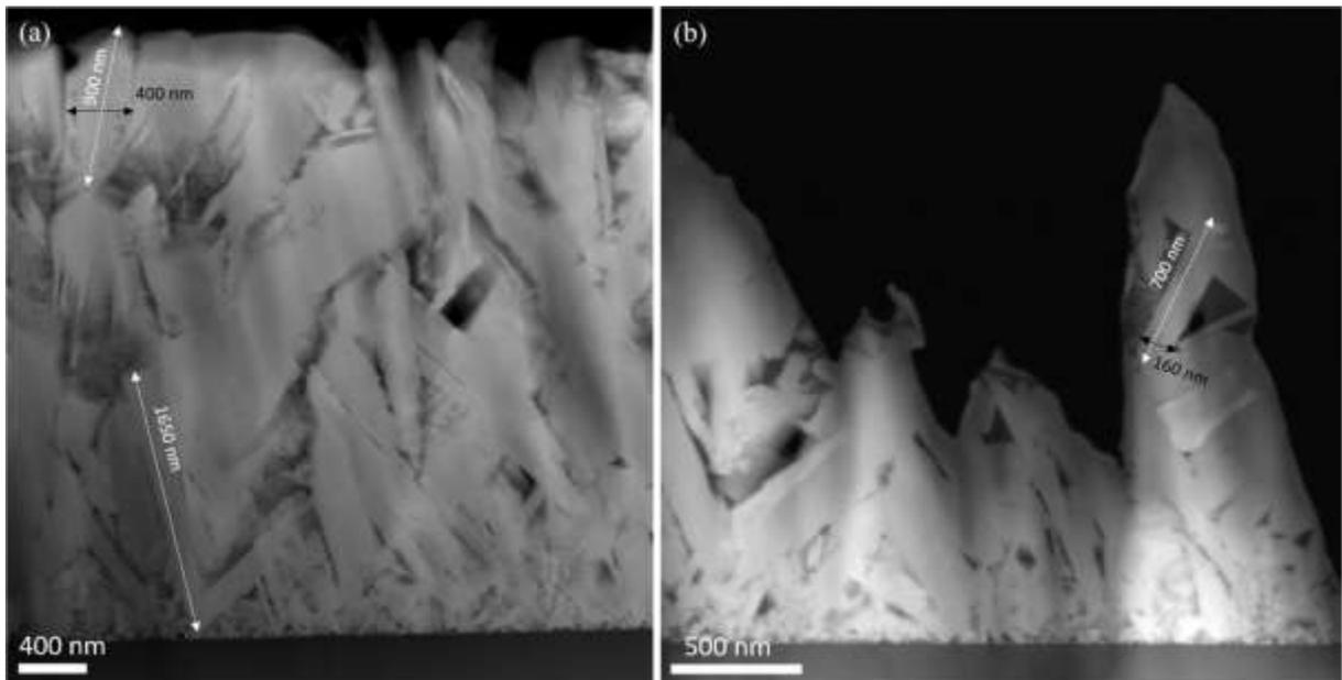
Figure S5: Low magnification HAADF STEM shows an average statistical analysis of MoAlB domain measuring the grain size in (a). The MoAlB grain in (b) is the area of interest described in the manuscript.
