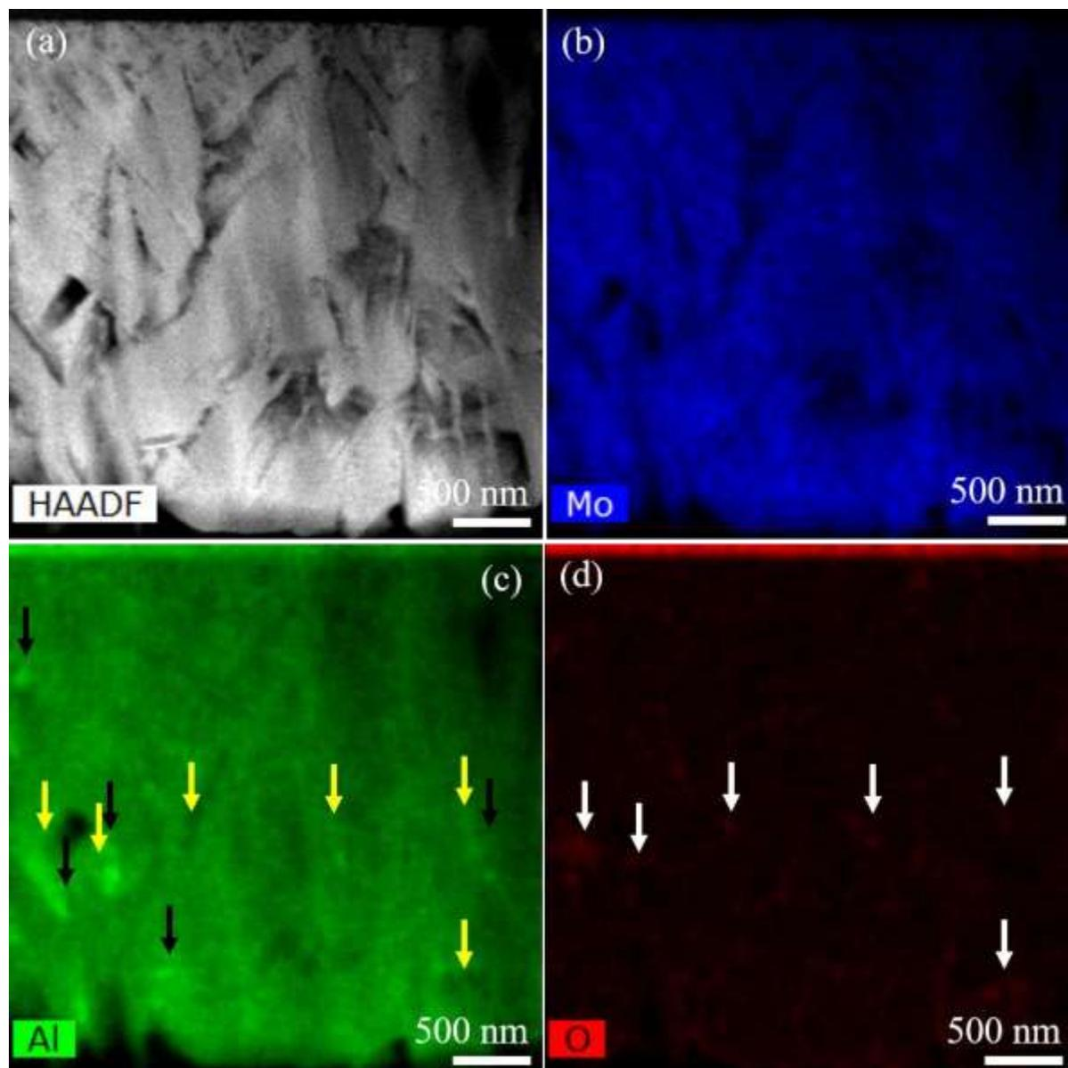
Figure S1: (a)-(d) Large-scale STEM EDX showing chemical composition mapping of Mo, Al and O. Al-rich and O-rich phases are marked by black and white arrows in (c) and (d) respectively. Representative areas of AlO<sub>x</sub> are marked by yellow arrows in (c).
