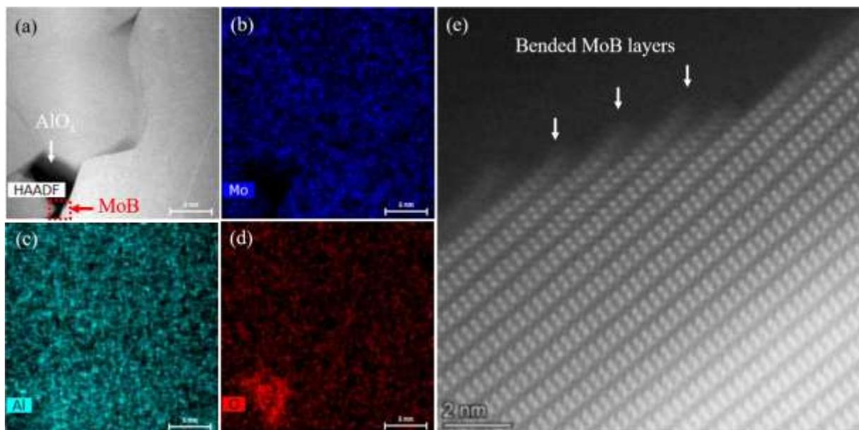
Figure S7: (a) HAADF STEM image where  $\text{AlO}_x$  region (white arrow) and 2D MoB MBene area (red dotted rectangle) are marked. (b)-(d) are STEM EDS showing chemical mapping of the same area as in (a). (e) HR-STEM image depicting bent MoB layers marked with white arrows.
