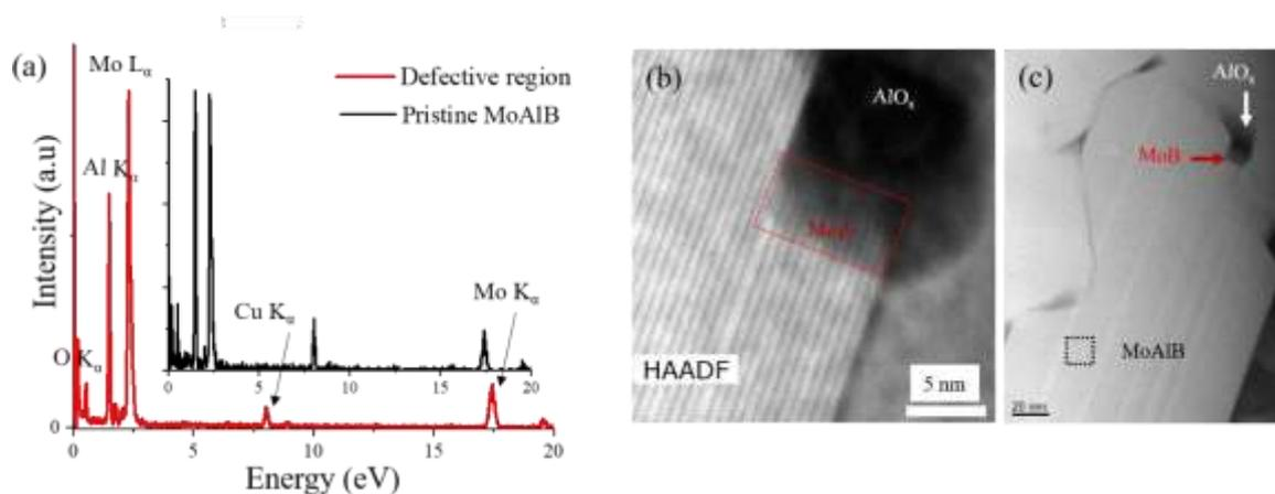
Figure S4: (a) Comparison of EDS spectra and Mo and Al intensities in MoAlB and MoB region. HAADF images (b) and (c) where the areas of spectra acquisition for MoB (red rectangle) and MoAlB (black rectangle) are marked.
