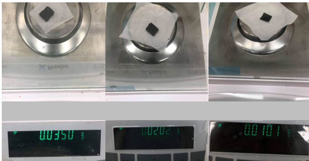
Figure S3. Digital photographs showing their representative mass loading (35, 20, and 10 \text{mgcm}^{-2} .) of the fabricated electrodes
