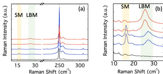
Figure S2. Room temperature ultra-low frequency Raman measurements using 532nm excitation and an Ondax SureBlock ultra narrow-band notch filter. (a) Spectra are acquired from 2H (blue), 3R (red) and monolayer (black). Spectra are offset for clarity. (b) Both shear (SM) and layer-breathing modes (LBM) are evident in 2H bilayers. 3R stacking exhibits only a LBM mode. Monolayer WSe<sub>2</sub> exhibits neither SM or LBM.
