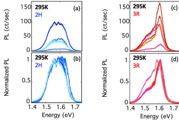
Figure S3. Room temperature photoluminescence from (a) five additional 2H samples and (c) five additional 3R samples. In both stacking orders the overall intensity varies significantly. (b,d) The normalized PL shows a consistent line shape for each stacking order, despite the intensity variations. 532nm excitation and identical parameters are used to probe all samples.
