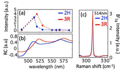
Figure S5. (a) Low-temperature (4K) excitation-dependent Raman intensity of the  $B_{2g}^1$  mode and (b) reflectance contrast, RC, plotted as a function of wavelength. The RC is the same data presented in Fig 5b of the main text, replotted here for clarity. (c) The  $B_{2g}^1$  mode of 2H (blue) and 3R (red)  $WSe_2$  is nearly indistinguishable for 514 nm excitation.
