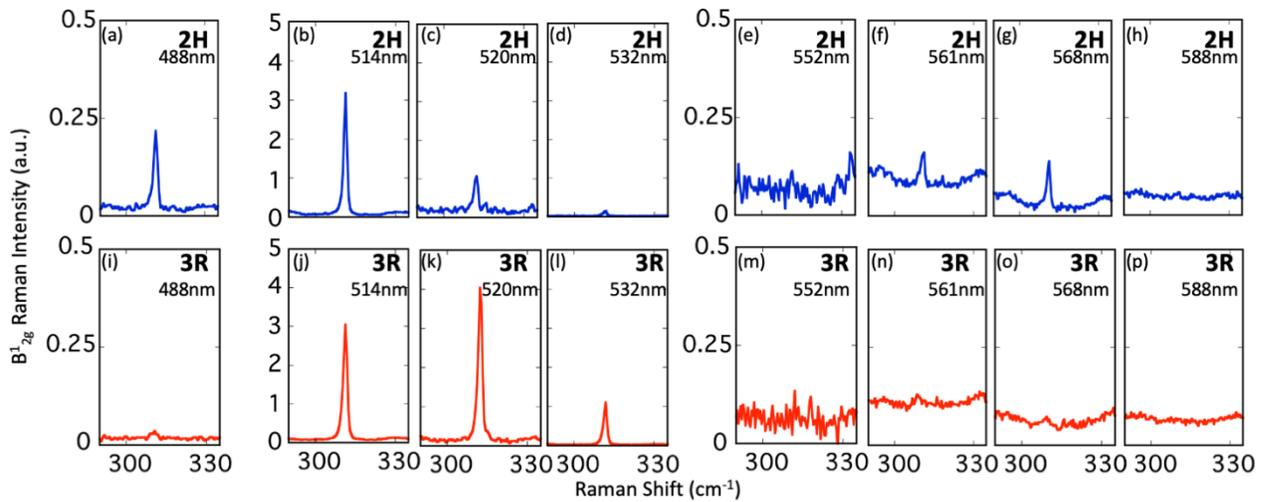
Figure S4. Low-temperature (4K) excitation-dependent Raman of the  $B_{2g}^1$  Raman mode in  $WSe_2$  bilayers for (a-h) 2H and (i-p) 3R stacking orientation. All spectra are normalized to Si Raman intensity at  $523\text{ cm}^{-1}$  and excitation wavelength is indicated in the upper right corner.
