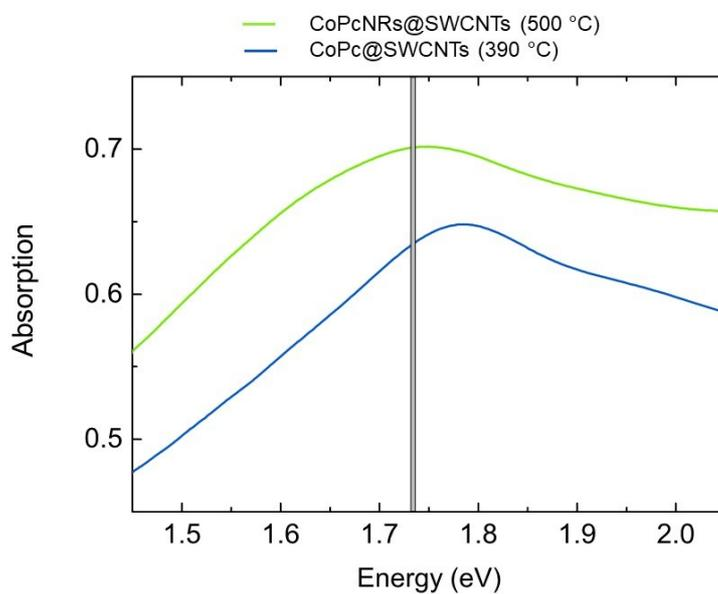
**Figure S2.** Absorption spectra of pristine SWCNTs and nanotubes after the filling protocols and polymerization step at lower (390 °C) and higher temperature (500 °C). Not fully polymerized NRs (blue color) and CoPcNRs inside SWCNTs as in the main text (green color).
