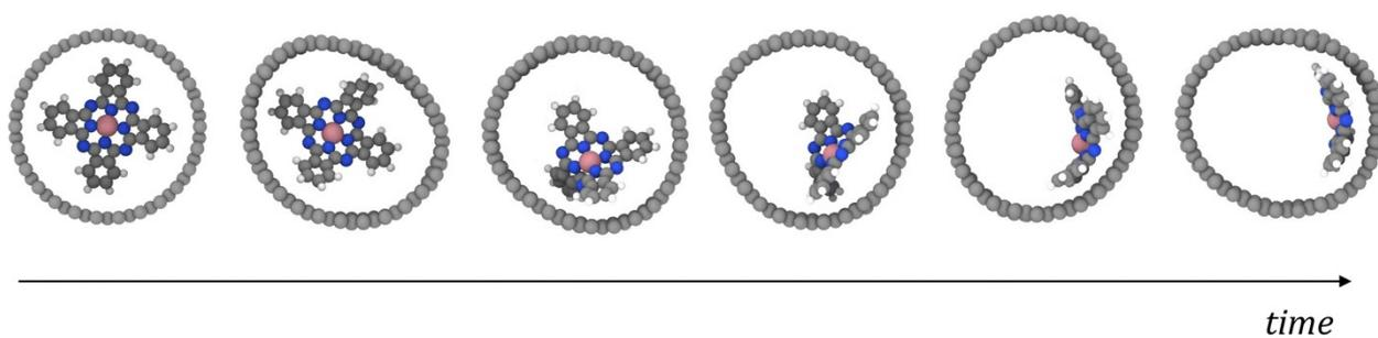
**Figure S6.** Snapshots of molecule motion during time inside the nanotube. The CoPc molecules tend to stick to the inner surface and bend. The behavior might depend on SWCNT diameter.
