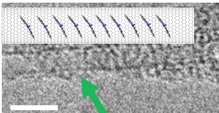
**Figure S5.** HR TEM images of CoPc molecules in SWCNTs (area marked with the green arrow indicates a section of about 10 stacked CoPc molecules). Elongated twisted structures characteristic for CoPcNR are not observed in this material. The scale bar is 2 nm.
