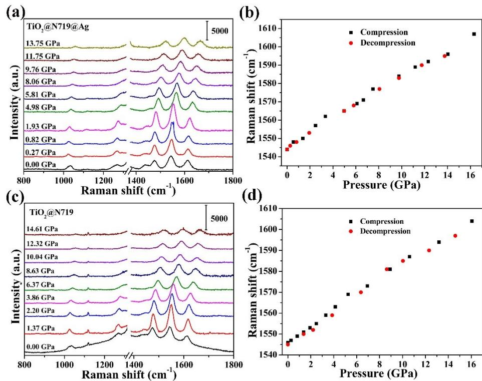
Figure S5. High pressure SERS spectra of (a)  $\text{TiO}_2@\text{N719}@\text{Ag}$  system and (c)  $\text{TiO}_2@\text{N719}$  measured during decompression experiment. Plots of frequencies of the band at  $1544 \text{ cm}^{-1}$  versus the pressure upon compression and decompression of (b)  $\text{TiO}_2@\text{N719}@\text{Ag}$  system and (d)  $\text{TiO}_2@\text{N719}$ .
