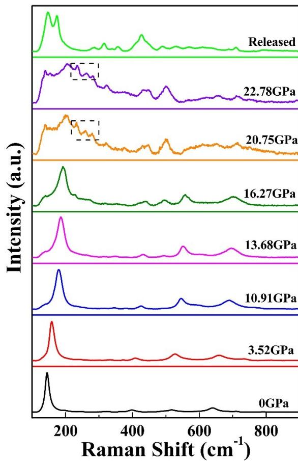
Figure S4. Raman spectra of  $\text{TiO}_2$  NPs obtained under high pressure.
