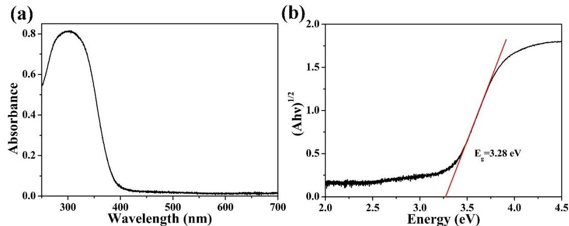
Figure S3. (a) UV-Vis absorption spectra of  $\text{TiO}_2$  NPs. (b) Relationship between  $(Ahv)^{1/2}$  and photon energy ( $hv$ ) for  $\text{TiO}_2$  NPs.
