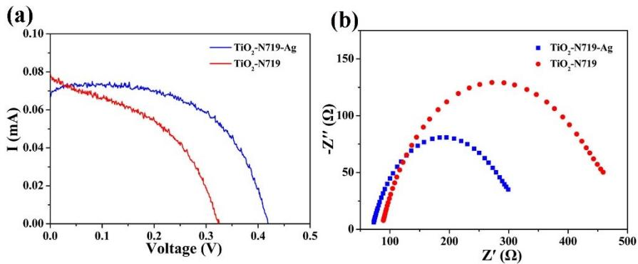
Figure S2. The photocurrent-voltage (I-V) curves (a) and impedance spectra (b) for the  $\text{TiO}_2\text{@N719}$  and  $\text{TiO}_2\text{@N719@Ag}$  systems.
