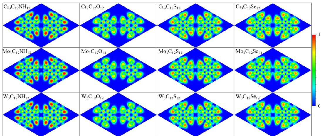
**Figure S3.** Illustrations of electron localization functions for unit cell  $M_3C_{12}X_{12}$ .
