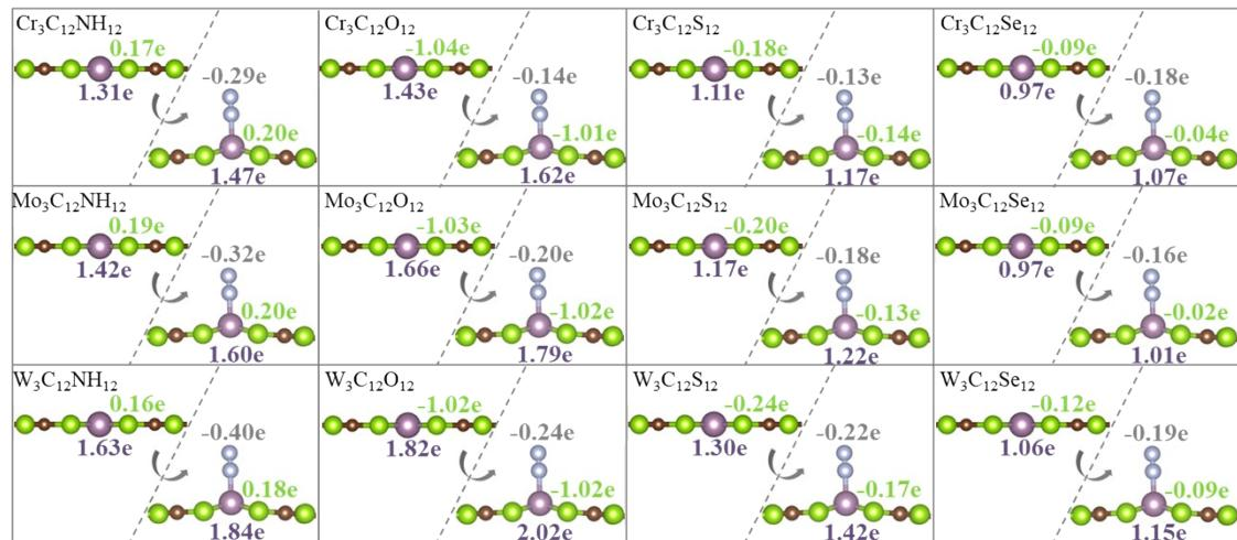
**Figure S2.** Schematic diagram of Bader charge distribution before and after  $N_2$  adsorption on  $M_3C_{12}X_{12}$ .
