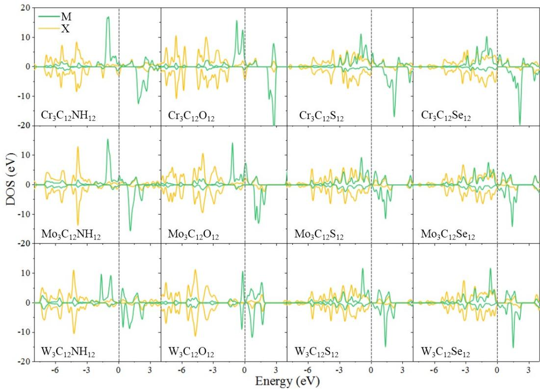
**Figure S1.** Spin-polarized partial density of states of M-d orbitals and X-p orbitals for  $M_3C_{12}X_{12}$ . The Fermi level is set to zero.
