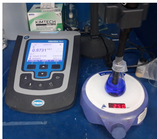
Figure S6. Ion-selective electrode (ISE) method of measuring ammonia contents. Photograph showing the one of a method which was used to measure the ammonia production rate.
