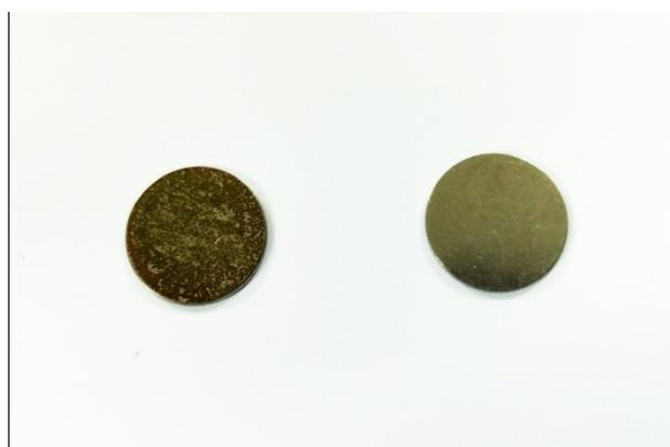
**Fig. S12.** The optical photographs of the gasket in assembled zinc ion battery without NMO electrode (Left image is after cycling and the right is initial state).
