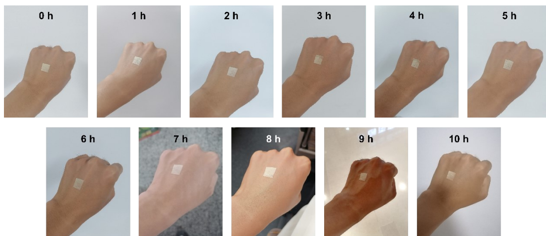
Figure S3. The ITO/PU micromesh attached on the hand of tester for 10 h. After peeling off the micromesh, the skin has no adverse feeling.
