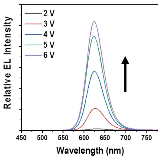
**Figure S14.** Electroluminescence spectra of InP QD-based LEDs at different operating voltages.
