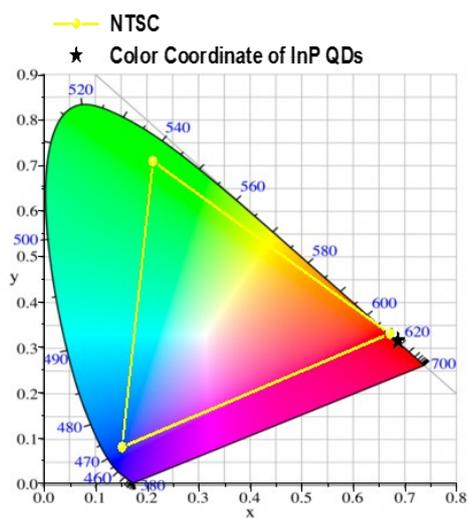
**Figure S12.** CIE 1931 chromatic coordinates of  $\text{InP}$  QDs at a certain applied voltage for an  $\text{ITO}/\text{PEDOT}:\text{PSS}/\text{PTAA}/\text{InP}$  QDs/ $\text{ZnO}$  NPs/ $\text{Al}$  device structure.
