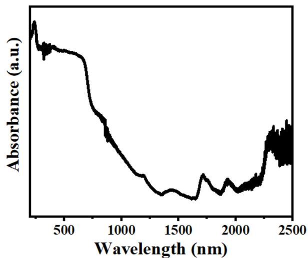
**Fig. S12** The absorption spectrum of the PLD-derived Te nanofilm.
