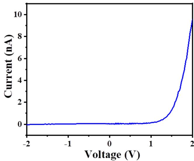
**Fig. S6** Rectifying characteristic of a Te/Si heterojunction diode.
