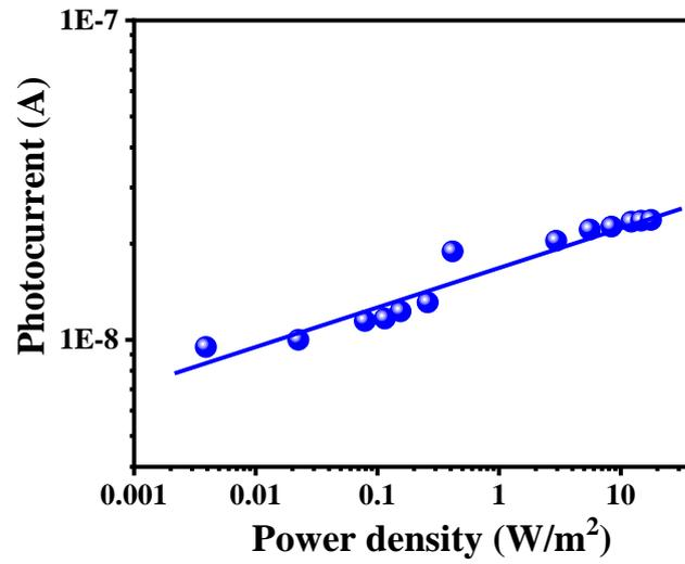
**Fig. S9** Photocurrent as a function of light power density of a Te/Si heterojunction photodetector under 405 nm illumination.
