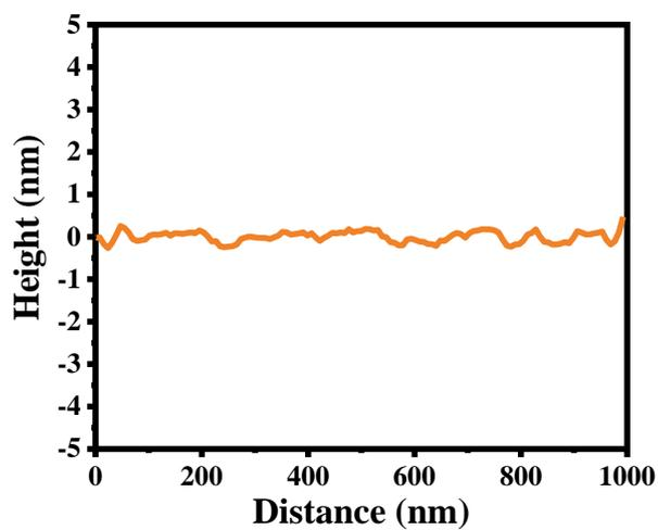
**Fig. S2** The AFM height profile along the surface of the PLD-derived Te nanofilm. The surface undulations are extracted to be below 1 nm.
