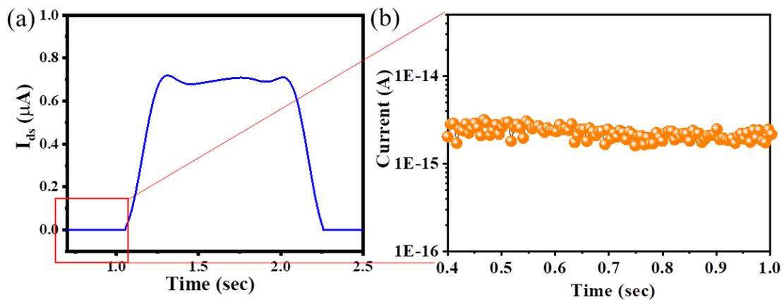
**Fig. S11** (a) A single photoswitching cycle of a Te/Si heterojunction photodetector acquired with a slow sampling working mode and (b) an enlarged view of the dark current.
