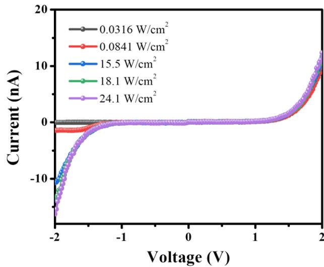
**Fig. S8** I-V curves of a Te/Si heterojunction photodetector under illumination with various light intensities.
