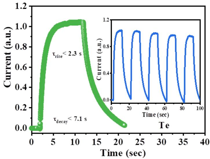
**Fig. S10** Photoswitching curve of a pure Te photodetector.
