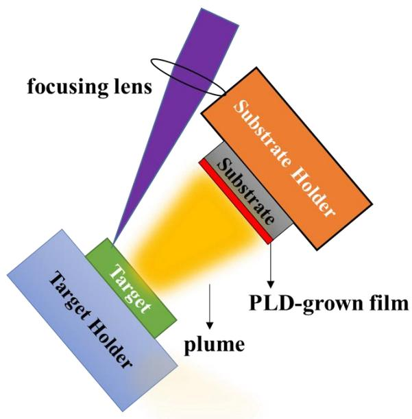
**Fig. S1** Schematic illustration of the PLD growth of Te nanofilms.
