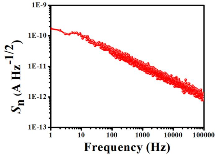
**Fig. S13** Current noise spectral density of a Te/Si heterojunction photodetector.
