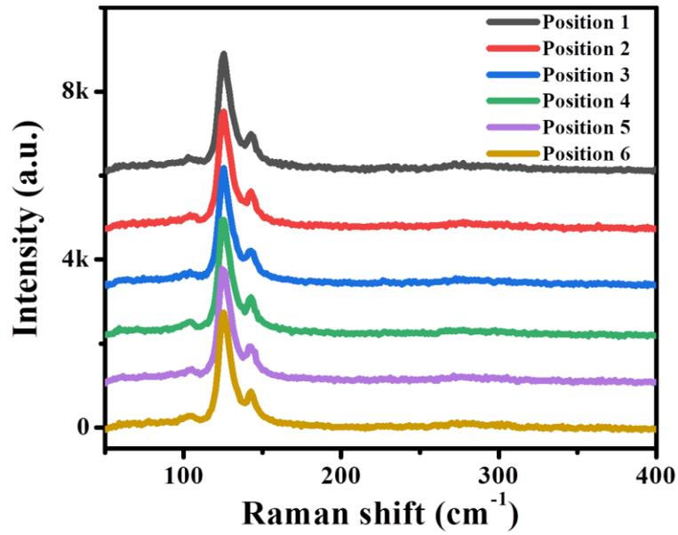
**Fig. S5** Raman spectra of random multiple points of a PLD-derived 2-inch Te nanofilm.
