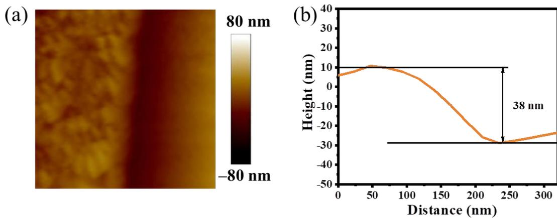
**Fig. S3** (a) AFM image of a Te/SiO<sub>2</sub> heterointerface and (b) the corresponding thickness profile across the heterointerface.
