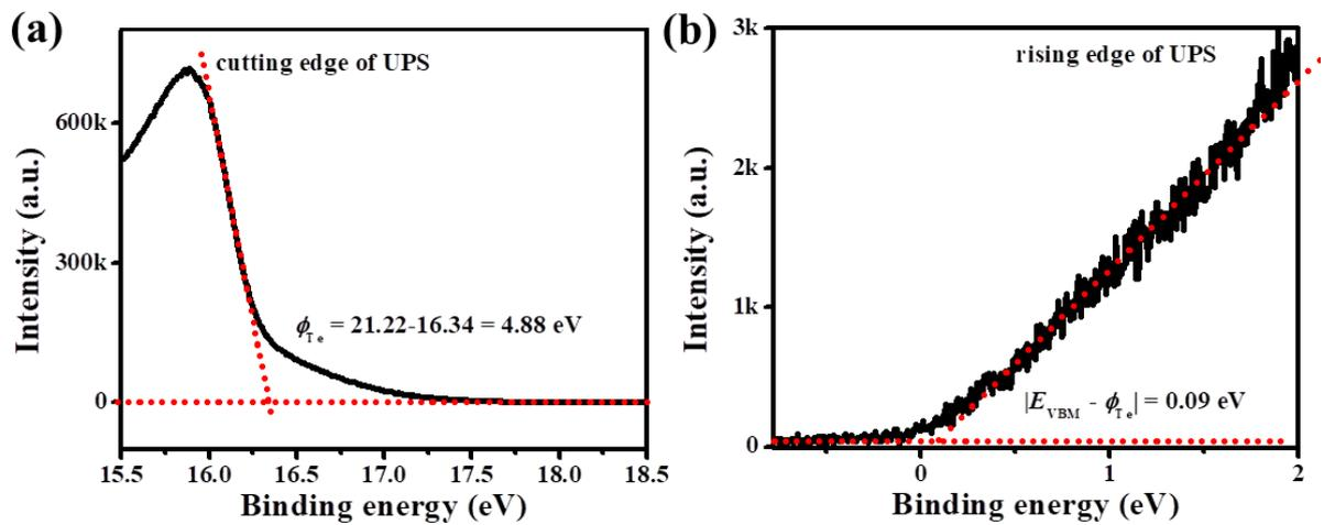
**Fig. S16** (a) The cutting edge and (b) rising edge of the UPS spectrum of the PLD-derived Te nanofilm.  $\phi_{Te}$  is the work function of Te.  $E_{VBM}$  is the energy level of the valence band maximum. The Fermi level is extracted to be 0.09 eV higher than the valence band maximum.
