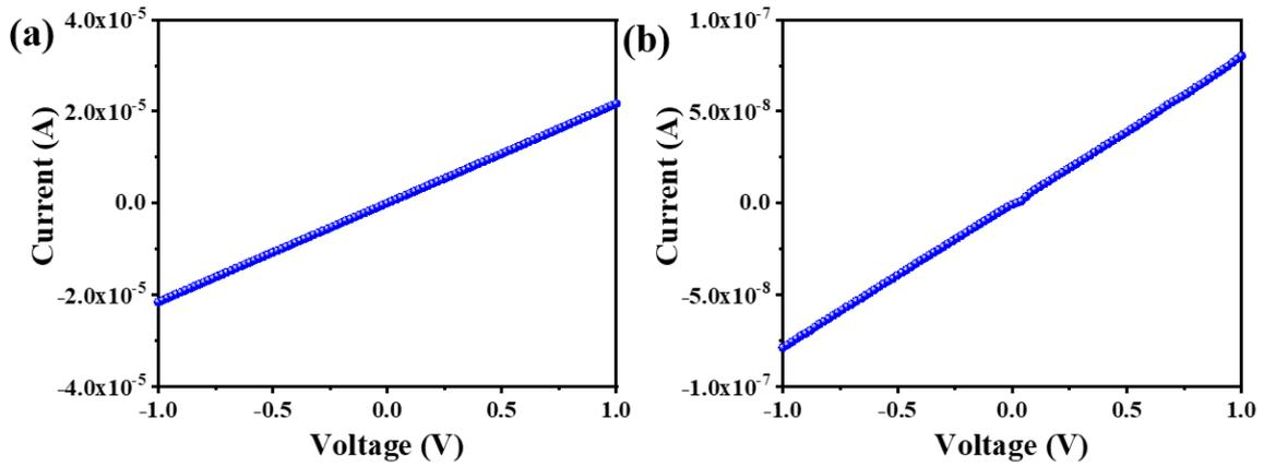
**Fig. S7** The I-V curves of (a) Ag-Si-Ag and (b) Ti/Au-Te-Ti/Au.
