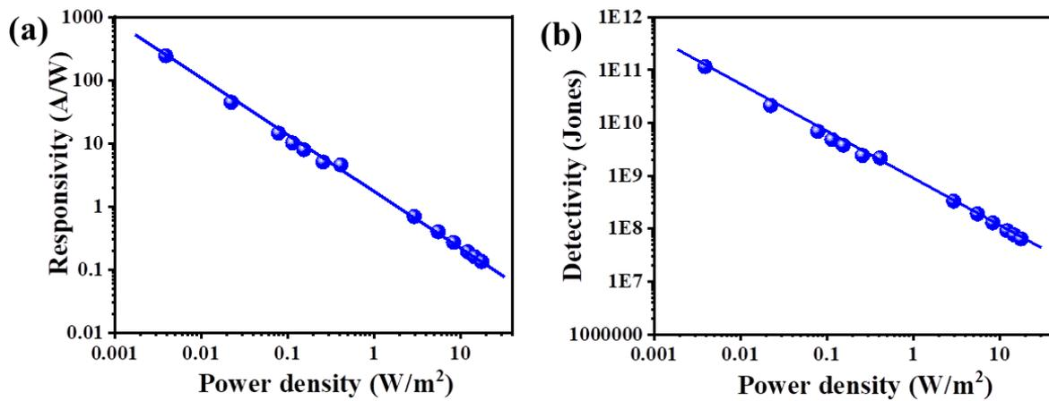
**Fig. S14** (a) Responsivity and (b) detectivity of a typical Te/Si heterojunction photodetector as a function of light power density under 405 nm illumination.
