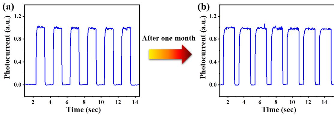
**Fig. S15** (a) The photoswitching curves of an as-fabricated Te/Si heterojunction photodetector and (b) that after a one-month storage in air.
