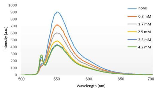
**Figure S6.** Emission Quenching of **4** by **1t**
