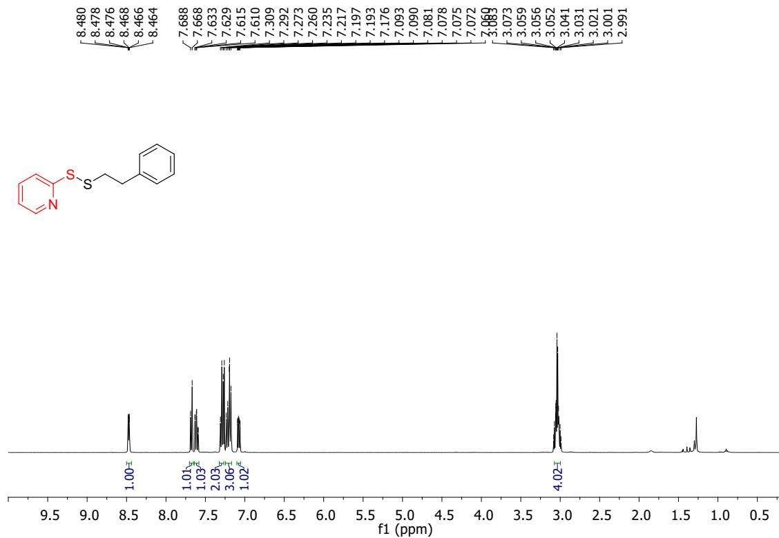
**Fig. S43.**  $^1\text{H}$  NMR spectrum of 2-(phenethyldisulfaneyl) pyridine (**2gl**)
