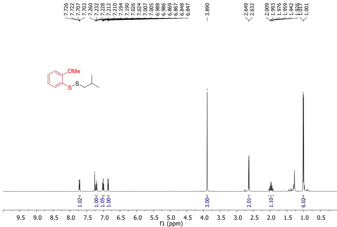
**Fig. S21.** <sup>1</sup>H NMR spectrum of 1-isobutyl-2-(2-methoxyphenyl)disulfane (**2cn**)
