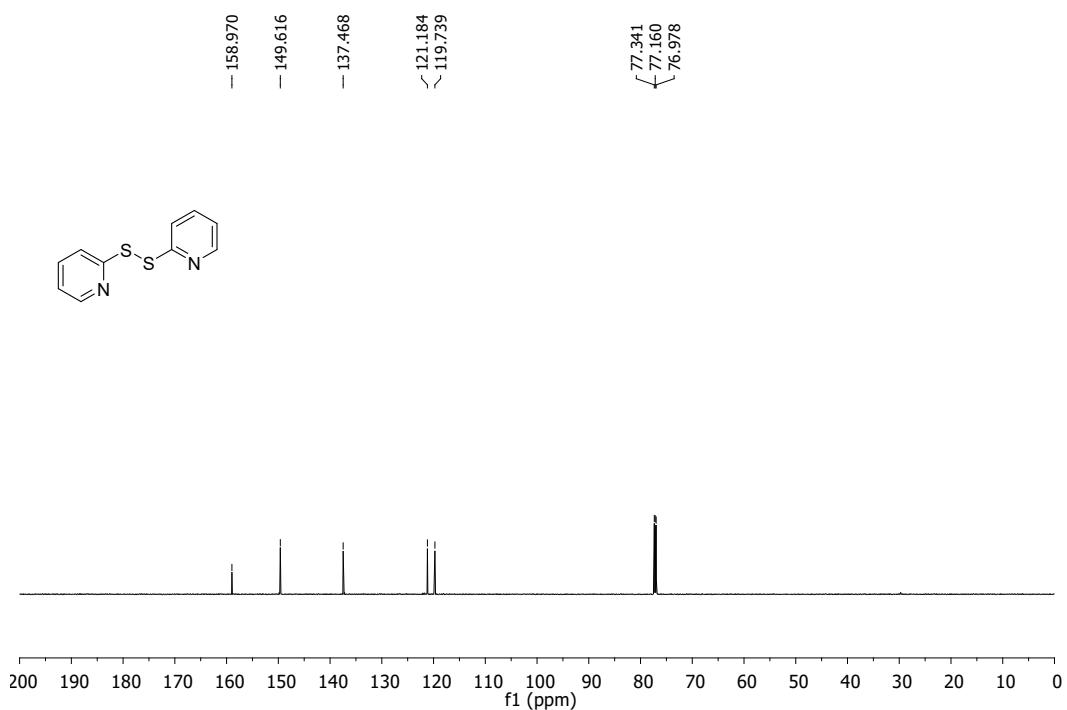
**Fig. S56.** <sup>13</sup>C NMR spectrum of 1,2-di(pyridin-2-yl)disulfane (**1g**).
