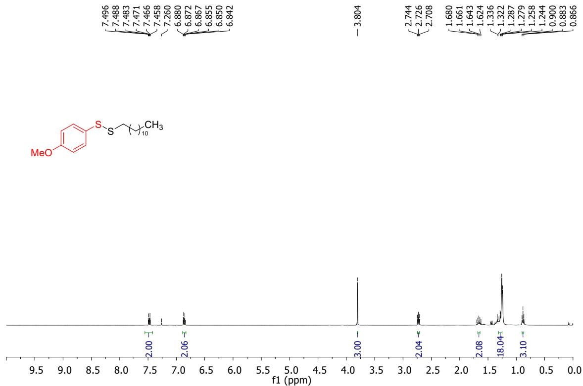
**Fig. S31.** <sup>1</sup>H NMR spectrum of 1-dodecyl-2-(4-methoxyphenyl)disulfane (**2eo**)
