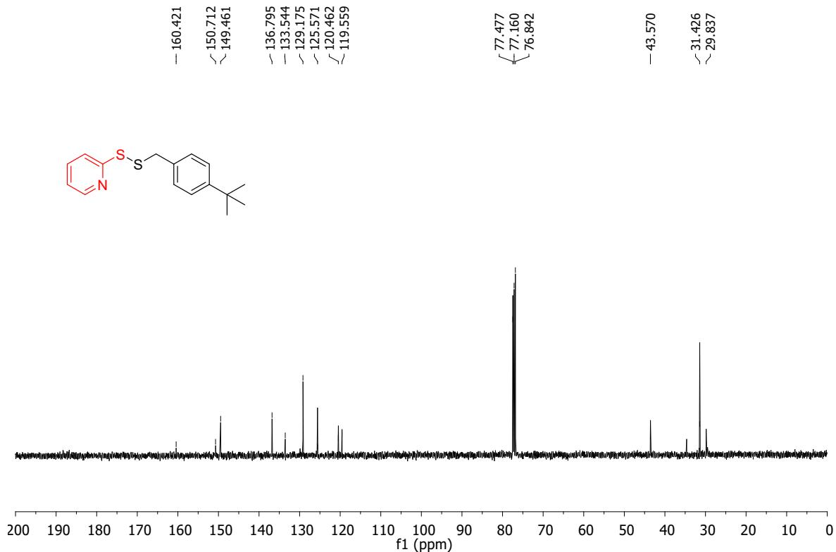
**Fig. S42.** <sup>13</sup>C NMR spectrum of 2-((4-(tert-butyl)benzyl)disulfaneyl)pyridine (**2gk**)
