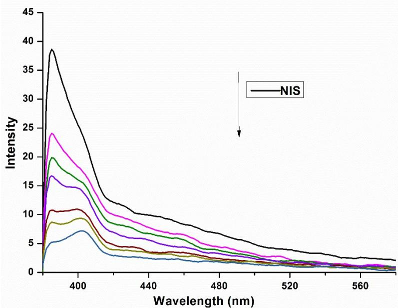
**Fig. S6.** Time-dependent Fluorescence spectrum of disulfide **1e** and NIS in MeCN (every 10 min intervals).
