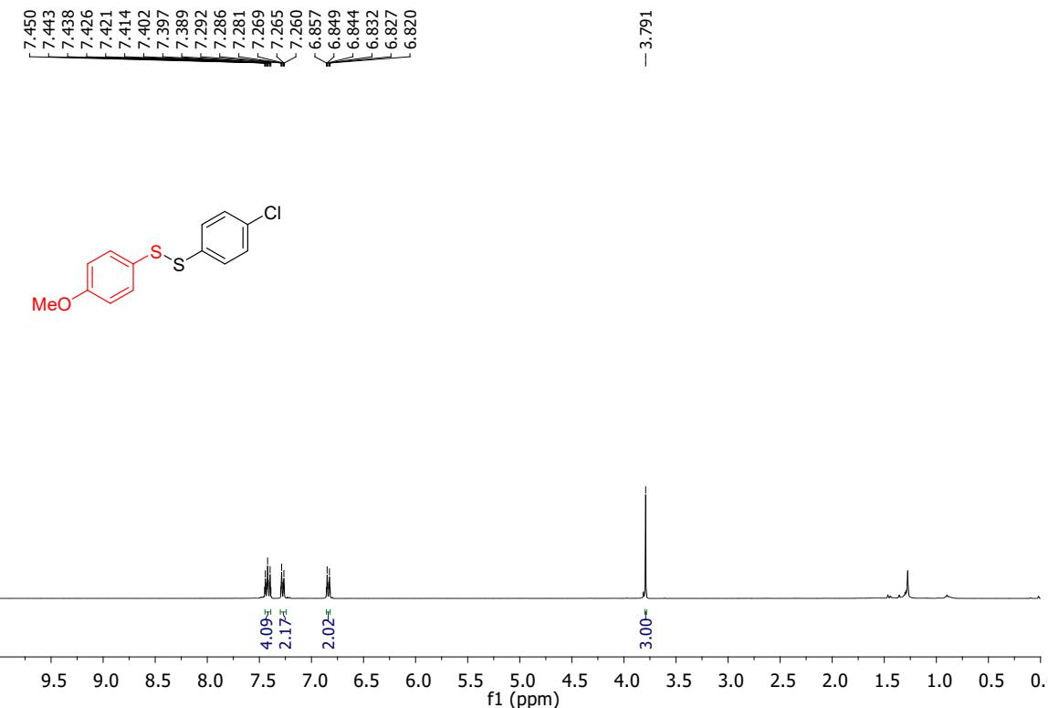
**Fig. S29.** <sup>1</sup>H NMR spectrum of 1-(4-chlorophenyl)-2-(4-methoxyphenyl)disulfane (**2ef**)
