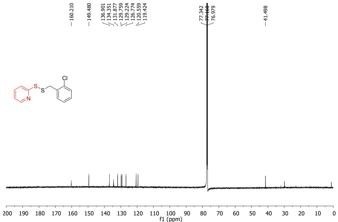
**Fig. S50.** <sup>13</sup>C NMR spectrum of 2-((2-chlorobenzyl)disulfaneyl)pyridine (2gp)
