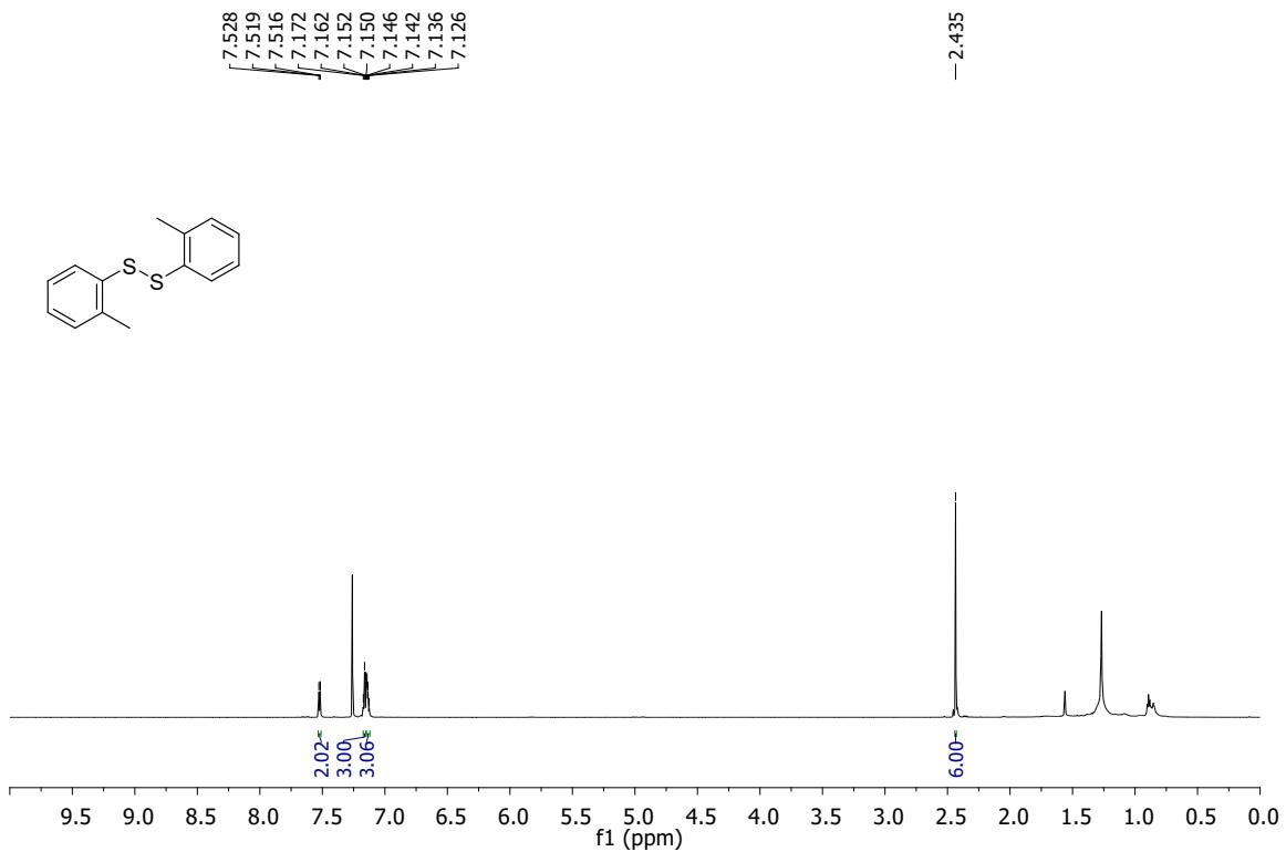
**Fig. S53.** <sup>1</sup>H NMR spectrum of 1,2-di-o-tolyldisulfane (**1a**)
