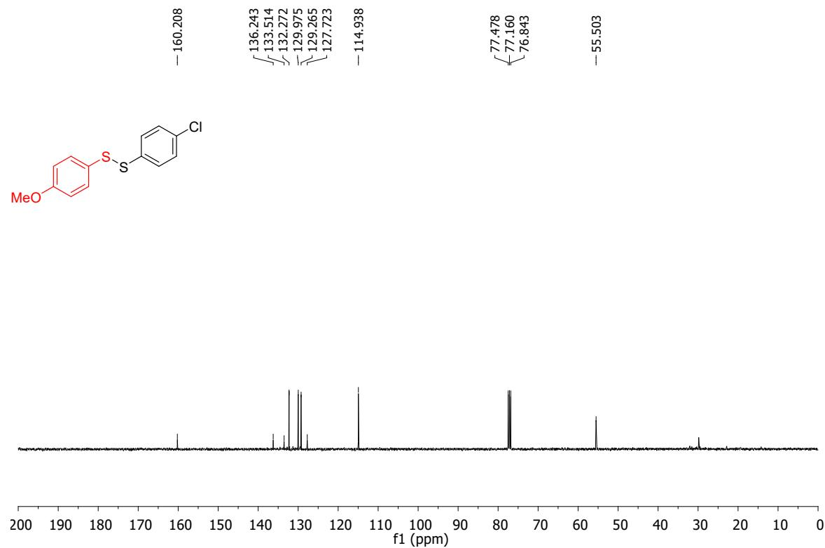
**Fig. S30.** <sup>13</sup>C NMR spectrum of 1-(4-chlorophenyl)-2-(4-methoxyphenyl)disulfane (**2ef**)
