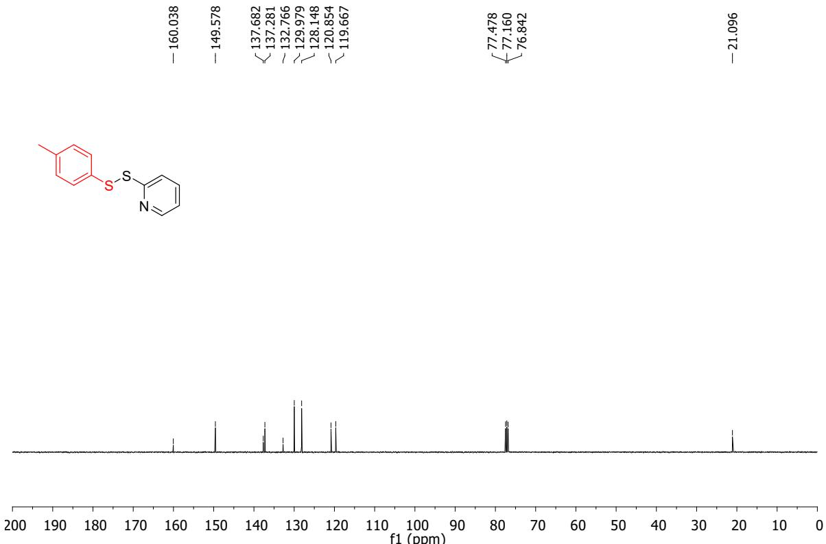
**Fig. S16.** <sup>13</sup>C NMR spectrum of 2-(p-tolyldisulfaneyl)pyridine (**2bg**)
