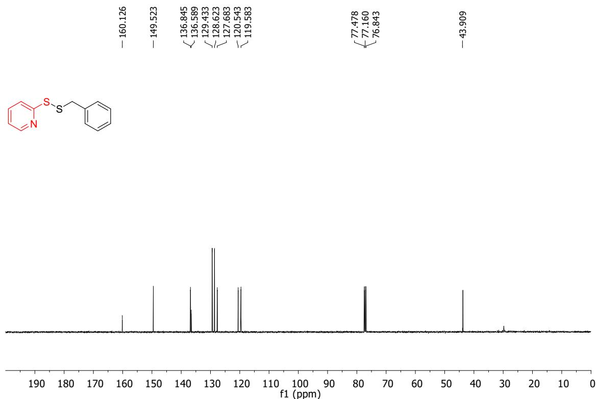
**Fig. S40.** <sup>13</sup>C NMR spectrum of 2-(benzyldisulfaneyl)pyridine (**2gj**)
