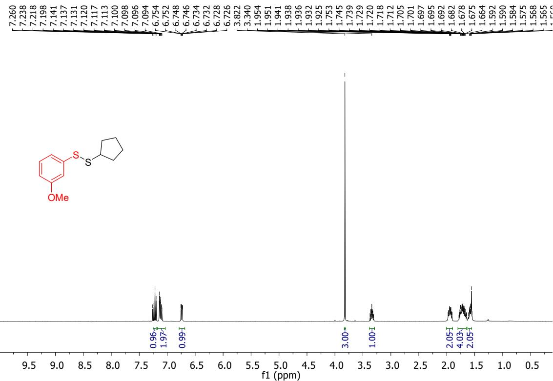
**Fig. S25.** <sup>1</sup>H NMR spectrum of 1-cyclopentyl-2-(3-methoxyphenyl)disulfane (**dh**)
