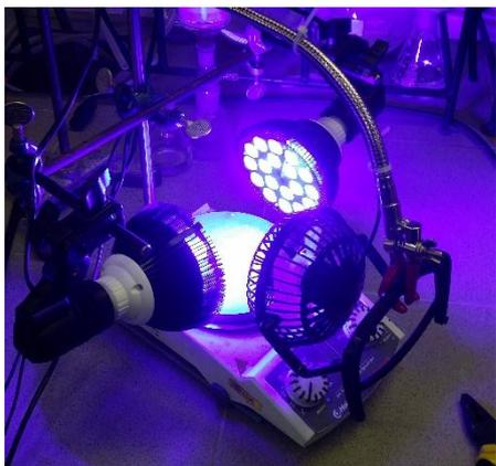
Figure 1. Photoredox reaction set-up.
