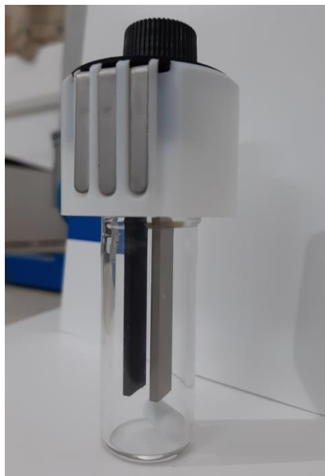
Fig. S2 10 ml reaction vessel with graphite & Pt electrodes
