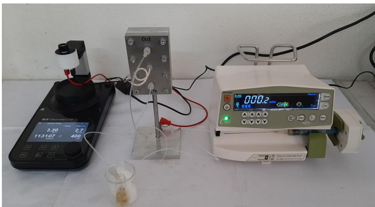
Fig. S3 IKA ElectraSyn 2.0 as power supply (left), \mu -EFR (middle), syringe pump (right).
