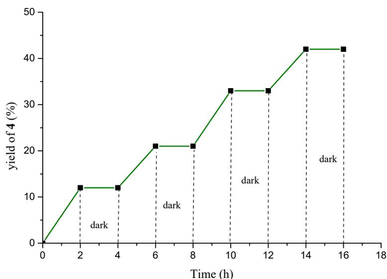
**Figure S4 Light on-off experiments. Yields were determined by  $^1\text{H}$  NMR spectroscopy with dibromomethane as an internal standard.**
