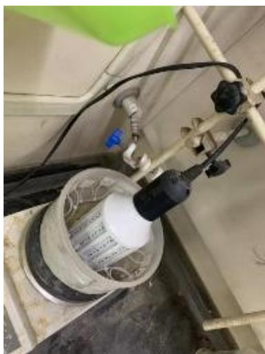
**Figure S1 Photograph of the Photocatalytic reactor used for reactions conducted under 450 nm LED irradiation.**
