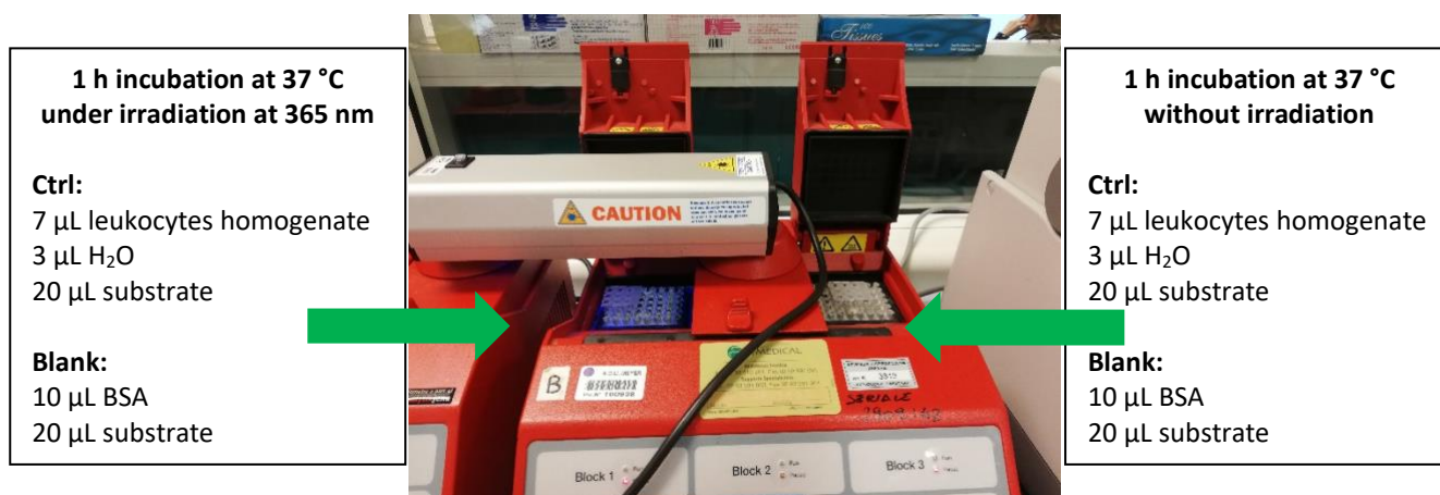
Figure S77: Novel set-up for the enzymatic activity assay under continuous irradiation at 365 nm (left) and without irradiation (right). During the experiment the left side was completely covered with foil to avoid visible light illumination.
