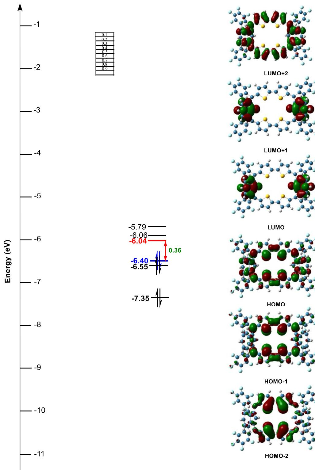
**Figure S27.** Selected frontier MOs of **6** calculated at B3LYP/6-31G (d, p) level of theory.
