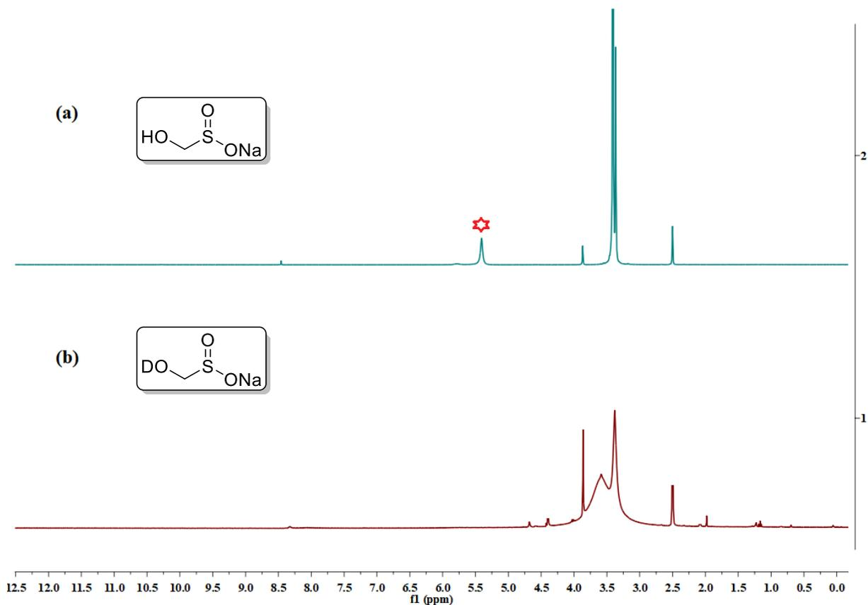
**Figure S2.**  $^1\text{H}$  NMR spectra of (a) Rongalite; (b) Deuterated rongalite.
