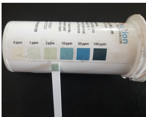
Figure S12: \text{H}_2\text{O}_2 detection using hydrogen peroxide strips
